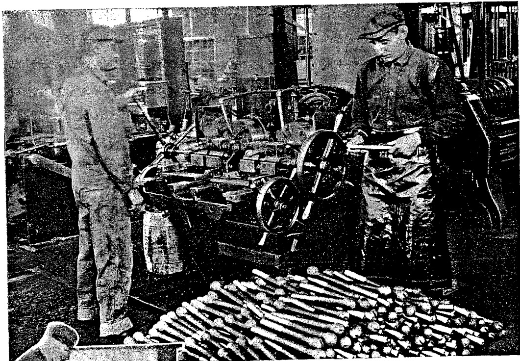
(Above)—Machine set up for threading flexible staybolts
