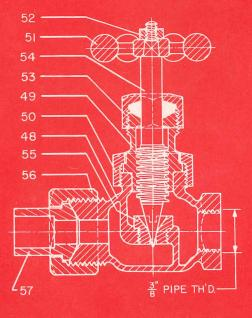
The Test Valve is used to check the operation of the Low Water Alarm. When the valve is opened, the chilled water in the expansion tube is blown out and replaced by hotter water from the boiler. The resulting increase in temperature causes the expansion tube to expand and the alarm to function.
