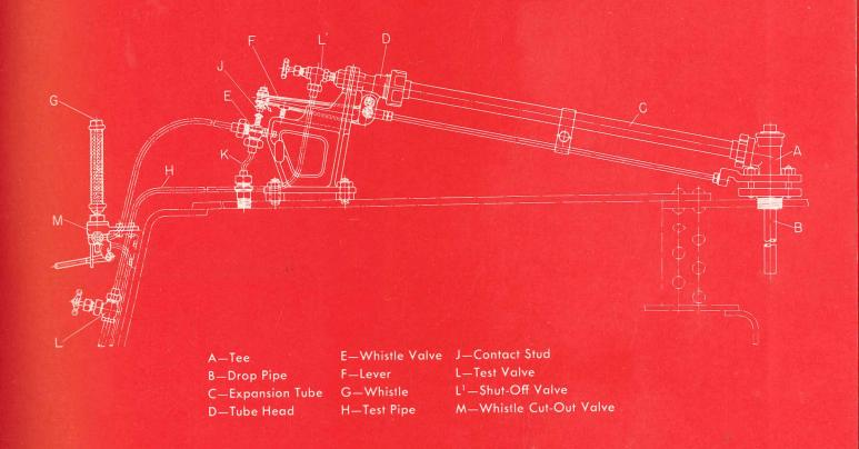
The Type B Alarmis furnished with its whistle mounted inside the cab. The Whistle Cut-Out Valve, Type 3241, illustrated on page 5, reduces the sound of the whistle while blowing down an engine.
