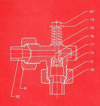
The opening of this valve sounds the whistle. It is operated by movement of the expansion tube transmitted through the lever pivoted on the tube head. As soon as the normal water level in the boiler has been restored, the valve closes.
