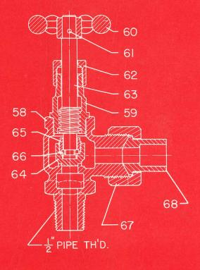
This valve is mounted between the Test Valve and the expansion tube. It should be kept open at all times and closed only when regrinding or otherwise repairing the Test Valve with boiler under steam.
