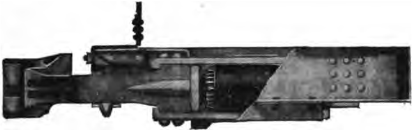
Westinghouse Friction Draft Gear as applied to Freight Cars of Pressed Steel Type
