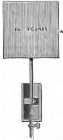
Fig. 24. Weight Raised by Pressure of Steam below Piston. Scale 8 in.—1 ft.
