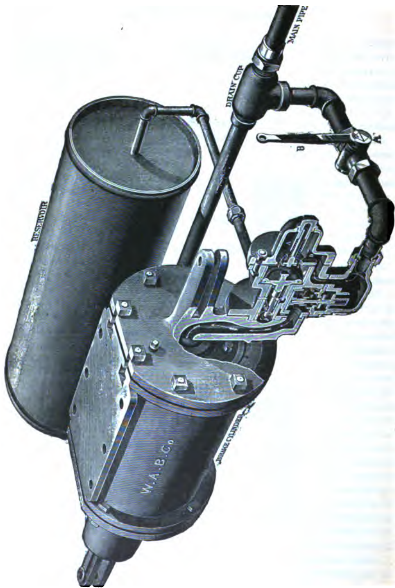
Fig. 464. Brake-Cylinder, Auxiliary Reservoir, and Triple-Valve.
