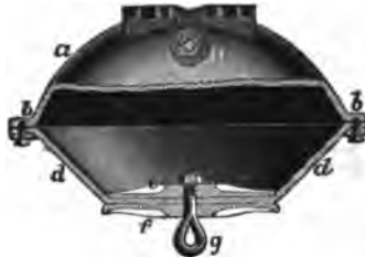
Fig. 463. Diaphragm Vessel for Vacuum-Brake.
