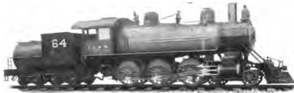
TEN-WHEEL LOCOMOTIVE With Vanderbilt Boiler and Tender
