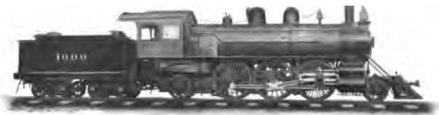
COMPOUND PRAIRIE TYPE LOCOMOTIVE For the Atchison, Topeka & Santa Fe Railway
