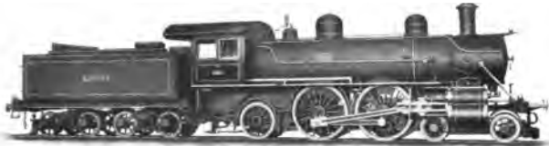
COMPOUND ATLANTIC TYPE LOCOMOTIVE For the Bavarian State Railways
