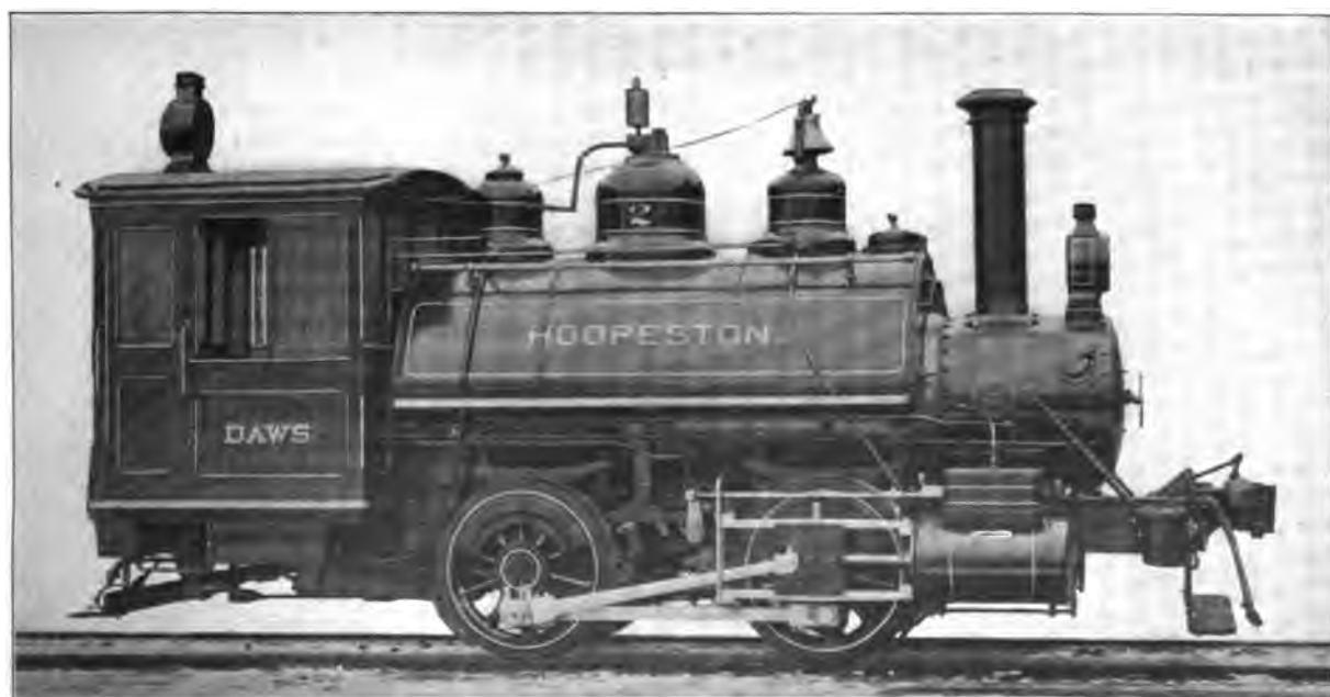
Fig. 6. Four-Wheel (0—4—0) Tank Switching Locomotive. Built by the Baldwin Locomotive Works for the Hoopes & Townsend Co. Cylinders 13 in. x 20 in., Working Steam Pressure 160 lbs. per sq. in., Heating Surface 414.74 sq. ft., Diameter of Drivers 42 in., Weight on Drivers 50,000 lbs., Total Weight 50,000 lbs.
