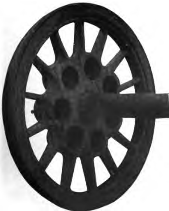
Fig. 4697. Inside View of Driving Wheel Showing Pockets for Driving Pins on Quill.
