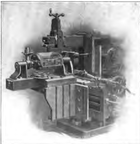
Fig. 5251. Draw Cut Shaper Attachment for Planing Brass Shells for Axle Boxes. Morton Mfg. Co.
