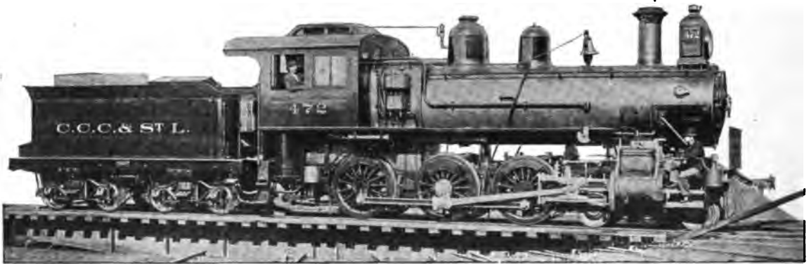
Fig. 64. Ten-Wheel (4-6-0) Richmond Compound Locomotive. Built by the American Locomotive Co. for the Cleveland, Cincinnati, Chicago & St. Louis. Cylinders 19 in. and 30 in. x 24 in., Working Steam Pressure 180 lbs. per sq. in., Diameter of Drivers 53 in., Weight on Drivers 108,000 lbs., Total Weight 178,000 lbs.
