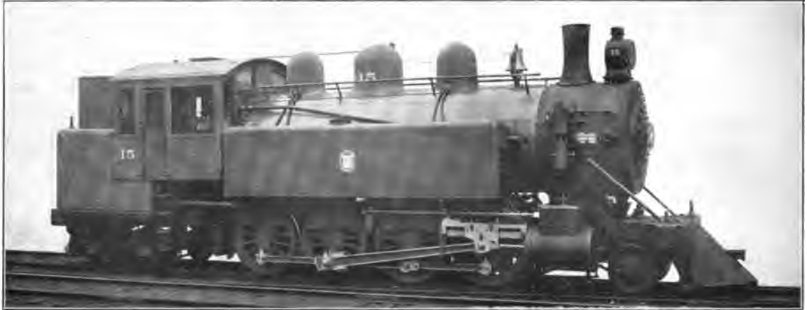
Fig. 48. Eight-Coupled (2-8-4) Tank Locomotive. Built by the American Locomotive Co. for the Dominion Coal Co. Cylinders 22 in. x 28 in., Working Steam Pressure 200 lbs. per sq. in., Heating Surface 2,687.47 sq. ft., Diameter of Drivers 55 in., Weight on Drivers 170,000 lbs., Total Weight 239,000 lbs.
