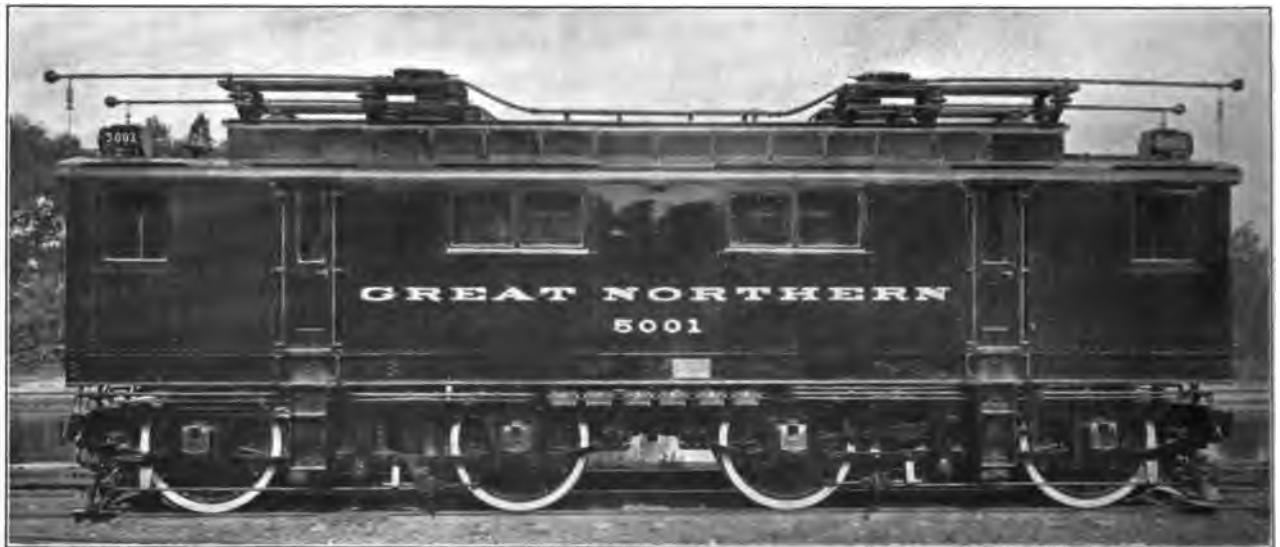
Fig. 4708. 115-Ton Electric Locomotive for the Great Northern Railway. Built by the General Electric and American Locomotive Companies.
