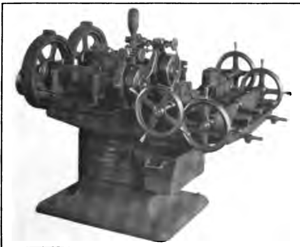
Fig. 5098. 1½-Inch Double Bolt Cutter. Can be fitted with holders for threading pipe nippers. Acme Machinery Co.
