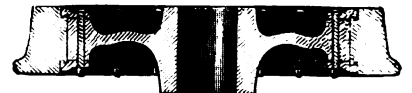
Figs. 4539-4540. No. 1 Krupp Wheel. Forged Steel Disc Center. Tire Secured by Wrought Iron Retaining Rings.
