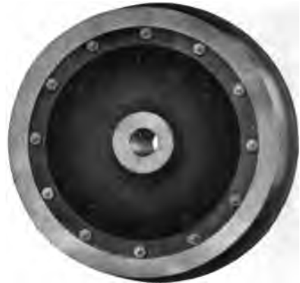
Figs. 4563-4564. Cast-iron Plate Center held by Shrinkage and Bolts.
