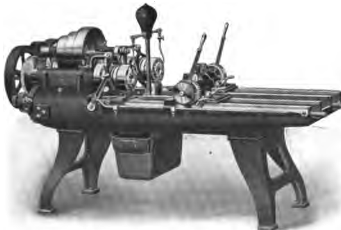
Fig. 5102. Triple-Head Bolt Cutter, All Steel Die Head. Landis Machine Co.
