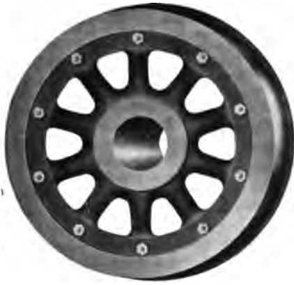
Figs. 4557-4558. (For Engine Trucks.) Cast-iron or Cast-steel Spoke Center held by Shrinkage and Bolts.
