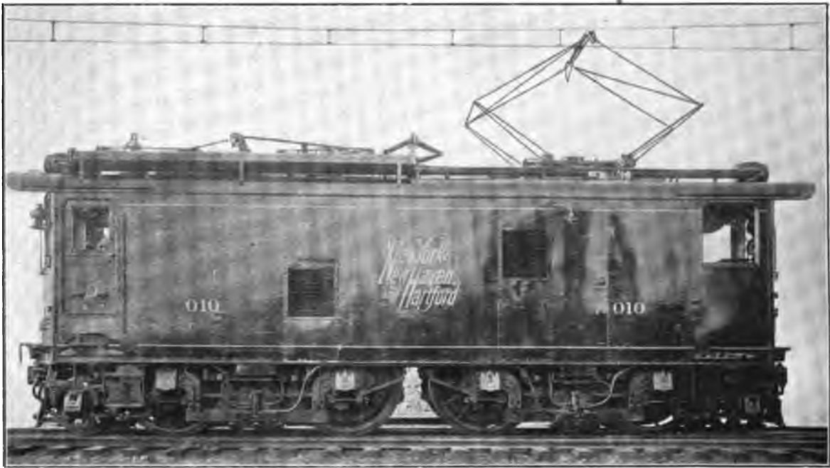
Fig. 4689. Electric Locomotive for Single-Phase Alternating or Direct Current Operation. New York, New Haven & Hartford. Built by the Westinghouse Electric & Mfg. Co. and the Baldwin Locomotive Works.
