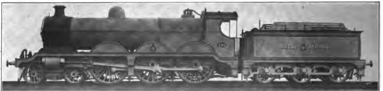
Figs. 4994. Ten-Wheel, Six-Coupled Locomotive. Great Central Railway. Cylinders 19½ in. x 26 in.; Working Steam Pressure 180 lbs. per sq. in.; Total Heating Surface 1,917 sq. ft.
