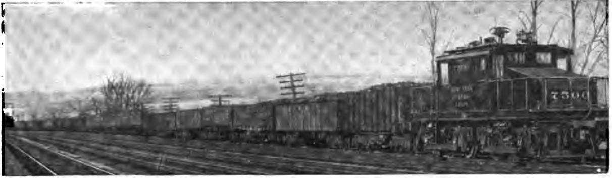
Detroit River Tunnel Co. Locomotive Hauling 26-Car Train, Total Weight 1578 Tons
