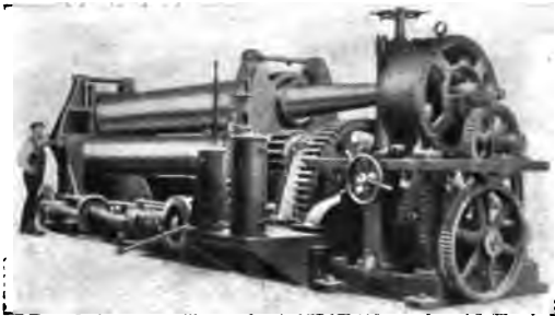
Westinghouse Motor Driving Bending Rolls.
