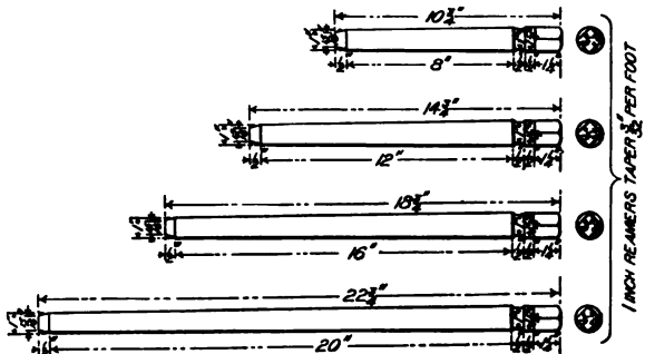
Figs. 4750-4757. Standard Taper Reamers.
