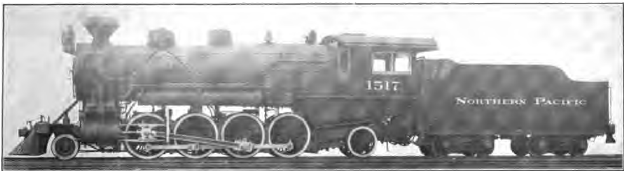
Fig. 47. Mikado (2—8—2) Type Locomotive. Built by the American Locomotive Co. for the Northern Pacific. Cylinders 24 in. x 30 in., Working Steam Pressure 200 lbs. per sq. in., Heating Surface 4,007 sq. ft., Diameter of Drivers 63 in., Weight on Drivers 196,000 lbs., Total Weight 259,000 lbs.
