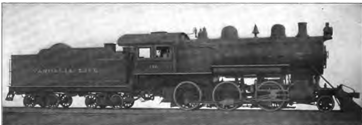
Fig. 36. Mogul (2—6—0) Locomotive. Built by the American Locomotive Co. for the Vandalia Line. Cylinders 21 in. x 28 in., Working Steam Pressure 200 lbs. per sq. in., Total Heating Surface 2,935 sq. ft., Diameter of Drivers 63 in., Weight on Drivers 156,500 lbs., Total Weight 182,500 lbs.
