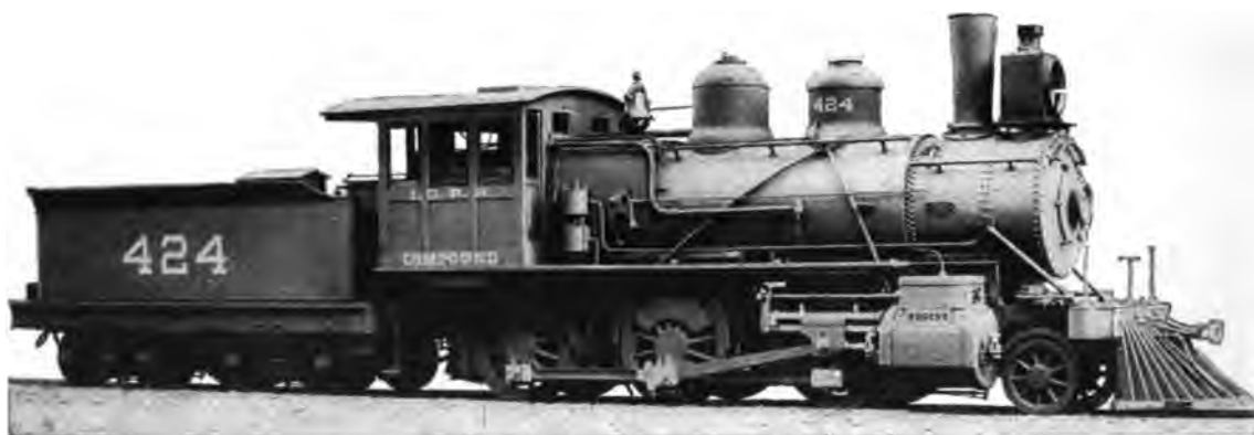
Fig. 34. Mogul (2—6—0) Two-Cylinder Compound Locomotive. Built by the Rogers Locomotive Works for the Illinois Central. Cylinders 20 in. and 29 in. x 26 in., Working Steam Pressure 200 lbs. per sq. in., Diameter of Drivers 56½ in., Weight on Drivers 107,000 lbs., Total Weight 129,000 lbs.
