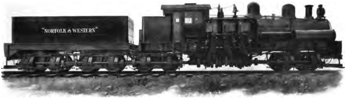
Fig. 130. Sixteen-Wheel Shay Geared Locomotive. Built by the Lima Locomotive & Machine Co. for the Norfolk & Western Railway. Cylinders, 3 in Number, 17-in. Diameter, 18-in. Stroke; Drivers, 46-in. Diameter; Working Steam Pressure, 200 lbs.; Total Heating Surface, 2,400 sq. ft.; Total Weight, 155 Tons.
