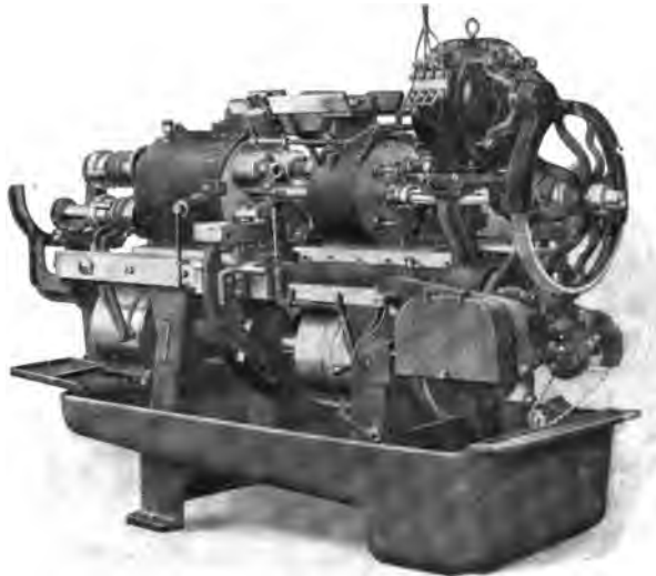
Fig. 5239. Motor-Driven Automatic Multiple-Spindle Screw Machine. National-Acme Manufacturing Co.
