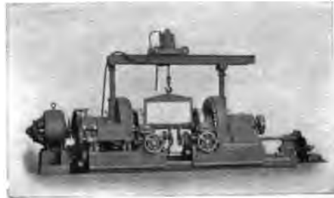
Westinghouse Motor Driving Car Wheel Lathe
