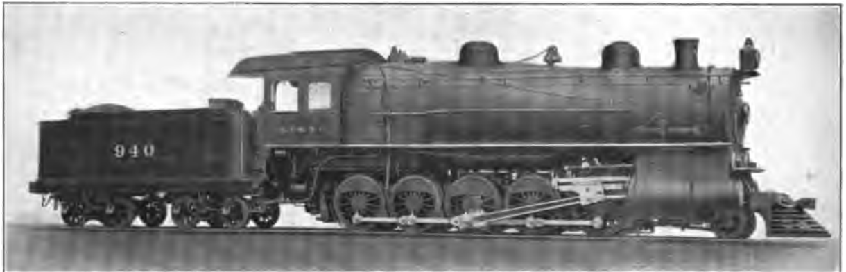
Fig. 49. Decapod (2-10-0) Tandem Compound Locomotive. Built by the Baldwin Locomotive Works for the Atchison, Topeka & Santa Fe. Cylinders 19 in. and 32 in. x 32 in., Working Steam Pressure 225 lbs. per sq. in., Total Heating Surface 5,390 sq. ft., Diameter of Drivers 57 in., Weight on Drivers 237,800 lbs., Total Weight 267,800 lbs.
