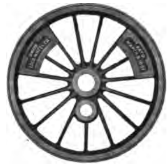
Fig. 1326. Cast-Steel Driving Wheel Center with Davis Counterbalance. Davis Loco. Wheel Co.
