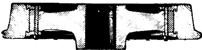
Figs. 4535-4536. No. 3 Krupp Wheel. Cast Iron Spoke Center. Tire Secured by Wrought Iron Retaining Rings.
