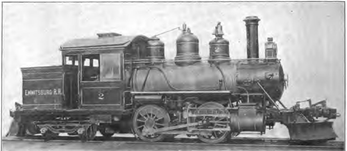
Fig. 13. Forney Four-Coupled (0-4-4) Locomotive with Four-Wheel Rear Truck. Built by the Baldwin Locomotive Works for the Emmitsburg Railroad. Cylinders 13 in. x 20 in., Working Steam Pressure 160 lbs. per sq. in., Total Heating Surface 592.4 sq. ft., Diameter of Drivers 44 in., Weight on Drivers 50,700 lbs., Total Weight 73,000 lbs.
