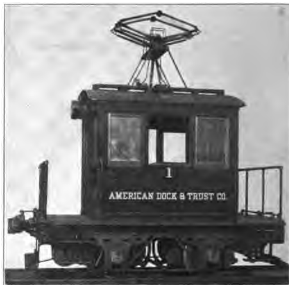
Fig. 4714. Baldwin-Westinghouse Electric Locomotive for the American Dock & Trust Co. Weight, 36,000 lbs.; Wheel Base, 5 ft. 6 in.; Drawbar Pull, Starting, 9,000 lbs.; Drawbar Pull, Running, 6,000 lbs.; No. of Motors, 2.
