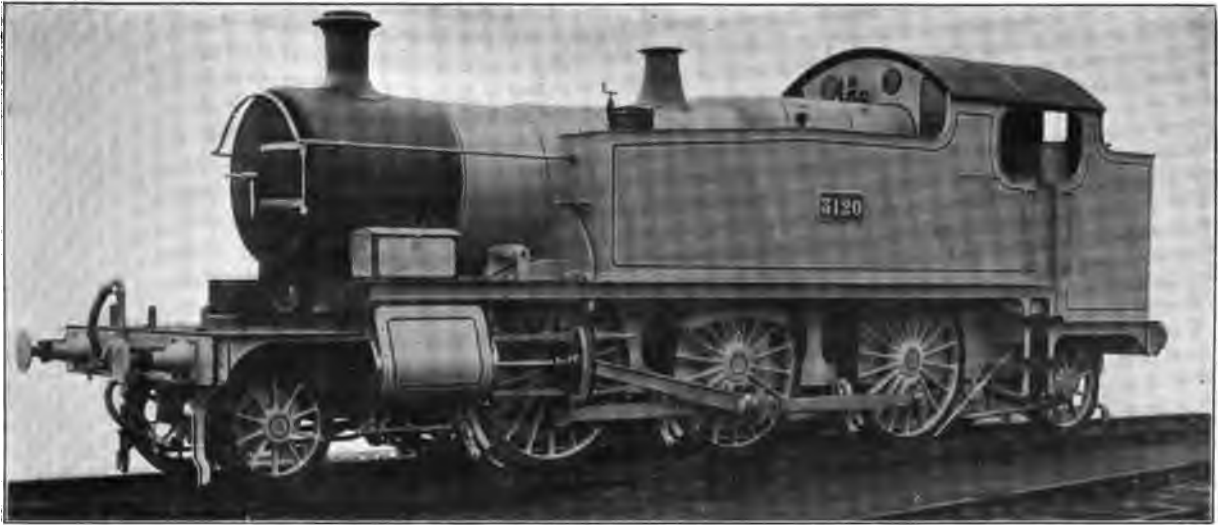
Fig. 4971. Ten-Wheel, Six-Coupled Tank Locomotive. Great Western Railway. Cylinders 18 in. x 30 in.; Working Steam Pressure 195 lbs. per sq. in.; Total Heating Surface 1,517.89 sq. ft.; Weight on Drivers 123,812 lbs.; Total Weight 169,120 lbs.
