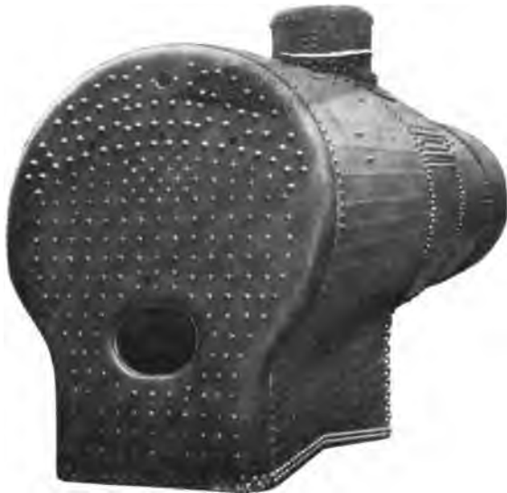
Fig. 146. Rear End View of Extended Wagon Top Boiler with Narrow Firebox.
