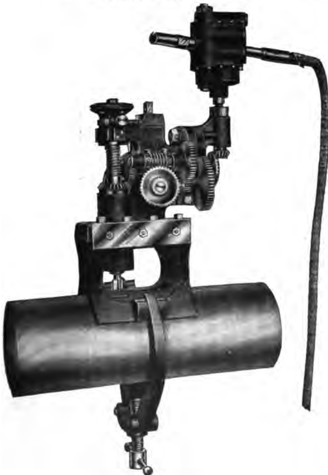
Fig. 5176. Portable Automatic Key Seating Machine. Joseph T. Ryerson & Son.
