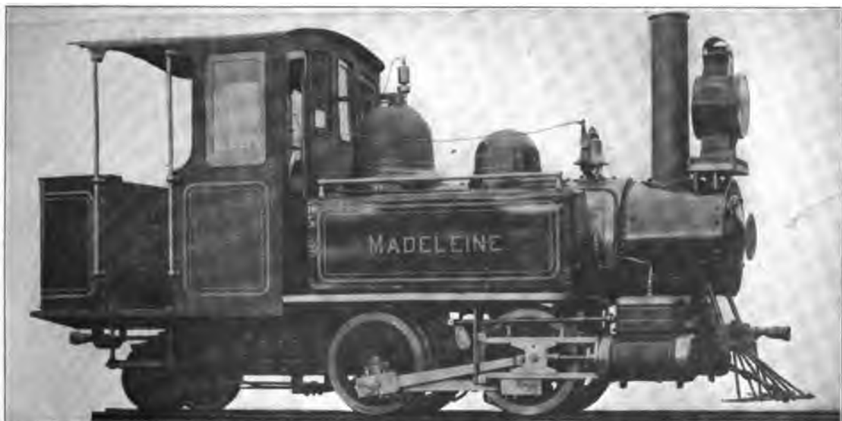
Fig. 11. Four-Coupled (0—4—2) Tank Locomotive with Trailing Truck. Built by the American Locomotive Co. Cylinders 8 in. x 12 in., Working Steam Pressure 180 lbs. per sq. in., Heating Surface 226 sq. ft., Diameter of Drivers 28 in., Weight on Drivers 17,600 lbs., Total Weight 20,300 lbs.
