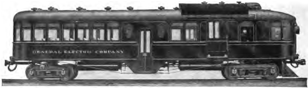
Gas-Electric Car for Passenger and Baggage Service; 45 Passengers.
