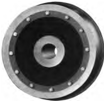
Figs. 4565-4566. Cast-steel Plate Center held by Shrinkage and Bolts.
