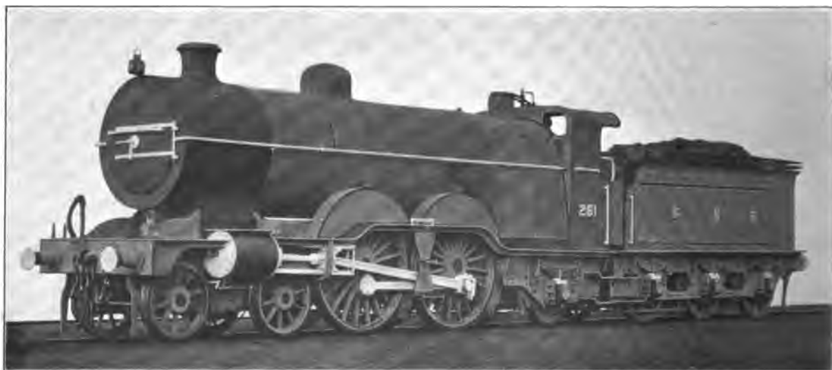
Fig. 4982. Ten-Wheel, Four-Coupled Locomotive. Great Northern Railway. Cylinders 19 in. x 24 in.; Working Steam Pressure 175 lbs. per sq. in.; Total Heating Surface 2,500 sq. ft.; Diameter of Drivers 80 in.; Weight on Drivers 84,640 lbs.; Total Weight 146,720 lbs.
