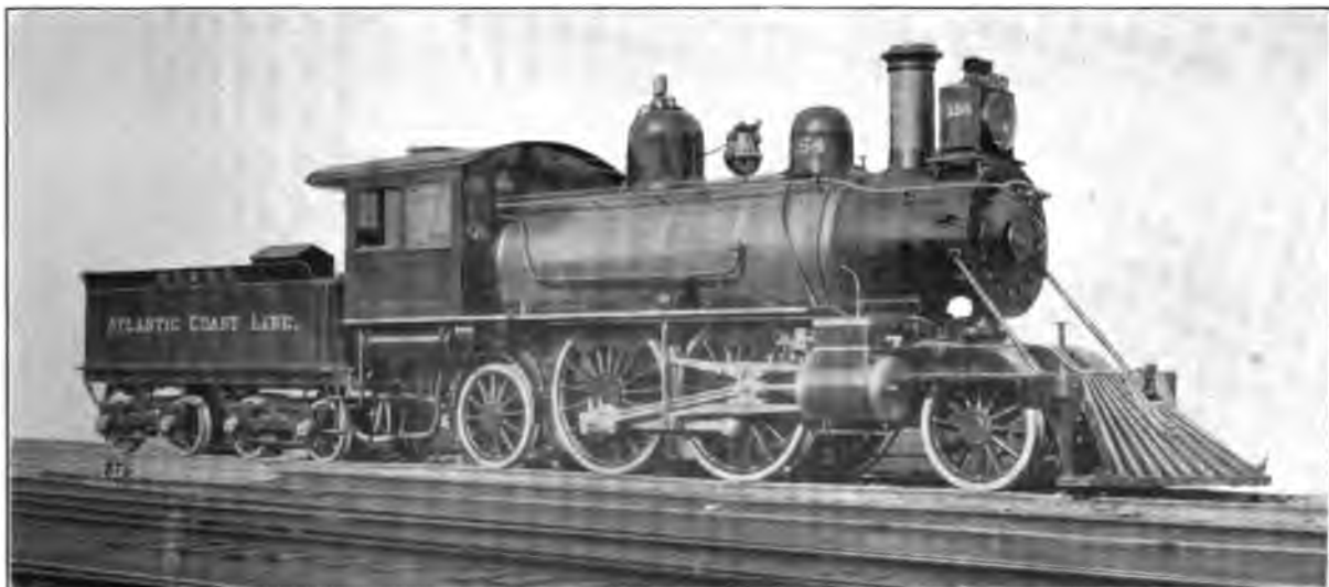
Fig. 25. Columbia (2-4-2) Type Locomotive. Built by the Baldwin Locomotive Works for the Atlantic Coast Line. Cylinders 19 in. x 24 in., Working Steam Pressure 180 lbs. per sq. in., Total Heating Surface 1,686.97 sq. ft., Diameter of Drivers 72 in., Weight on Drivers 75,800 lbs., Total Weight 124,500 lbs.
