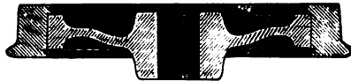
Figs. 4537-4538. No. 14 Krupp Wheel. Disc Center. Steel Tire Secured with Bute Fastening. Thomas Prosser & Son.
