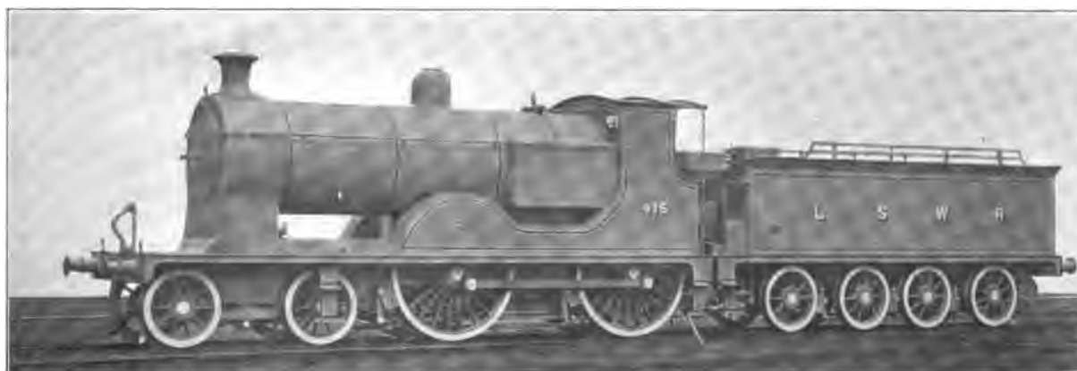
Fig. 4979. Eight-Wheel, Four-Coupled Locomotive, London & South Western. Cylinders 19 in. x 26 in.; Working Steam Pressure 175 lbs. per sq. in.; Total Heating Surface 1,550 lbs.; Diameter of Drivers 79 in.
