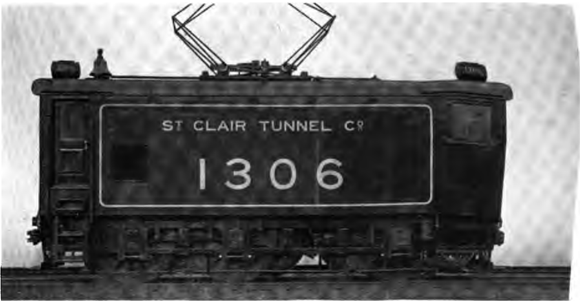
Fig. 4710. 65-Ton Freight Locomotive Used by the St. Clair Tunnel Co. Built by the Westinghouse Electric & Mfg. Co.
