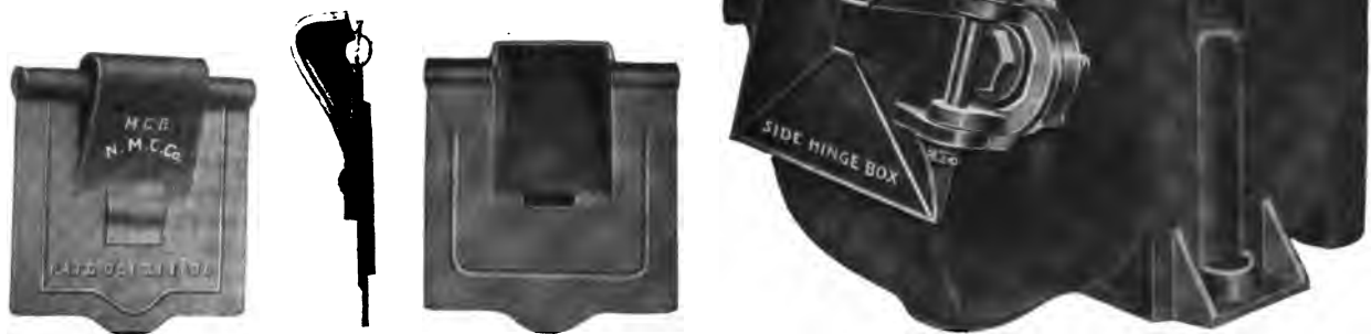
Figs. 4477-4478. M. C. B. Standard Malleable Journal Box Lids made for 3 1/4-in. x 7-in., 4 1/4-in. x 8-in., 5-in. x 9-in. and 5 1/2-in. x 10-in. size Boxes.
