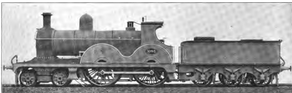
Fig. 4977. Eight-Wheel, Four-Coupled Locomotive, Lancashire & Yorkshire. Working Steam Pressure 160 lbs. per sq. in.; Total Heating Surface 1,261.41 sq. ft.; Diameter of Drivers 87 in.; Weight on Drivers 69,440 lbs.; Total Weight 100,360 lbs.
