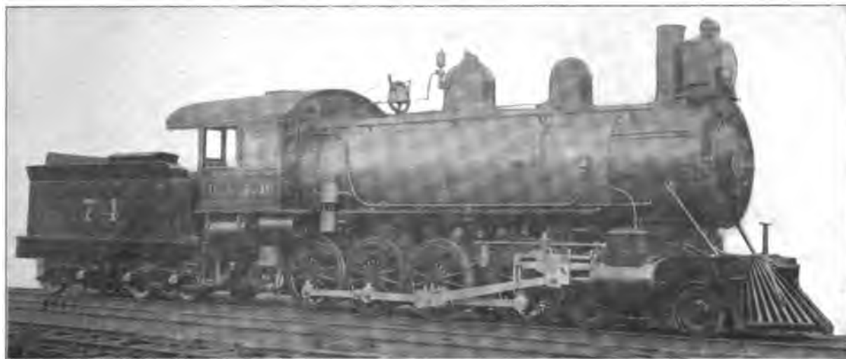
Fig. 76. Twelve-Wheel (4-8-0) Locomotive. Built by the Baldwin Locomotive Works for the Duluth & Iron Range. Cylinders 22 in. x 26 in., Diameter of Drivers 54 in., Weight on Drivers 140,060 lbs., Total Weight 172,260 lbs.
