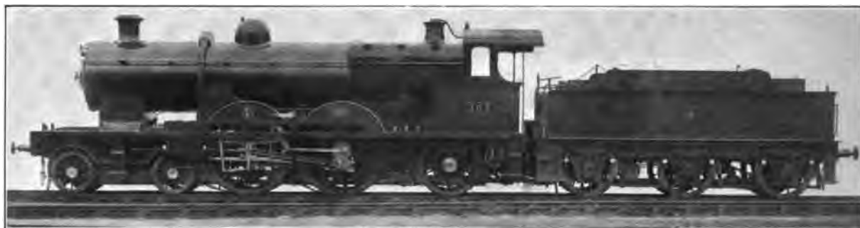
Fig. 4986. Ten-Wheel, Four-Coupled, De Glehn, Four-Cylinder Balanced Compound Locomotive. Great Western Railway. Cylinders 14\frac{1}{8} in. and 23\frac{3}{8} in. x 25\frac{7}{8} in.; Working Steam Pressure 227 lbs. per sq. in.; Total Heating Surface 2,755.7 sq. ft.; Weight on Drivers 75,040 lbs.; Total Weight 159,940 lbs.
