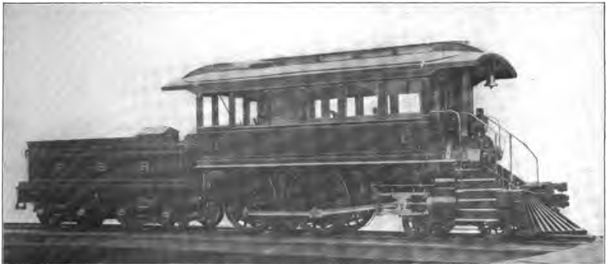
Fig. 56. Eight-Wheel (4—4—0) Inspection Locomotive. Built by the Baldwin Locomotive Works for the Philadelphia & Reading. Cylinders 17 in. x 20 in., Working Steam Pressure 200 lbs. per sq. in., Heating Surface 999 sq. ft., Diameter of Drivers 60 in., Weight on Drivers 65,000 lbs., Total Weight 99,400 lbs.
