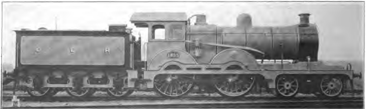
Fig. 4976. Eight-Wheel, Four-Coupled Locomotive. Great Eastern Railway. Cylinders 19 in. x 26 in. Total Heating Surface 1,706.58 sq. ft.; Diameter of Drivers 84 in.; Weight on Drivers 77,040 lbs.; Total Weight 115,850 lbs.
