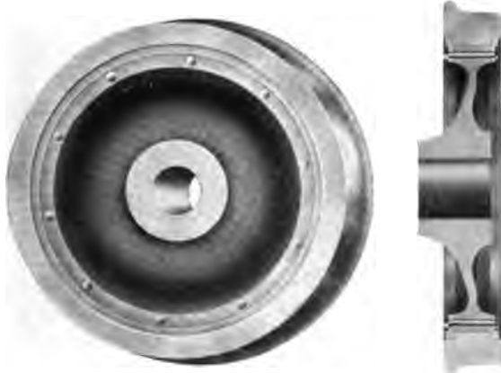
Figs. 4577-4578. Cast-steel Plate Center held by Shrinkage, Mansell Retaining Rings and Bolts.
