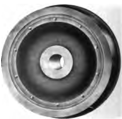
Figs. 4571-4572. Cast-iron Plate Center held by Shrinkage, Mansell Retaining Rings and Rivets.
