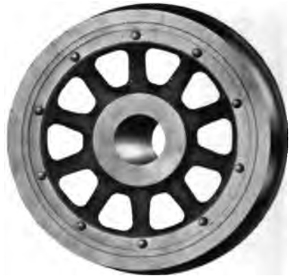
Figs. 4559-4560. (For Engine Trucks.) Cast-iron or Cast-steel Spoke Center held by Shrinkage. Double Lip Retaining Rings and Rivets.
