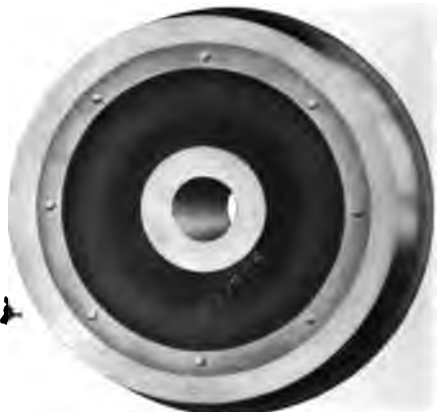
Figs. 4567-4568. Cast-iron Plate Center held by Shrinkage, Double Lip Retaining Rings and Rivets.
