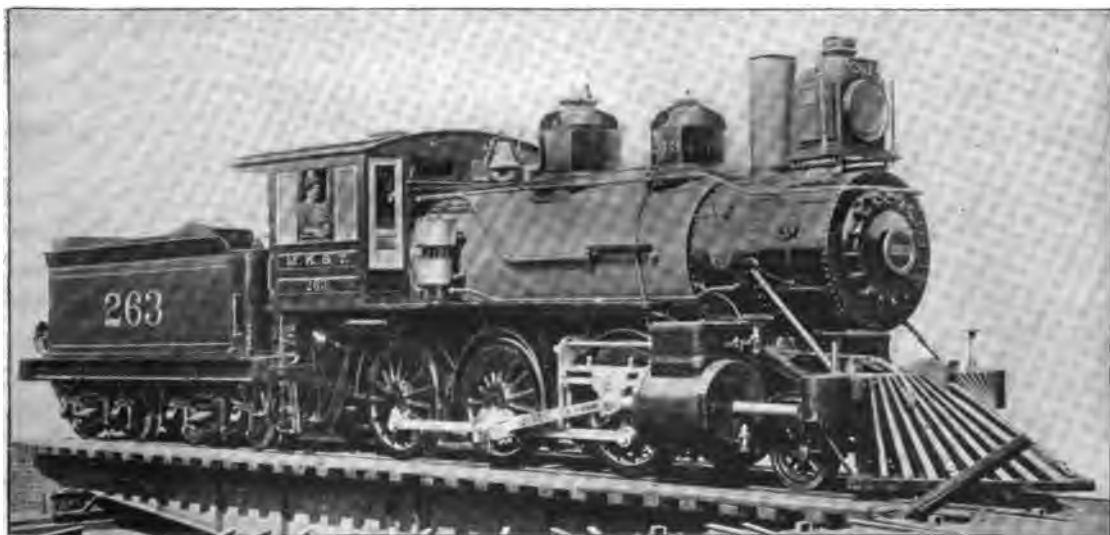
Fig. 33. Mogul (2-6-0) Richmond Compound Locomotive. Built by the American Locomotive Co. for the Missouri, Kansas & Texas. Cylinders 19 in. and 30 in. x 24 in., Working Steam Pressure 170 lbs., per sq. in., Diameter of Drivers 56 in., Weight on Drivers 107,000 lbs., Total Weight 120,000 lbs.
