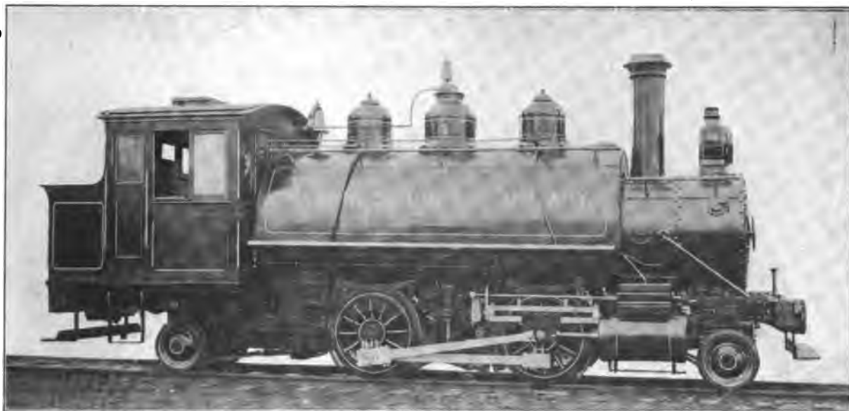
Fig. 28. Four-Coupled Double Ender (2—4—2) Tank Locomotive. Built by the Baldwin Locomotive Works for the Hastings Lumber Co. Cylinders 16 in. x 22 in., Working Steam Pressure 160 lbs. per sq. in., Total Heating Surface 1,062 sq. ft., Diameter of Drivers 44 in., Weight on Drivers 62,000 lbs., Total Weight 86,000 lbs.
