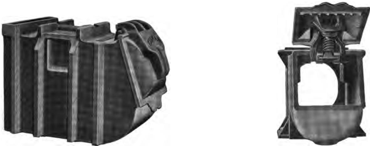
Figs. 4471-4472. Climax Journal Box for Passenger Cars and Open View.
