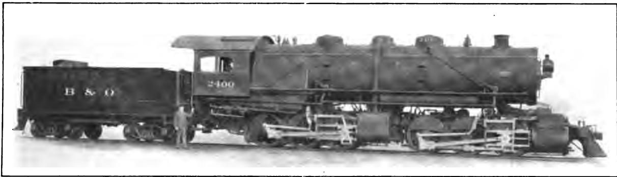
Fig. 23. Twelve-Wheel (0-6-6-0) Mallet Articulated Compound Locomotive. Built by the American Locomotive Co. for the Baltimore & Ohio. Cylinders 20 in. and 32 in. x 32 in., Working Steam Pressure 235 lbs. per sq. in., Total Heating Surface 5,585.7 sq. ft., Diameter of Drivers 56 in., Weight on Drivers 334,500 lbs., Total Weight 334,500 lbs.
