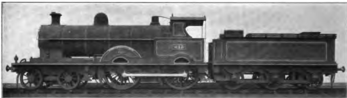
Fig. 4980. Eight-Wheel, Four-Coupled Locomotive. London & North Western. Cylinders 19 in. x 26 in.; Working Steam Pressure 175 lbs. per sq. in.; Total Heating Surface 2,009.7 sq. ft.; Diameter of Drivers 81 in.
