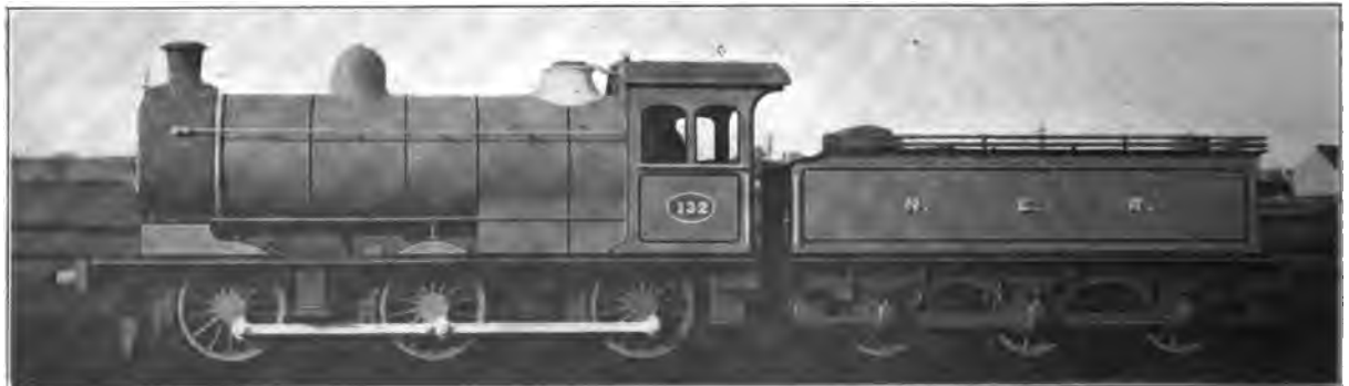
Fig. 4958. Six-Coupled Goods Locomotive. North Eastern Railway. Cylinders 18\frac{1}{2} in. \times 26 in.; Total Heating Surface 1,658 sq. ft.; Diameter of Drivers 55\frac{1}{2} in.; Weight on Drivers 106,740 lbs.; Total Weight 106,740 lbs.
