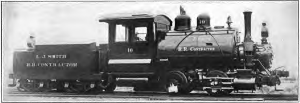
Fig. 7. Four-Wheel (0-4-0) Contractor's Locomotive. Built by the Davenport Locomotive Works. Cylinders 15 in. x 20 in., Working Steam Pressure 170 lbs., Heating Surface 720 sq. ft., Diameter of Drivers 42 in., Weight on Drivers 76,000 lbs.
