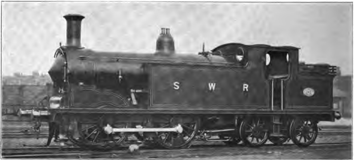
Fig. 4956. Eight-Wheel, Four-Coupled Tank Locomotive. London & South Western. Cylinders 18\frac{1}{2} in. \times 26 in.; Working Steam Pressure 175 lbs. per sq. in.; Total Heating Surface 1,191.68 sq. ft.; Diameter of Drivers 67 in.; Total Weight 122,500 lbs.
