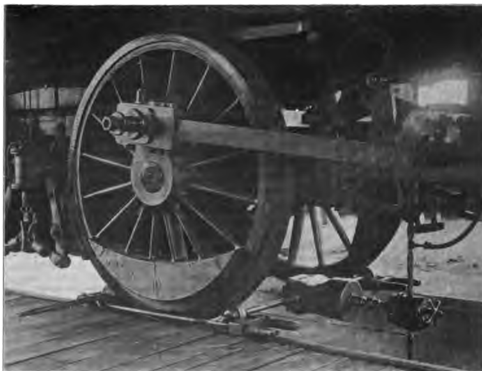
Fig. 5262. Farrington's Valve Setting Machine, Fitted with Mills Power Attachment. Sherburne & Co.
