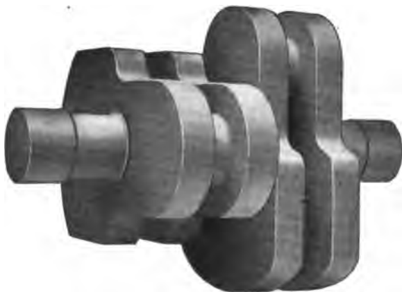
Fig. 2185. Built-up Crank Axle with Weights Balanced in Same Plane.
