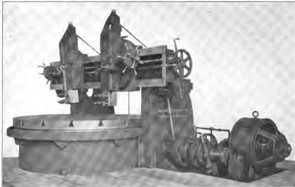
Fig. 5121. 84-Inch Tire Turning Mill. Betts Machine Co.
