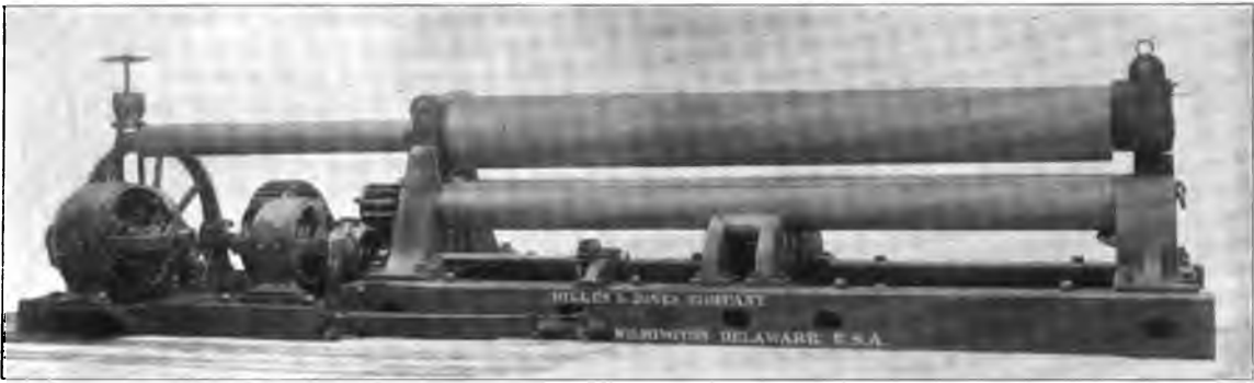
Fig. 5095. Heavy Plate Bending Rolls, Provided with Two Motors. One for Driving the Lower Rolls and the Other for Raising and Lowering the Top Rolls. Hilles & Jones Co.
