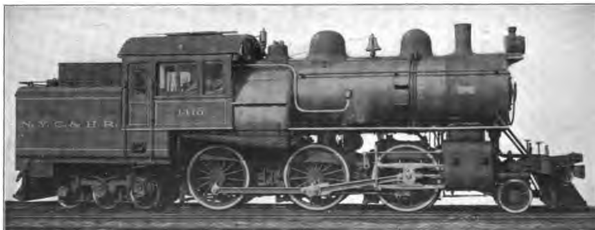
Fig. 39. Six-Coupled Double Ender (2-6-6) Locomotive. Built by the American Locomotive Co. for the New York Central & Hudson River. Cylinders 20 in. x 24 in., Working Steam Pressure 200 lbs. per sq. in., Total Heating Surface 2,425.3 sq. ft., Diameter of Drivers 63 in., Weight on Drivers 128,000 lbs., Total Weight 216,000 lbs.
