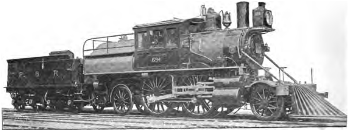
Fig. 26. Columbia (2—4—2) Type Compound Locomotive. Built by the Baldwin Locomotive Works for the Philadelphia & Reading. Cylinders 13 in. and 22 in. x 24 in., Working Steam Pressure 180 lbs. per sq. in., Diameter of Drivers 78 in., Weight on Drivers 78,000 lbs., Total Weight 125,000 lbs.
