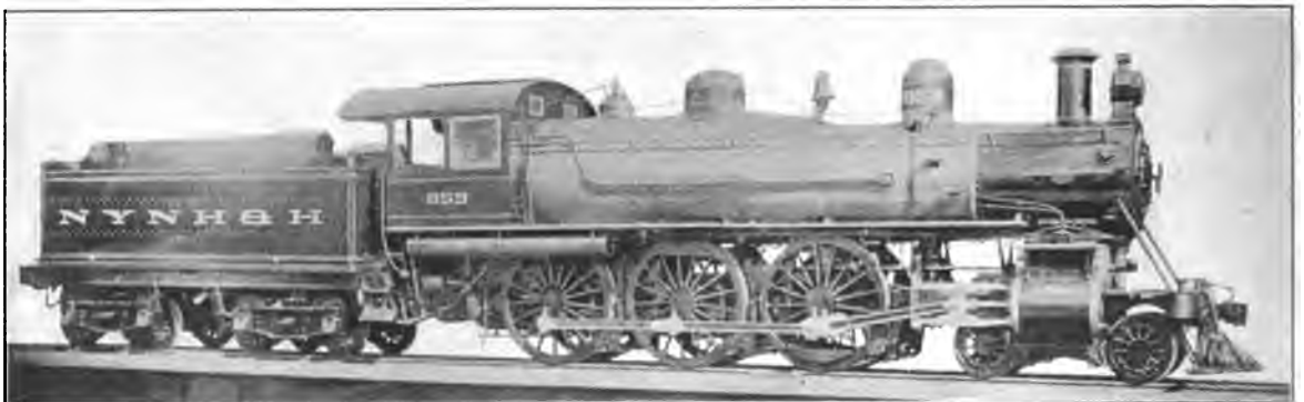
Fig. 66. Ten-Wheel (4-6-0) Vauclain Balanced Compound Locomotive. Built by the Baldwin Locomotive Works for the New York, New Haven & Hartford. Cylinders 15 in. and 25 in. x 26 in., Working Steam Pressure 200 lbs. per sq. in., Heating Surface 2,636 sq. ft., Diameter of Drivers 72 in., Weight on Drivers 123,100 lbs., Total Weight 160,600 lbs.
