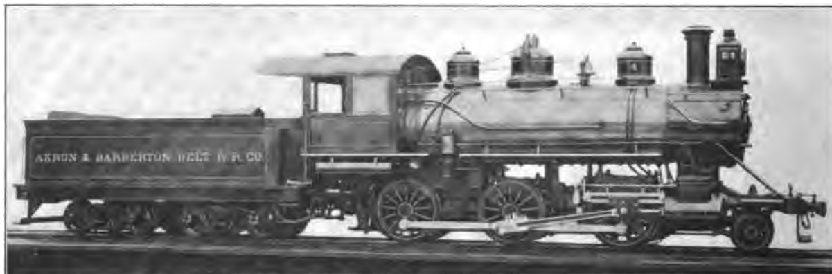
Fig. 35. Mogul (2—6—0) Locomotive. Built by the Baldwin Locomotive Works for the Akron & Barberton Belt Railroad. Cylinders 20 in. x 24 in., Working Steam Pressure 180 lbs. per sq. in., Heating Surface 1,829.3 sq. ft., Diameter of Drivers 56 in., Weight on Drivers 115,000 lbs., Total Weight 132,000 lbs.
