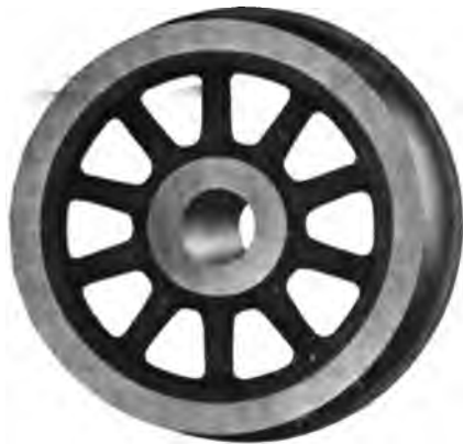
Figs. 4561-4562. (For Engine Trucks.) Cast-iron or Cast-steel Spoke Center held by Shrinkage and Shoulder.
