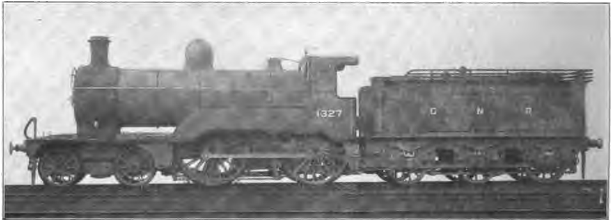
Fig. 4975. Eight-Wheel, Four-Coupled Locomotive. Great Northern Railway. Cylinders 17\frac{1}{2} in. x 26 in.; Working Steam Pressure 170 lbs. per sq. in.; Total Heating Surface 1,249.8 sq. ft.; Diameter of Drivers 80 in.; Weight on Drivers 69,440 lbs.; Total Weight 106,400 lbs.
