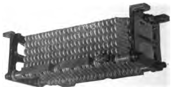
Fig. 4702. Grid Resistance. Westinghouse A. C. Electric Locomotive.
