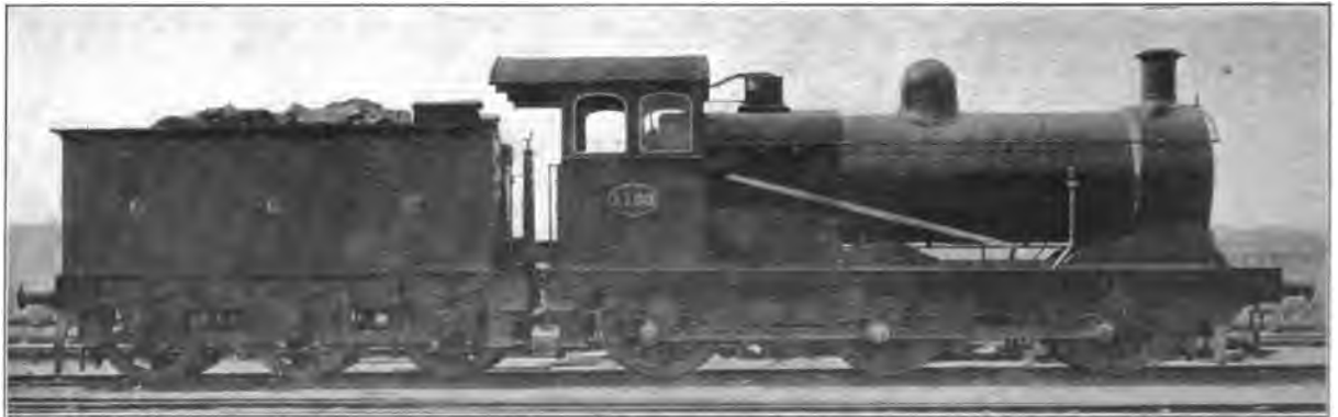
Fig. 4962. Six-Coupled Goods Locomotive. Great Eastern Railway. Cylinders 19 in. x 26 in.; Total Heating Surface 1,706.58 sq. ft.; Diameter of Drivers 59 in.; Weight on Drivers 102,680 lbs.; Total Weight 102,680 lbs.
