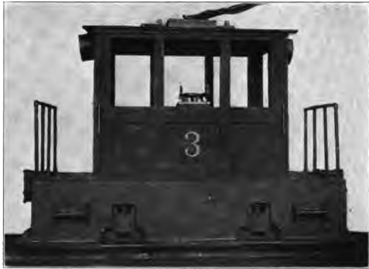
Fig. 4719. Baldwin-Westinghouse Electric Locomotive for the Pennsylvania Steel Co. Weight, 28,000 lbs.; Diameter of Drivers, 30 in.; Wheel Base, 5 ft. 6 in.; Drawbar Pull, 5,600 lbs.; No. of Motors, 2.
