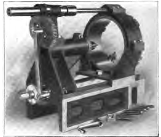
Fig. 5123. Portable Crank Pin Turning Machine. H. B. Underwood & Co.
