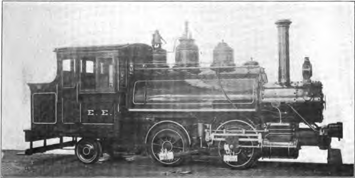
Fig. 10. Four-Coupled (0—4—2) Tank Locomotive with Trailing Truck. Built by the Baldwin Locomotive Works for the Embreeville Estate. Cylinders 10 in. x 16 in., Working Steam Pressure 160 lbs. per sq. in., Heating Surface 340 sq. ft., Diameter of Drivers 36 in., Weight on Drivers 32,440 lbs., Total Weight 37,140 lbs.
