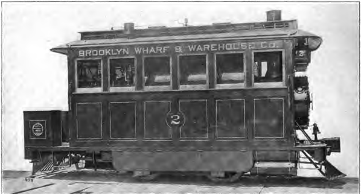
Fig. 8. Four-Wheel (0-4-0) Compound Switching Locomotive. Built by the Baldwin Locomotive Works for the Brooklyn Wharf & Warehouse Co. Cylinders 10 in. and 17 in. x 24 in., Working Steam Pressure 186 lbs. per sq. in., Heating Surface 676.56 sq. ft., Diameter of Drivers 41 in., Weight on Drivers 78,770 lbs., Total Weight 78,770 lbs.
