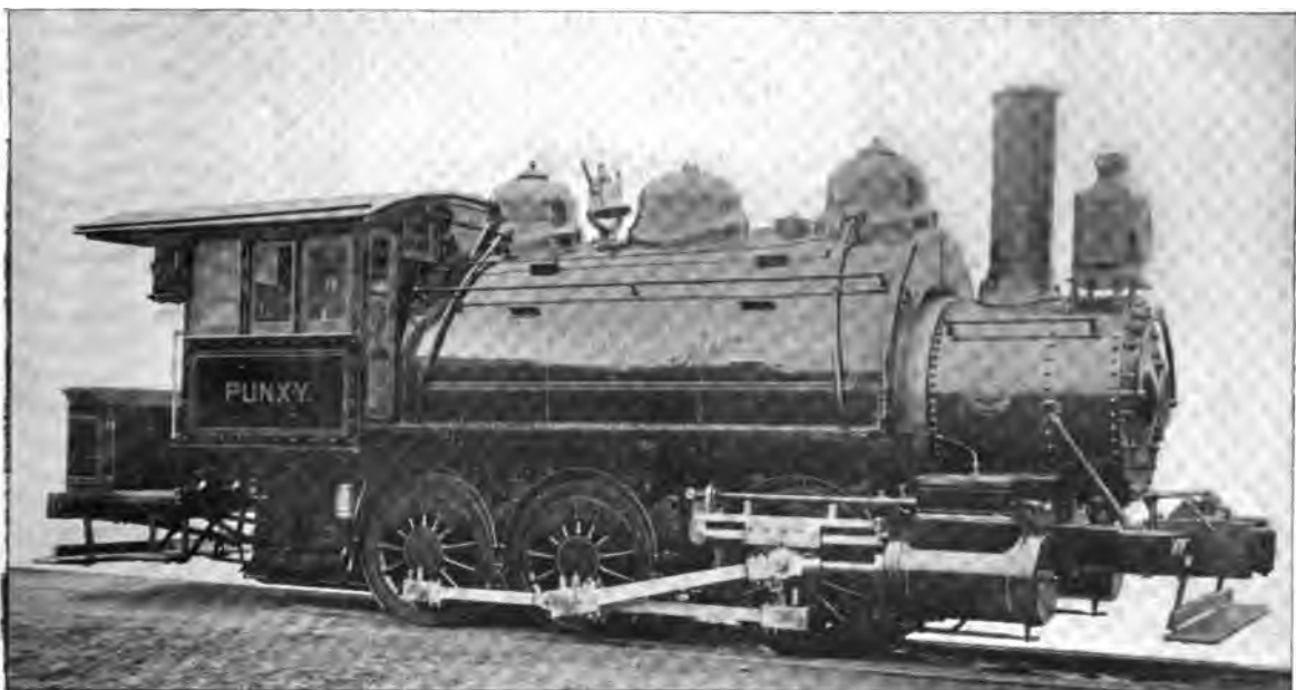
Fig. 15. Six-Wheel (0-6-0) Tank Switching Locomotive. Built by the American Locomotive Co. Cylinders 17 in. x 24 in., Working Steam Pressure 180 lbs. per sq. in., Diameter of Drivers 46 in., Weight on Drivers 96,000 lbs., Total Weight 96,000 lbs.
