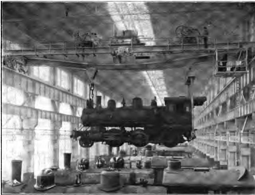
Fig. 5126. 120-Ton Crane, Grand Trunk Railway Shops at Battle Creek, Mich. Morgan Engineering Co.
