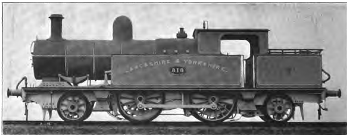
Fig. 4969. Eight-Wheel, Four-Coupled Tank Locomotive with Radial Axle Boxes. Lancashire & Yorkshire. Cylinders 17½ in. x 26 in.; Working Steam Pressure 160 lbs. per sq. in.; Total Heating Surface 1,216.41 sq. ft.; Diameter of Drivers 68 in.; Weight on Drivers 78,960 lbs.; Total Weight 135,520 lbs.
