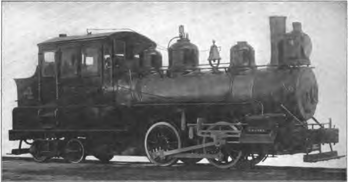
Fig. 12. Forney Four-Coupled (0-4-4) Locomotive with Four-Wheel Rear Truck. Built by the American Locomotive Co. Cylinders 17 in. x 24 in., Working Steam Pressure 165 lbs. per sq. in., Total Heating Surface 1,209 sq. ft., Diameter of Drivers 50 in., Weight on Drivers 80,500 lbs., Total Weight 113,500 lbs.
