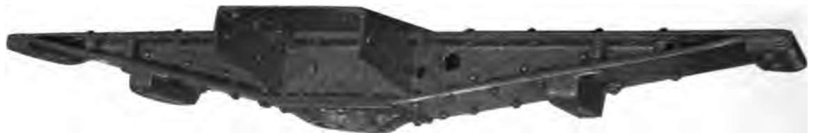
Fig. 4414. Simplex Body Bolster with Plate Web. Simplex Railway Appliance Co.
