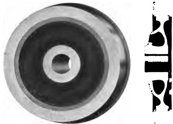
Figs. 4579-4580. Cast-iron Plate Center held by Shrinkage and Gibson Retaining Ring.
