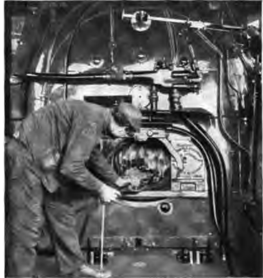
Fig. 334. Pneumatically Operated Horizontal Fire Door. Open Position.
