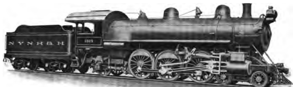
PACIFIC TYPE LOCOMOTIVE FOR THE NEW YORK, NEW HAVEN & HARTFORD RAILROAD COMPANY
