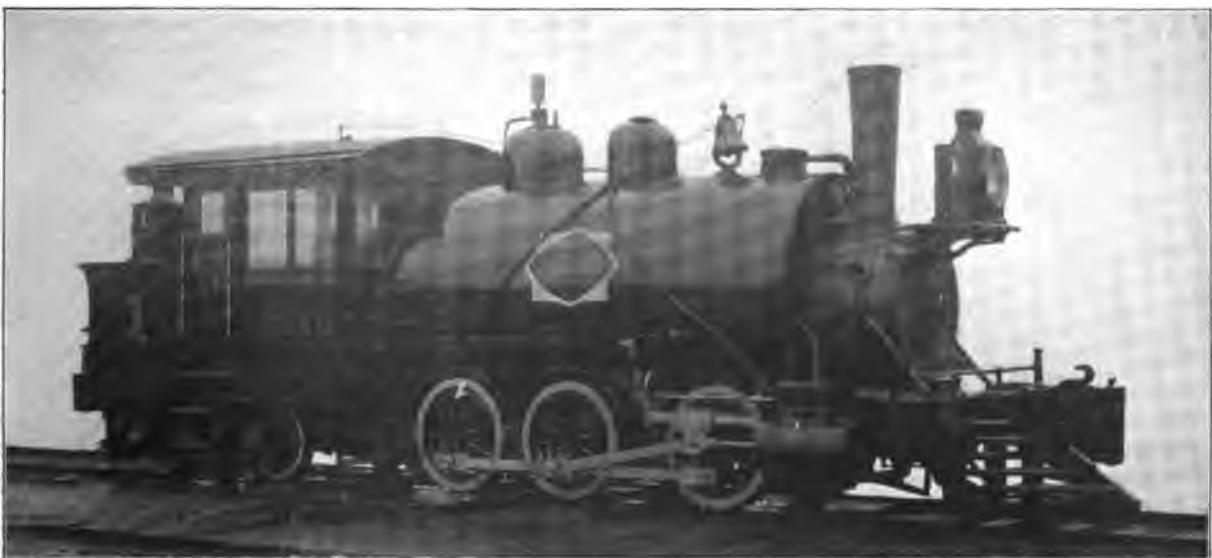
Fig. 19. Six-Coupled (0—6—4) Tank Locomotive. Built by the American Locomotive Co. for the Murphy Lumber Co. Cylinders 13 in. x 18 in., Working Steam Pressure 150 lbs. per sq. in., Heating Surface 723 sq. ft., Diameter of Drivers 33 in., Weight on Drivers 56,200 lbs., Total Weight 69,400 lbs.
