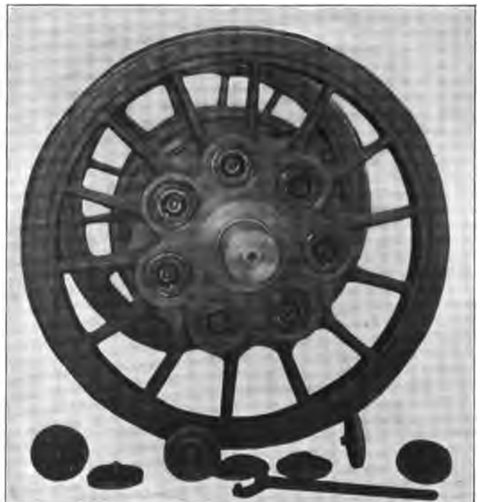
Fig. 4696. Driving Wheel with Caps Removed Showing Pockets for Driving Pins on Quill. Westinghouse A. C. Electric Locomotive.
