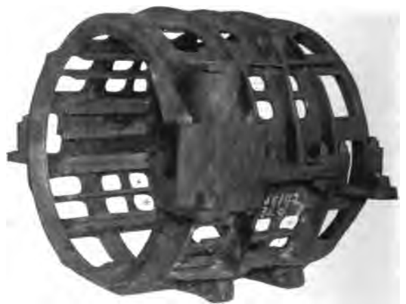
Fig. 4699. Skeleton Field Frame for Gearless Motor. Westinghouse A. C. Electric Locomotive.
