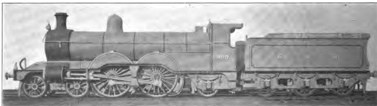
Fig. 4988. Ten-Wheel, Four-Coupled Locomotive. Great Northern Railway. Cylinders 19 in. x 24 in.; Working Steam Pressure 175 lbs. per sq. in.; Total Heating Surface 1,442 sq. ft.; Diameter of Drivers 80 in.; Weight on Drivers 69,440 lbs.; Total Weight 129,920 lbs.
