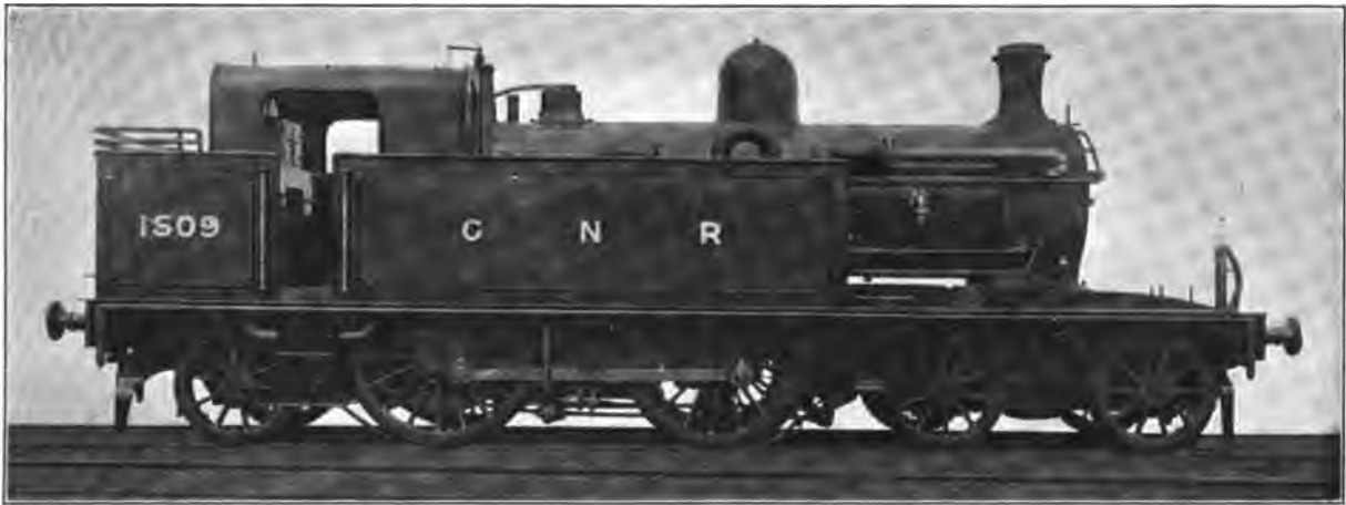
Fig. 4990. Ten-Wheel, Four-Coupled Tank Locomotive. Great Northern Railway. Cylinders 18 in. x 26 in.; Working Steam Pressure 170 lbs. per sq. in.; Total Heating Surface 1,123.8 sq. ft.; Diameter of Drivers 68 in.; Weight on Drivers 80,308 lbs.; Total Weight 138,770 lbs.
