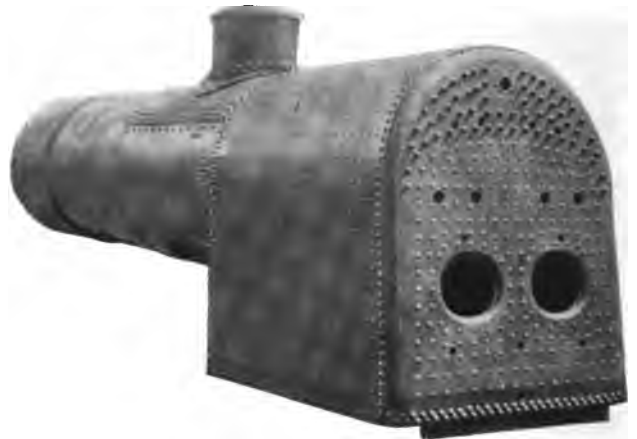
Fig. 147. Rear End View of Extended Wagon Top Boiler with Wide Firebox.
