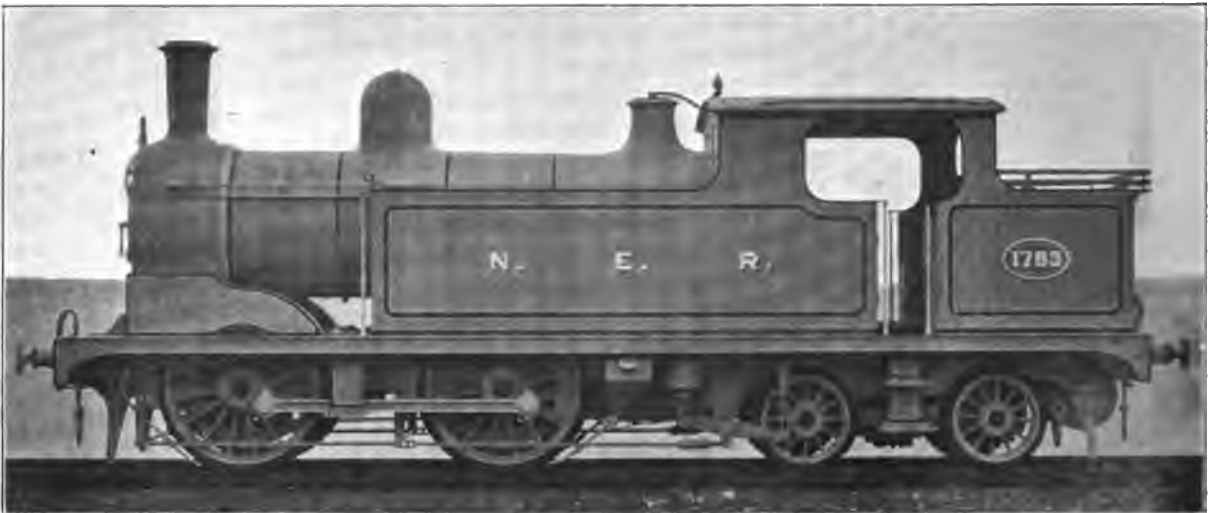
Fig. 4957. Eight-Wheel, Four-Coupled Tank Locomotive. North Eastern Railway. Cylinders 18 in. \times 24 in.; Working Steam Pressure 160 lbs. per sq. in.; Total Heating Surface 1,097 sq. ft.; Weight on Drivers 67,440 lbs.; Total Weight 115,250 lbs.
