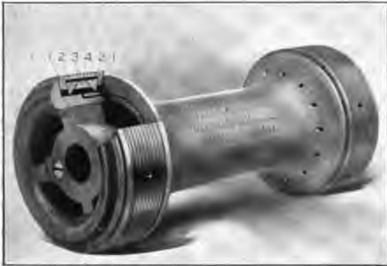
Fig. 2167. Semi-Plug Piston Valve, Showing the Packing Rings.
