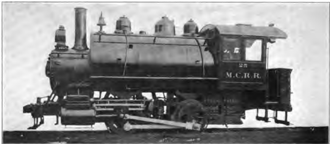
Fig. 3. Four-Wheel (0—4—0) Tank Switching Locomotive. Built by the American Locomotive Co. for the Michigan Central. Cylinders 18 in. x 24 in., Working Steam Pressure 180 lbs. per sq. in., Heating Surface 1,308 sq. ft., Diameter of Drivers 52 in., Weight on Drivers 114,400 lbs., Total Weight 114,400 lbs.
