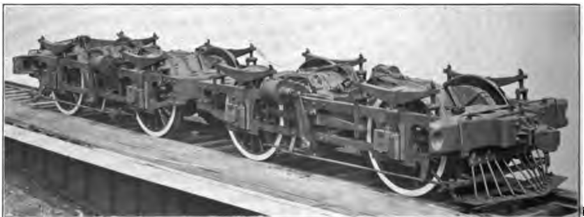
Fig. 4708. 115-Ton Electric Locomotive for the Great Northern Railway. Built by the General Electric and American Locomotive Companies.
