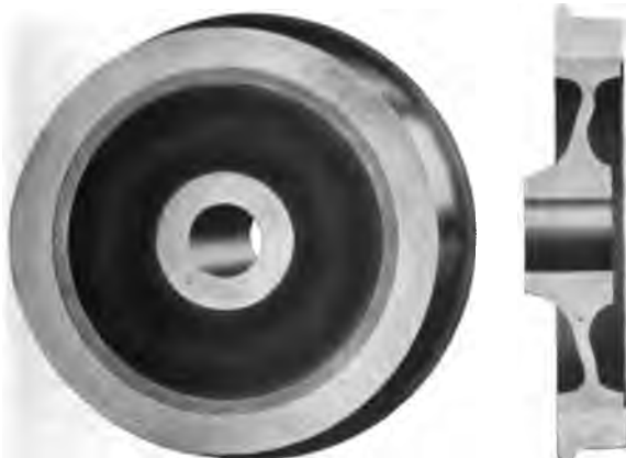
Figs. 4585-4586. Cast-steel Plate Center held by Shrinkage and Shoulder.
