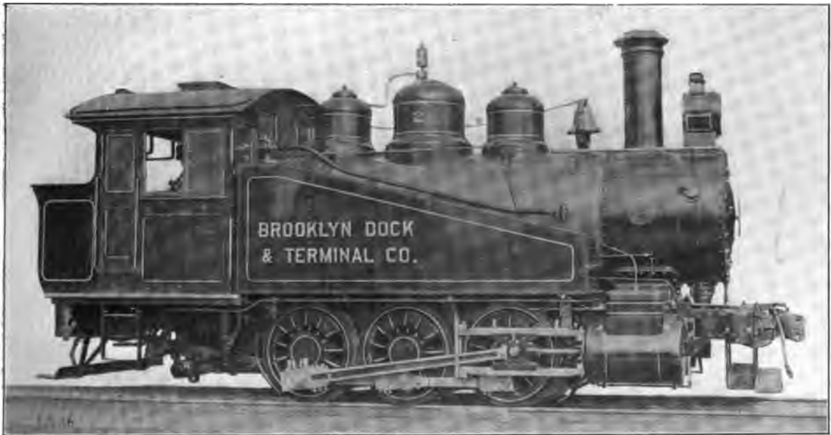
Fig. 14. Six-Wheel (0-6-0) Tank Switching Locomotive. Built by the Baldwin Locomotive Works for the Brooklyn Dock & Terminal Co. Cylinders 19 in. x 24 in., Working Steam Pressure 180 lbs. per sq. in., Total Heating Surface 1,070 sq. ft., Diameter of Drivers 46 in., Weight on Drivers 132,210 lbs., Total Weight 132,210 lbs.
