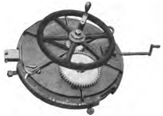
Fig. 5130. Locomotive Cylinder or Dome Facing Machine. H. B. Underwood & Co.
