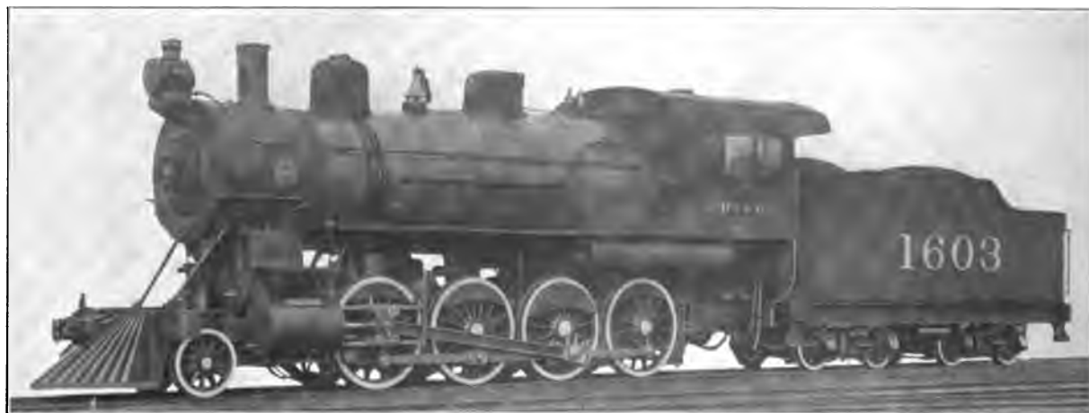
Fig. 41. Consolidation (2-8-0) Locomotive. Built by the American Locomotive Co. for the Chicago, Rock Island & Pacific. Cylinders 22 in. x 30 in., Working Steam Pressure 200 lbs. per sq. in., Heating Surface 3,264 sq. ft., Diameter of Drivers 63 in., Weight on Drivers 182,000 lbs., Total Weight 202,500 lbs.
