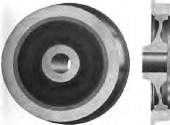
Figs. 4581-4582. Cast-steel Plate Center held by Shrinkage and Gibson Retaining Ring.
