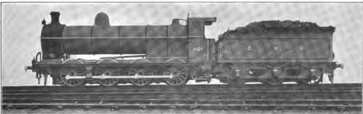
Fig. 4967. Eight-Coupled Goods Locomotive. Great Northern Railway. Cylinders 19 \frac{1}{4} in. x 26 in.; Working Steam Pressure 175 lbs. per sq. in.; Total Heating Surface 1,438.84 sq. ft.; Diameter of Drivers 56 in.; Weight on Drivers 122,340 lbs.; Total Weight 122,340 lbs.
