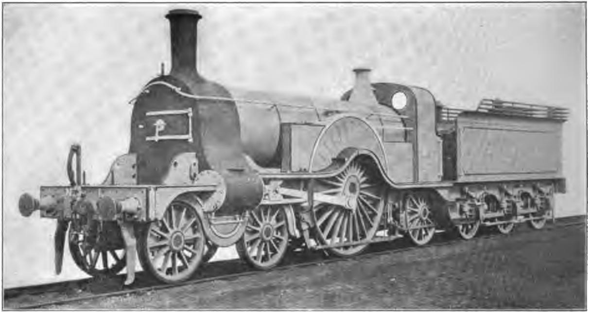
Fig. 4974. Eight-Wheel, Single Driver Locomotive. Great Northern Railway. Cylinders 18 in. x 28 in.; Working Steam Pressure 160 lbs. per sq. in.; Total Heating Surface 1,045 sq. ft.; Diameter of Drivers 98 in.; Weight on Drivers 38,800 lbs.; Total Weight 101,400 lbs.
