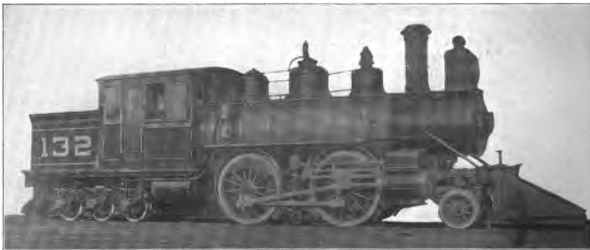
Fig. 31. Four-Coupled Double Ender (2—4—6) Suburban Locomotive. Built by the Baldwin Locomotive Works for the Wisconsin Central. Cylinders 17 in. x 24 in., Working Steam Pressure 130 lbs. per sq. in., Heating Surface 1,284.5 sq. ft., Diameter of Drivers 62 \frac{7}{8} in., Weight on Drivers 61,275 lbs., Total Weight 121,090 lbs.
