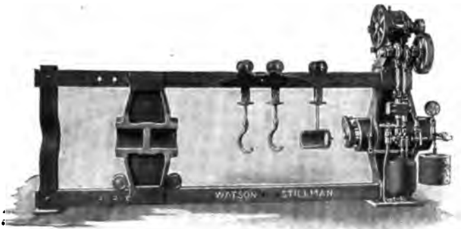
Fig. 5218. Motor Driven Hydro-Pneumatic Wheel Press; Watson-Stillman Co.
