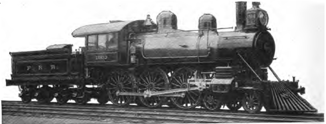
Fig. 65. Ten-Wheel (4-6-0) Two-Cylinder Schenectady Compound Locomotive. Built by the American Locomotive Co. for the Pennsylvania Railroad. Cylinders 20 in. and 30 in. x 24 in., Working Steam Pressure 180 lbs. per sq. in., Diameter of Drivers 74 in., Weight on Drivers 106,000 lbs., Total Weight 143,000 lbs.
