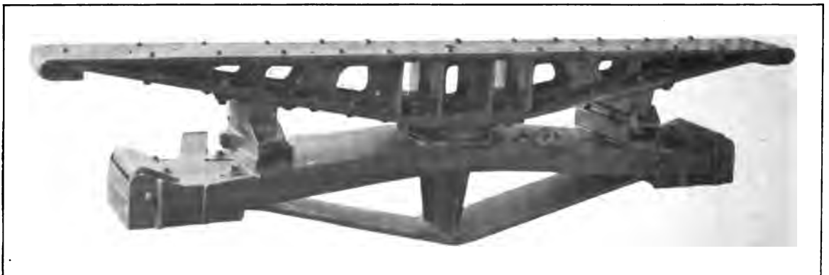
Fig. 4416. Simplex Body and Truck Bearings with Susemihl Side Bearings. Simplex Railway Appliance Co.
