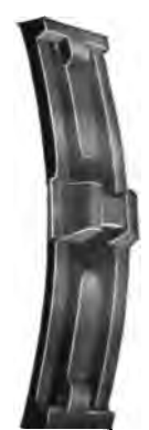
Fig. 2711. Steel Back Shoe, Worn Ort.
