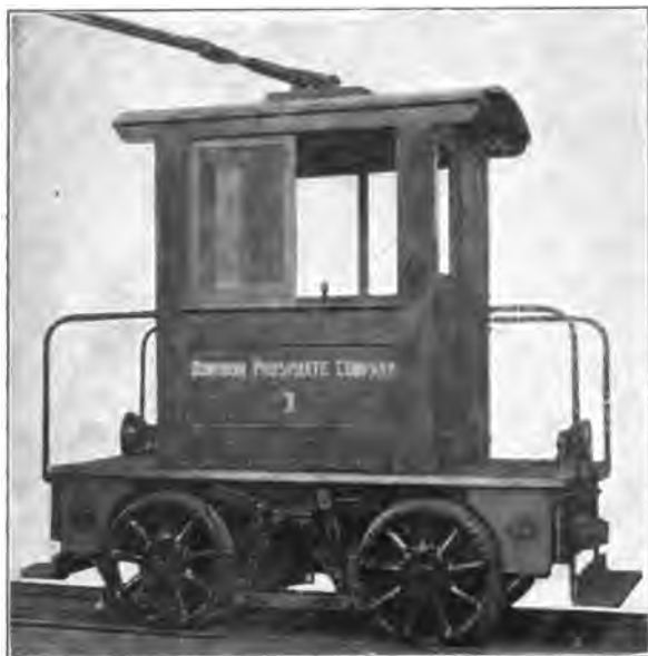
Fig. 4713. Baldwin-Westinghouse Electric Locomotive for the Dominion Phosphate Co. Weight, 12,000 lbs.; Diameter of Drivers, 30 in.; Wheel Base, 5 ft.; Drawbar Pull, Starting, 2,400 lbs.; Drawbar Pull, Running, 1,300 lbs.; No. of Motors, 2.
