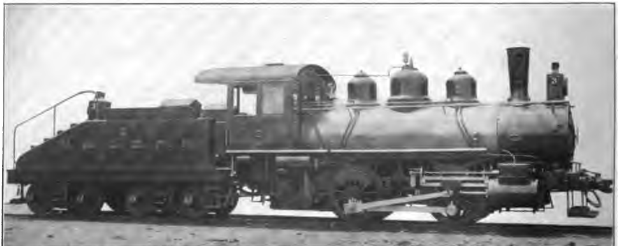
Fig. 4. Four-Wheel (0—4—0) Switching Locomotive. Built by the Baldwin Locomotive Works for the Wheeling & Lake Erie. Cylinders 17 in. x 24 in., Working Steam Pressure 175 lbs. per sq. in., Heating Surface 1,254 sq. ft., Diameter of Drivers 50 in., Weight on Drivers 93,110 lbs., Total Weight 93,110 lbs.
