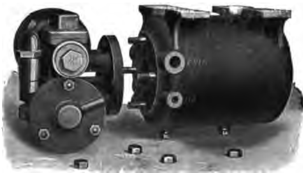
Distributing Valve and Double-Chamber Reservoir Showing Distributing Valve Disconnected
