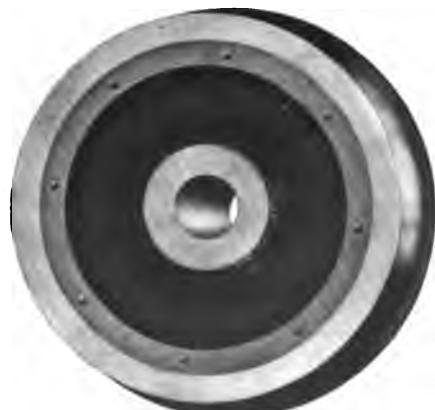
Figs. 4569-4570. Cast-steel Plate Center held by Shrinkage, Double Lip Retaining Rings and Rivets.
