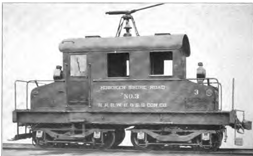
Fig. 4715. Baldwin-Westinghouse Electric Locomotive for the Hoboken Shore Road. Weight, 120,000 lbs.; Diameter of Drivers, 36 in.; Wheel Base, 19 ft.; Drawbar Pull, Starting, 24,000 lbs.; Drawbar Pull, Running, 14,500 lbs.; No. of Motors, 4.
