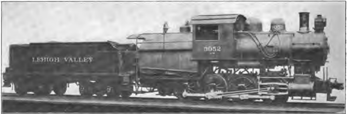
Fig. 20. Eight-Wheel (0-8-0) Switching Locomotive. Built by the Baldwin Locomotive Works for the Lehigh Valley. Cylinders 21 in. x 28 in., Working Steam Pressure 200 lbs. per sq. in., Heating Surface 2,248 sq. ft., Diameter of Drivers 55½ in., Weight on Drivers 172,450 lbs., Total Weight 172,450 lbs.
