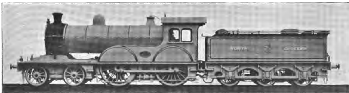
Fig. 4978. Eight-Wheel, Four-Coupled Locomotive. North Eastern Railway. Cylinders 19 in. x 26 in.; Total Heating Surface 1,527 sq. ft.; Diameter of Drivers 82 in.; Weight on Drivers, 79,960 lbs.; Total Weight 126,810 lbs.
