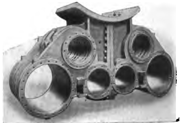
Fig. 2187. Cylinder Saddle for Baldwin Four-Cylinder Balanced Compound, Baldwin Locomotive Works.
