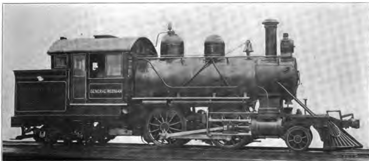
Fig. 29. Four-Coupled Double Ender (2—4—4) Locomotive. Built by the Baldwin Locomotive Works for the U. S. Government Sandy Hook Proving Grounds. Cylinders 15 in. x 22 in., Working Steam Pressure 160 lbs. per sq. in., Total Heating Surface 896 sq. ft., Diameter of Drivers 54 in., Weight on Drivers 58,420 lbs., Total Weight 111,940 lbs.
