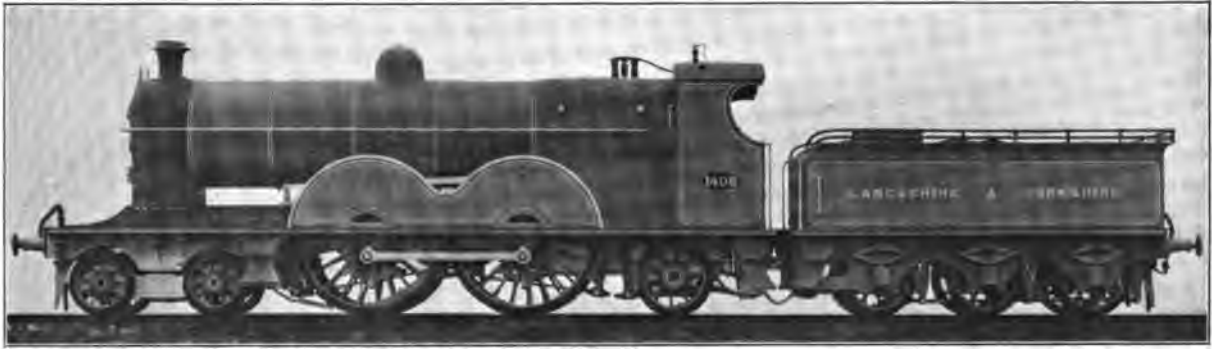
Fig. 4989. Ten-Wheel, Four-Coupled Locomotive. Lancashire & Yorkshire. Cylinders 19 in. x 26 in.; Working Steam Pressure 180 lbs. per sq. in.; Total Heating Surface 2,052.6 sq. ft.; Diameter of Drivers 87 in.; Weight on Drivers 78,400 lbs.; Total Weight 131,600 lbs.
