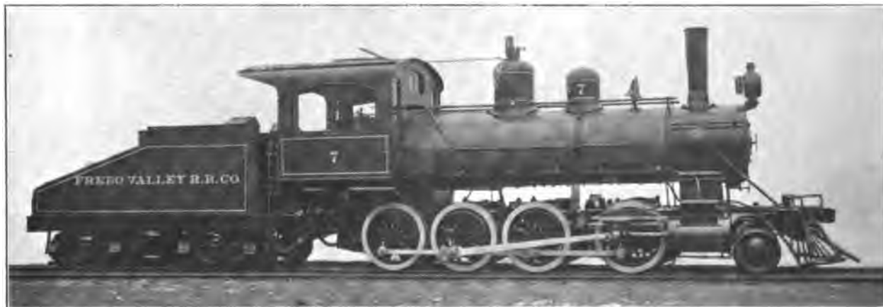
Fig. 40. Consolidation (2-8-0) Locomotive. Built by the Davenport Locomotive Works. Cylinders 16 in. x 24 in., Working Steam Pressure 160 lbs. per sq. in., Heating Surface 1,233 sq. ft., Diameter of Drivers 46 in., Weight on Drivers 82,700 lbs., Total Weight 92,500 lbs.
