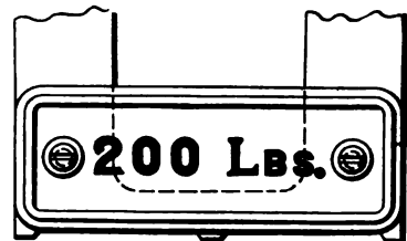
Figs. 237-238. Badge Plate for Boiler Pressure. Atlantic (4-4-2) Locomotive. P. R. R.
