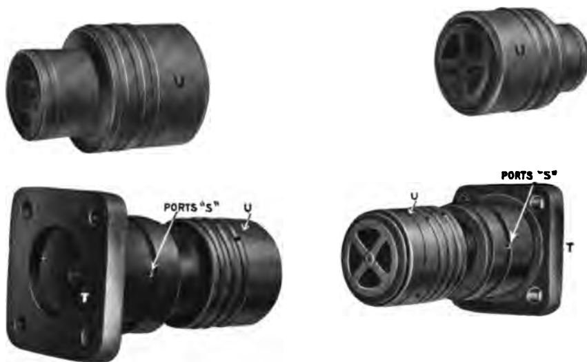
FIG. 12.—Construction of By-pass valves.
