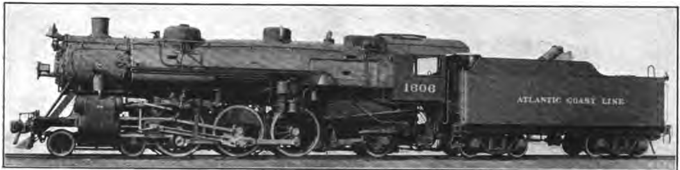
PACIFIC OR 4-6-2 TYPE LOCOMOTIVE FOR THE ATLANTIC COAST LINE. (BUILT BY THE BALDWIN LOCOMOTIVE WORKS.)
