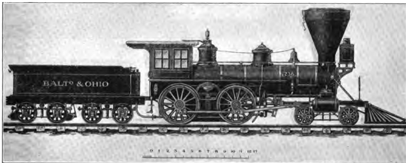
PASSENGER ENGINE BUILT FOR THE BALTIMORE & OHIO R. R. BY WM. MASON & CO. IN 1857
