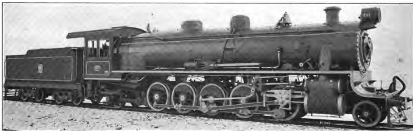
SANTE FE 2-10-2 TYPE LOCOMOTIVE FOR THE MANILA RAILROAD. AMERICAN LOCOMOTIVE COMPANY, BUILDERS.
