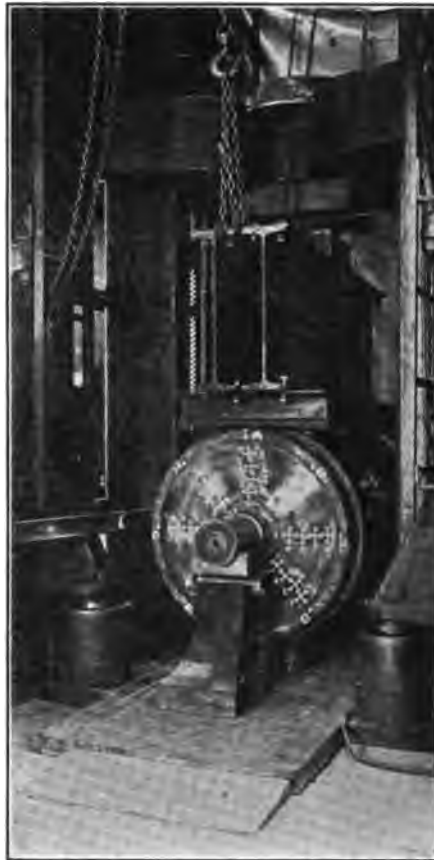
600,000-LB. TESTING MACHINE WITH PAIR OF WHEELS IN POSITION TO RECEIVE STATIC LOAD
