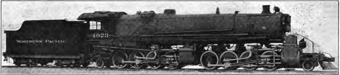
MALLET TYPE 2-8-8-2 LOCOMOTIVE FOR THE NORTHERN PACIFIC RAILWAY COMPANY. AMERICAN LOCOMOTIVE COMPANY, BUILDERS
