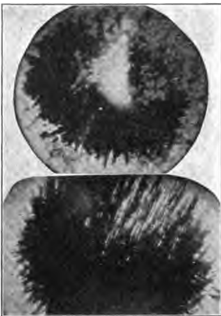
POWDER OF FILM UNDER MAGNETIC INFLUENCE—14 DIAMETERS
