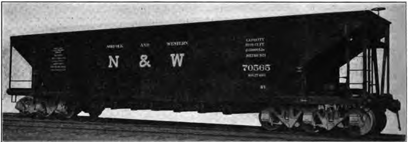
240,000 LBS. CAPACITY COAL CAR—NORFOLK & WESTERN RY.
