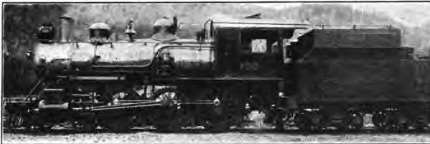
PACIFIC TYPE LOCOMOTIVE, SPOKANE INTERNATIONAL RAILWAY, WITH NICHOLSON THERMIC SYPHON.
