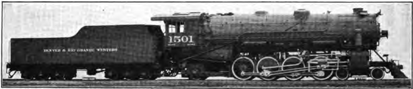
DENVER & RIO GRANDE RAILROAD MOUNTAIN TYPE LOCOMOTIVE. (BUILT BY THE AMERICAN LOCOMOTIVE CO.)
