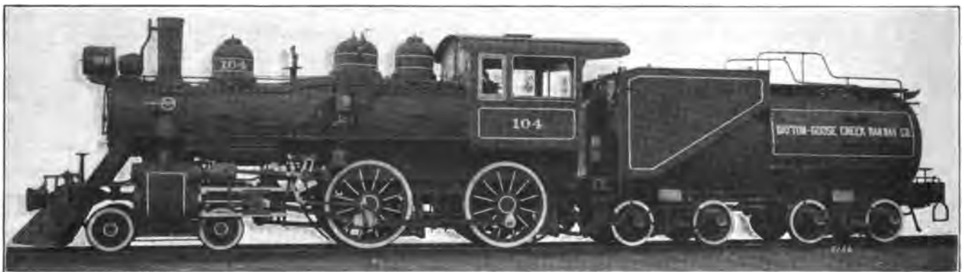
EIGHT-WHEEL TYPE 4-4-0 LOCOMOTIVE FOR THE DAYTON-GOOSE CREEK RAILWAY. BALDWIN LOCOMOTIVE WORKS, BUILDERS
