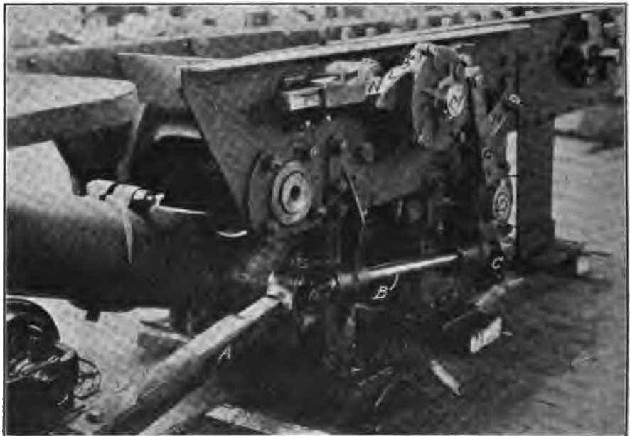
SIDE VIEW OF OPERATING MECHANISM OF CONVEYOR FEED OF ELVIN
