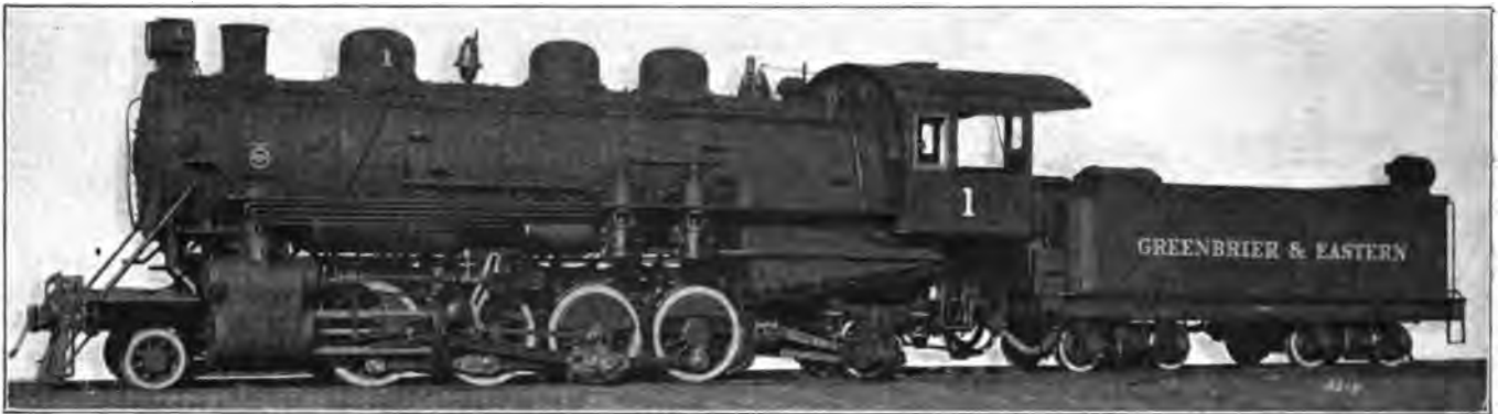
MIKADO TYPE 2-8-2 LOCOMOTIVE FOR THE GREENBRIER & EASTERN RAILROAD. BALDWIN LOCOMOTIVE WORKS, BUILDERS
