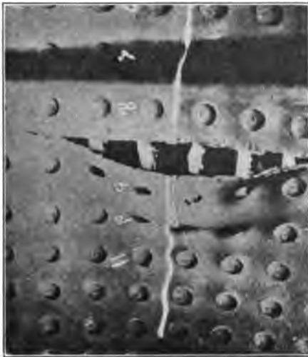
Fig. 2. Shows a crown-sheet failure, due to low water, which caused the serious injury of three persons. The autogenously welded seam between the crown sheet and combustion chamber failed. The line of demarcation showed that the water at the time of the accident was approximately 2 inches below the highest part of the crown sheet.
