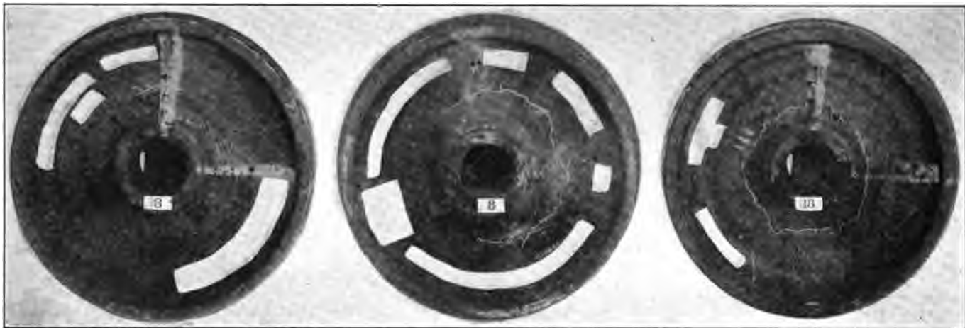
WHEELS FAILING UNDER THERMAL TESTS SHOWING CRACKS
