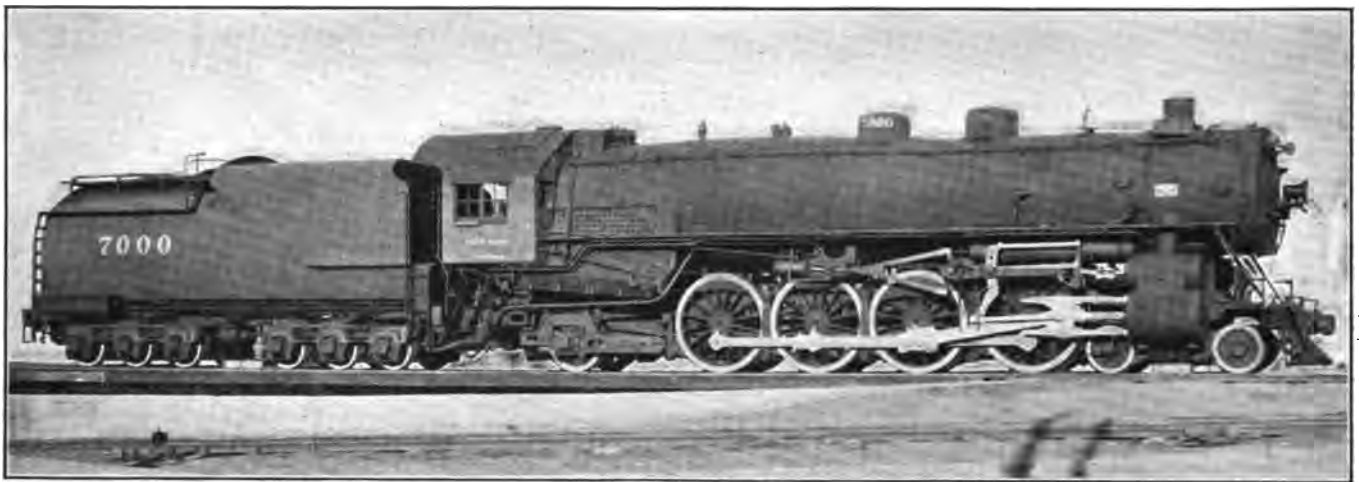
MOUNTAIN TYPE 4-8-2 PASSENGER LOCOMOTIVE FOR THE UNION PACIFIC RAILROAD AMERICAN LOCOMOTIVE COMPANY, BUILDERS
