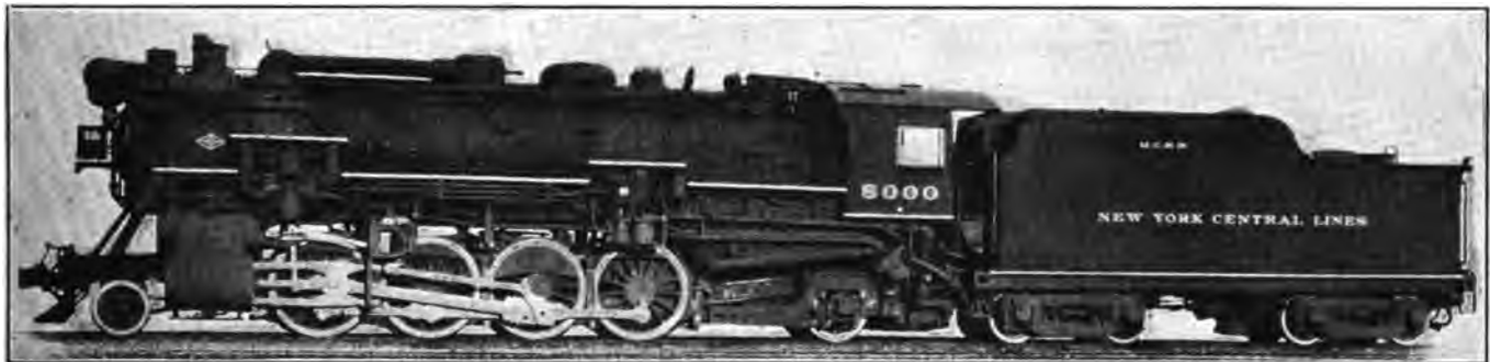
MICHIGAN CENTRAL LOCOMOTIVE OF THE MIKADO (2-8-2) TYPE—BUILT BY LIMA LOCOMOTIVE WORKS, INC.
