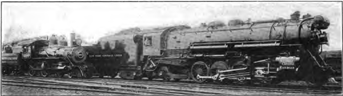
MIKADO 2-8-2 TYPE LOCOMOTIVE NO. 8000, OF THE MICHIGAN CENTRAL, SAID TO BE THE MOST POWERFUL OF ITS WEIGHT AND ON THE LEFT, ENGINE NO. 8977, FORMERLY 248, STILL RUNNING AFTER A SERVICE OF FORTY YEARS
