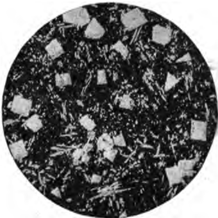
FIG. 1. GENUINE BABBITT. ANALYSIS IDENTICAL WITH FIG. 2. TIN 88.9, ANTIMONY 7.4, COPPER 3.7
