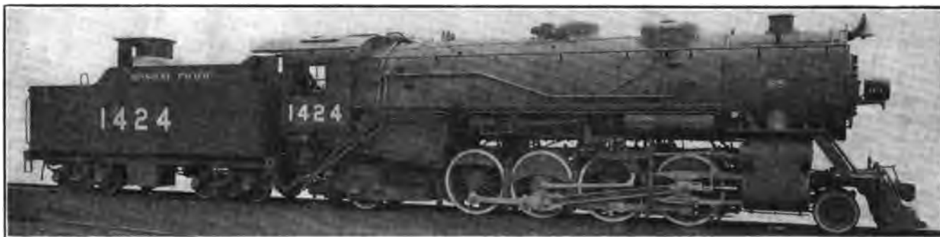
MIKADO 2-8-2 TYPE LOCOMOTIVE FOR THE MISSOURI PACIFIC RAILWAY AMERICAN LOCOMOTIVE COMPANY, BUILDERS
