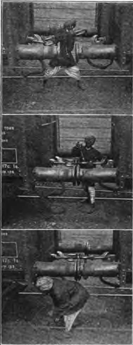
FIG. 3. SHOWING NATIVE SWITCHMAN ATTACHING SCREW COUPLING ONTO HOOK, TIGHTENING COUPLING, AND LEAVING VEHICLES
