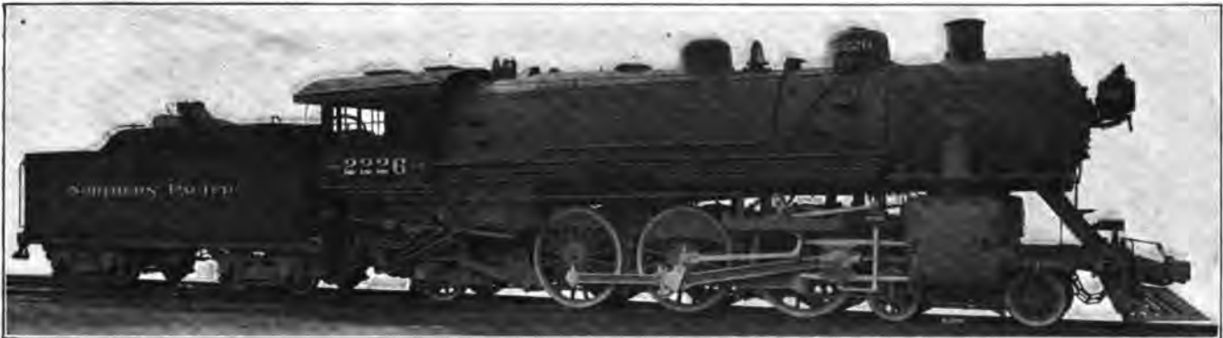
PACIFIC TYPE 4-6-2 LOCOMOTIVE FOR THE NORTHERN PACIFIC RAILWAY COMPANY. AMERICAN LOCOMOTIVE COMPANY, BUILDERS
