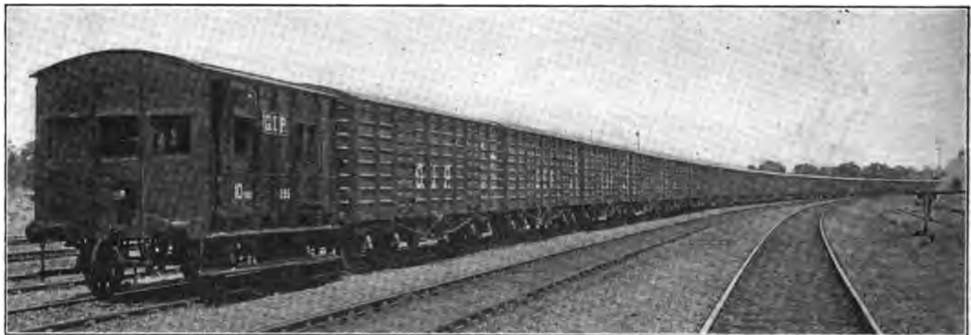
FIG. 2. 2,000 TON TRAIN, VIEW FROM REAR TO SHOW 10-TON CABOOSE. TRAIN THROUGHOUT FITTED WITH CONTINUOUS BRAKES
