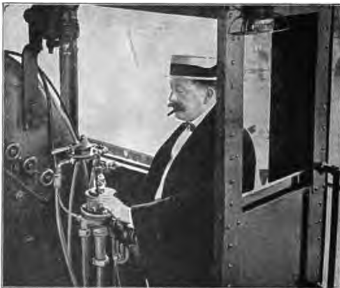
THIS ILLUSTRATION SHOWS LOCATION OF COMBINED RELEASE AND RETAINING VALVE JUST ABOVE THE ENGINEER'S AUTOMATIC BRAKE VALVE.
