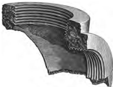
FIG. 5. — A BROKEN FITTING.
