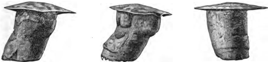
SOME DEFECTIVE RIVETS.
