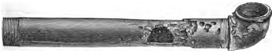
CORRODED BRASS PIPE FROM THE INTERIOR OF A BOILER.
