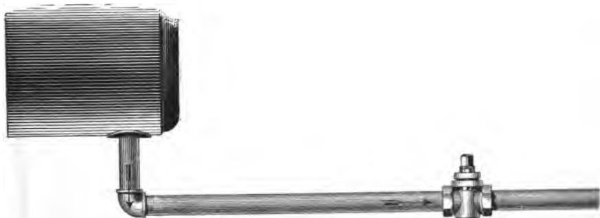
FIG. 3. — ILLUSTRATING THE "WATER RAM" IN BLOW-OFF PIPES.
