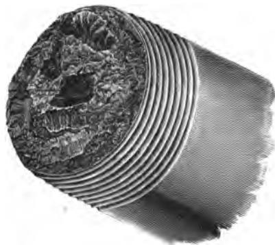
FIG. 3. — A FEED-PIPE CHOKED WITH A STONE-LIKE SCALE.
