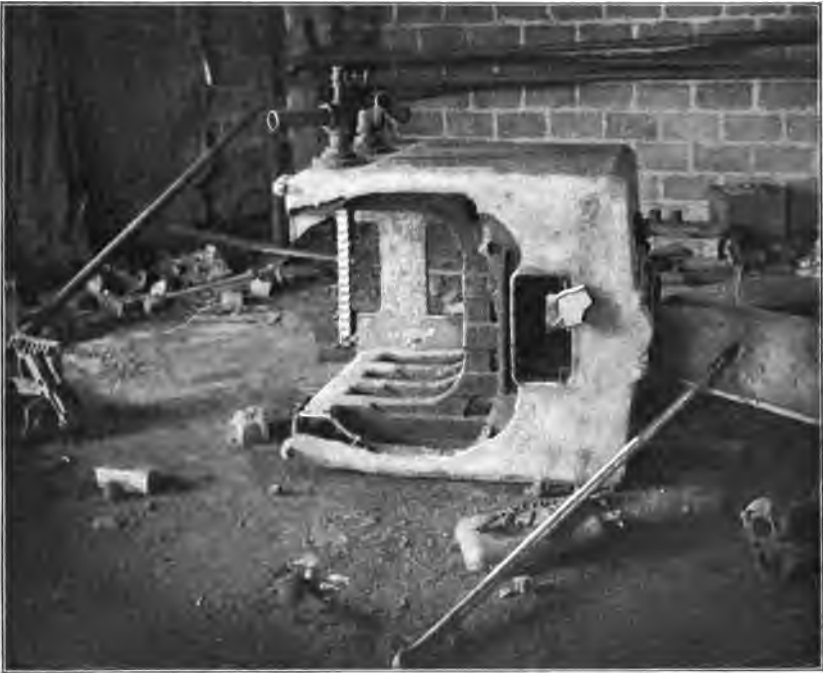
· EXPLODED HEATING BOILER.
