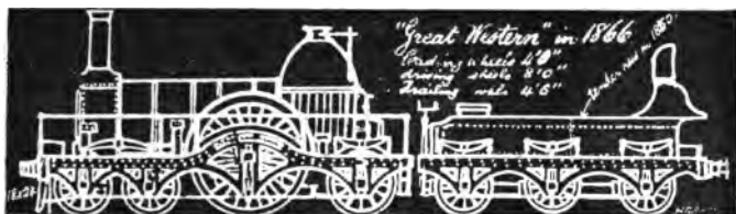
FIG 39.—THE ORIGINAL "GREAT WESTERN" AS REBUILT WITH TWO PAIRS OF LEADING WHEELS
