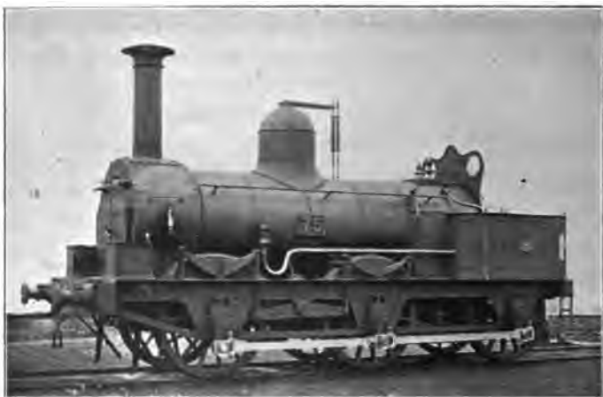
FIG. 81.—SIX-COUPLED MINERAL ENGINE, TAFF VALE R.WY., BUILT 1860
