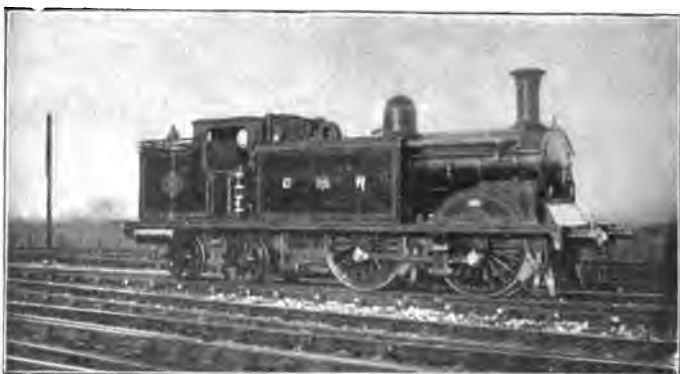
FIG 125.—MOUNTOSH'S 5FT. 9IN. CONDENSING TANK ENGINE, CALEDONIAN RAILWAY
