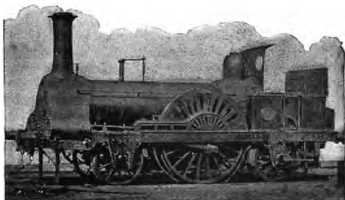
FIG. 62.—ONE OF J. V. GOOCH'S "SINGLE" TANK ENGINES, EASTERN COUNTIES RAILWAY
