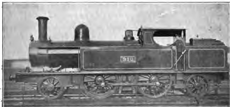
FIG. 146.—LONDON AND NORTH-WESTERN RAILWAY, NEW TYPE OF 8-WHEEL TANK ENGINE
