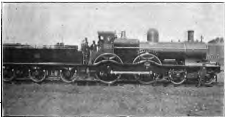
Fig. 134. — "BARRINGTON," NEW TYPE OF 4-COUPLED ENGINE, GREAT WESTERN RAILWAY
