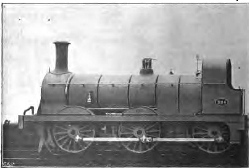
FIG. 110.—STANDARD GOODS ENGINE, SOUTH EASTERN RAILWAY
