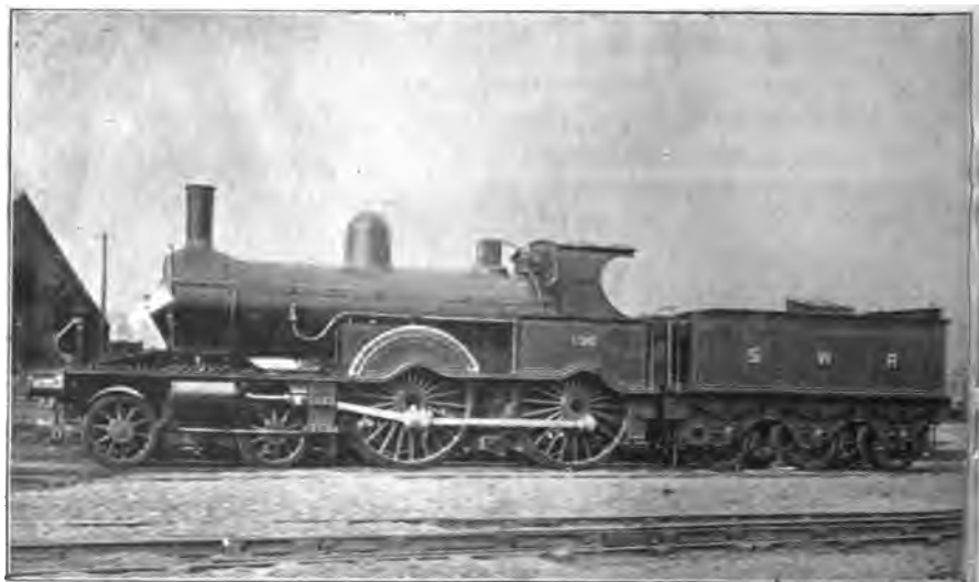
FIG. 114.—A "WINDCUTTER" LOCOMOTIVE ENGINE, "No. 136," L. & S.W.R., FITTED WITH A CONVEX SMOKE-BOX DOOR
