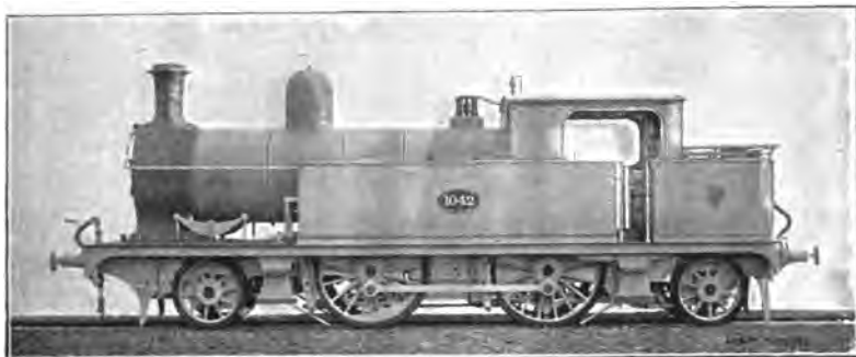
FIG. 113.—STANDARD 8 WHEEL PASSENGER TANK ENGINE, L. & Y.R.
