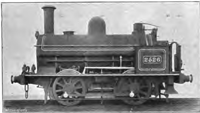
FIG. 118.—FOUR-WHEELS-COUPLED, SADDLE TANK ENGINE, LONDON AND NORTH WESTERN RAILWAY
