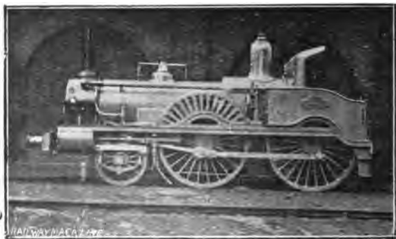
FIG. 90.—"PYTHON," A 7ft. 1in. COUPLED EXPRESS ENGINE, LONDON AND SOUTH WESTERN RAILWAY
