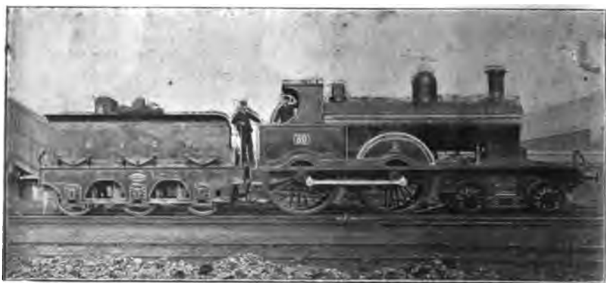
FIG. 148.—"JUBILEE," 4-WHEELS COUPLED COMPOUND LOCOMOTIVE, BELFAST AND NORTHERN COUNTIES RAILWAY
