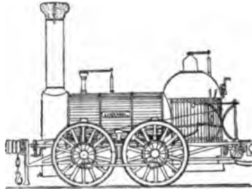
Fig. 96. —Bury's first Inside-cylinder Engine, "Liverpool," completed March, 1831 ; sent to America.
