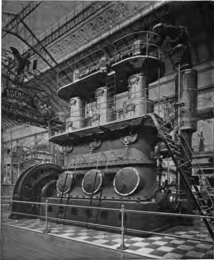
FIG. 12. A 3,000 H.P. TRIPLE EXPANSION CENTRAL VALVE ELECTRICAL ENGINE
