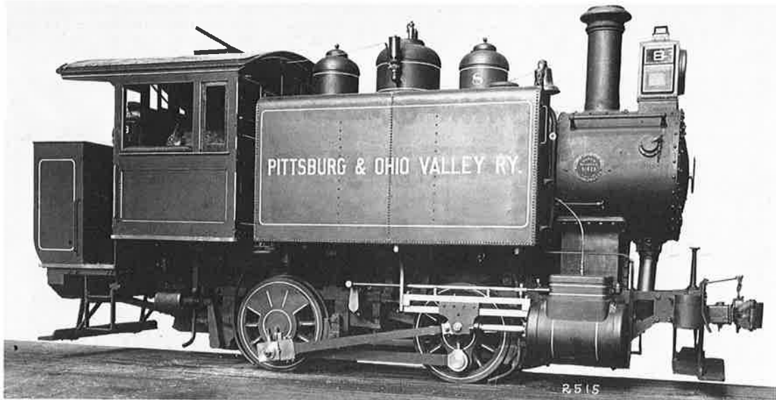
The Pittsburgh and Ohio Valley is the only railroad entirely on an island. No 8 was built in 1931 to switch cars on sharp industrial curves.
