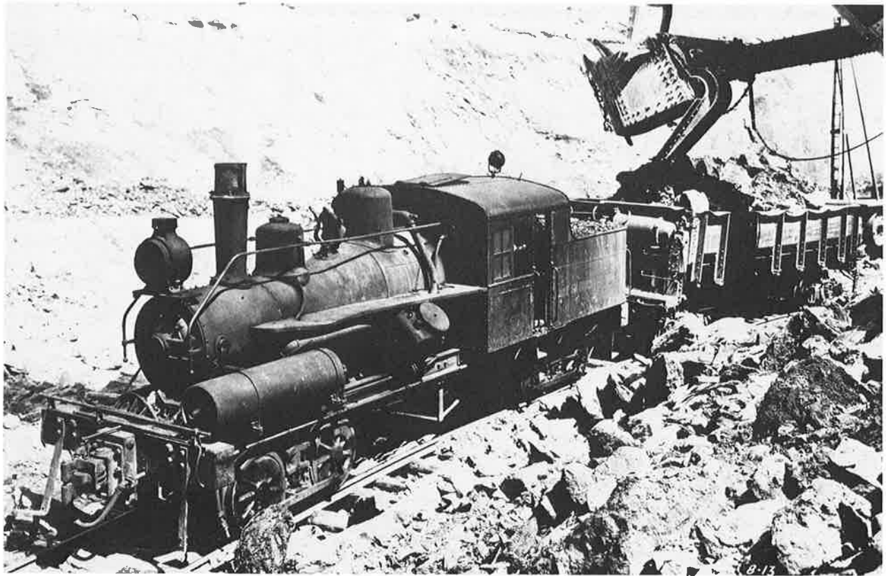
Beginning in the late 1920s and continuing until the mid 1930s a relatively large number of Heisler and Shay geared locomotives were sold to strip mining operations, particularly in Pennsylvania, Ohio, and Indiana. This is Harleigh Brookwood Coal Co. No. 64, Heisler c.n. 1517 at Frackville at an anthracite strip mine. Walter Casler
