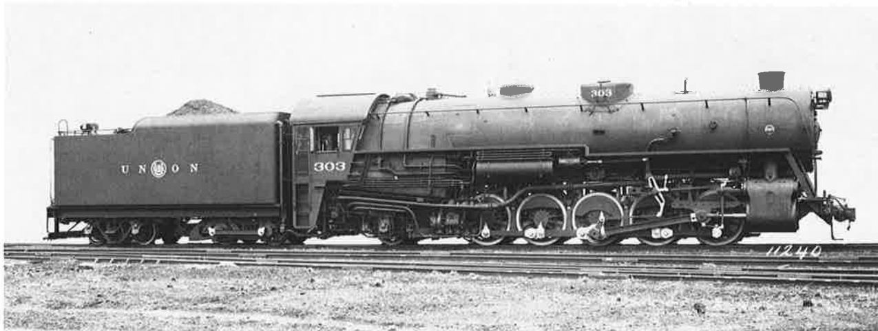
No. 303 was one of 9 giant transfer locomotives built in 1936 and 1937 to move ore trains brought down by the B&LE to North Bessemer. They replaced 2-8-0s which could only take part of a B&LE ore train. These 0-10-2s handled the full train on its slow run to the mills.
