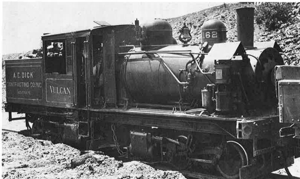
In 1932 the Vulcan Iron Works at Wilkes Barre, which had long been building industrial steam and gasoline locomotives, took an idea originated by the Davenport Locomotive Co. back around 1906 and came out with its Duplex. The 0-4-4-0 had cylinders mounted on the engine truck. Unfortunately, the swivelling steam pipe joints could not be kept tight. Vulcan built six in 1932 and 1933. All went to anthracite coal strip mine operations, A. E. Dick at Audenreid and Parsons bought 3, Hill and Suender Company at Natalie bought two, and Haddock Mining at Silver Brook bought one. As with Heisler geared engines sold at the same time to strip miners, their operating life was short, and none were still in operation by 1940. This is #4162.
