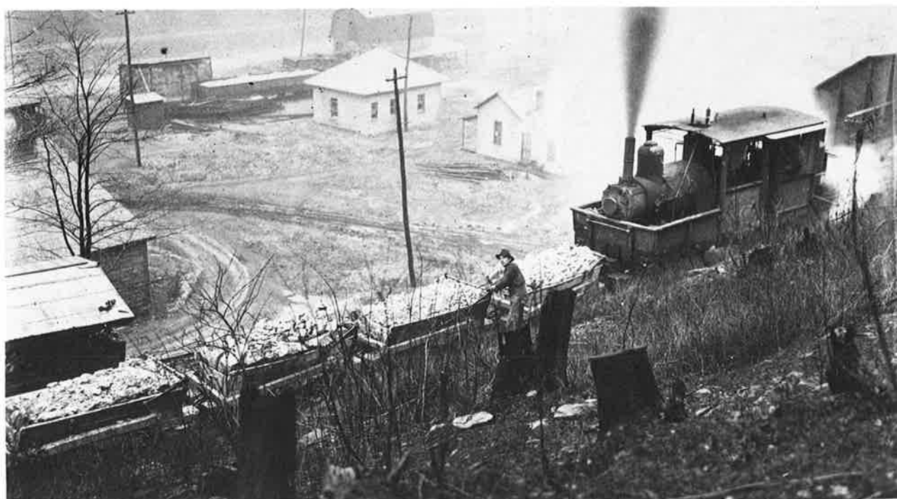
Elk Fire Brick Company's clay train drops down into Drury's Run, just west of Renovo in 1920. The clay cars are eight wheeled whereas cars used in the 1900-1910 had only four.
