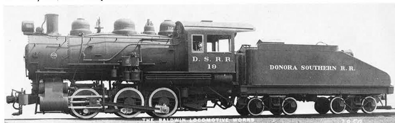
Donora Southern No. 19 built by Baldwin in 1921 to serve U.S. Steel Company's mill at Donora. Although earlier D.S. switchers had been superheated, this engine was not. Its narrow firebox and Stephenson valve gear are also throwbacks to the turn of the century.
