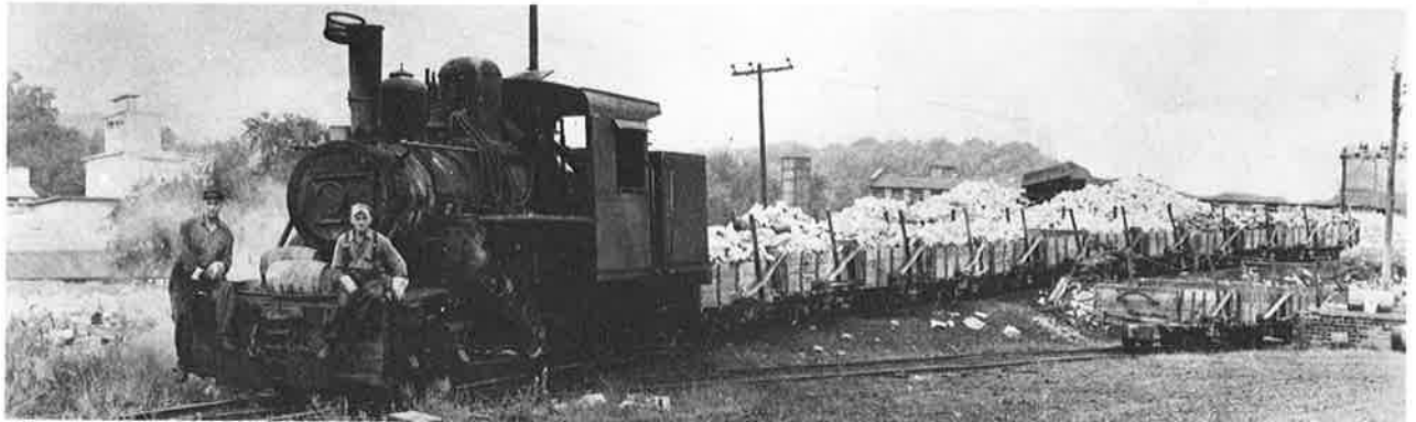
The narrow gauge Climax No. 2 of General Refractories Co. at Sproul, switches a string of mine cars at the brick plant probably during the early 1930s. They continued to use their railroad until about 1950. Walter Casler
