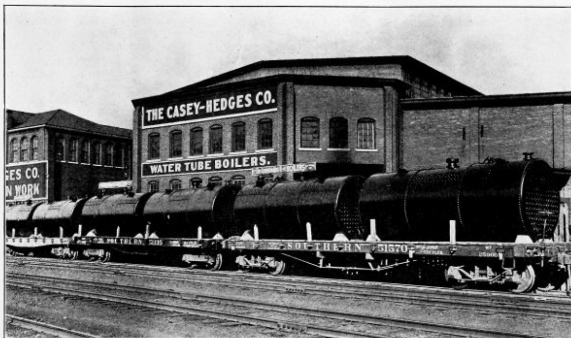
SHIPMENT OF HORIZONTAL RETURN TUBULAR BOILERS TO BE EQUIPPED WITH STEEL DUTCH OVEN SETTINGS.
