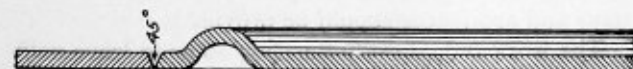
FIG. 1.—PARTIAL VIEW OF PATCH ABOUT TO BE WELDED TO THE SIDE SHEET.
