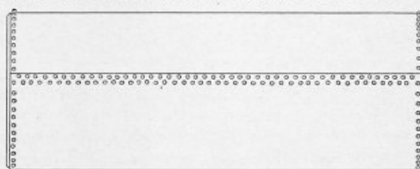
FIG. 5.—TWO SHEET CONSTRUCTION.
