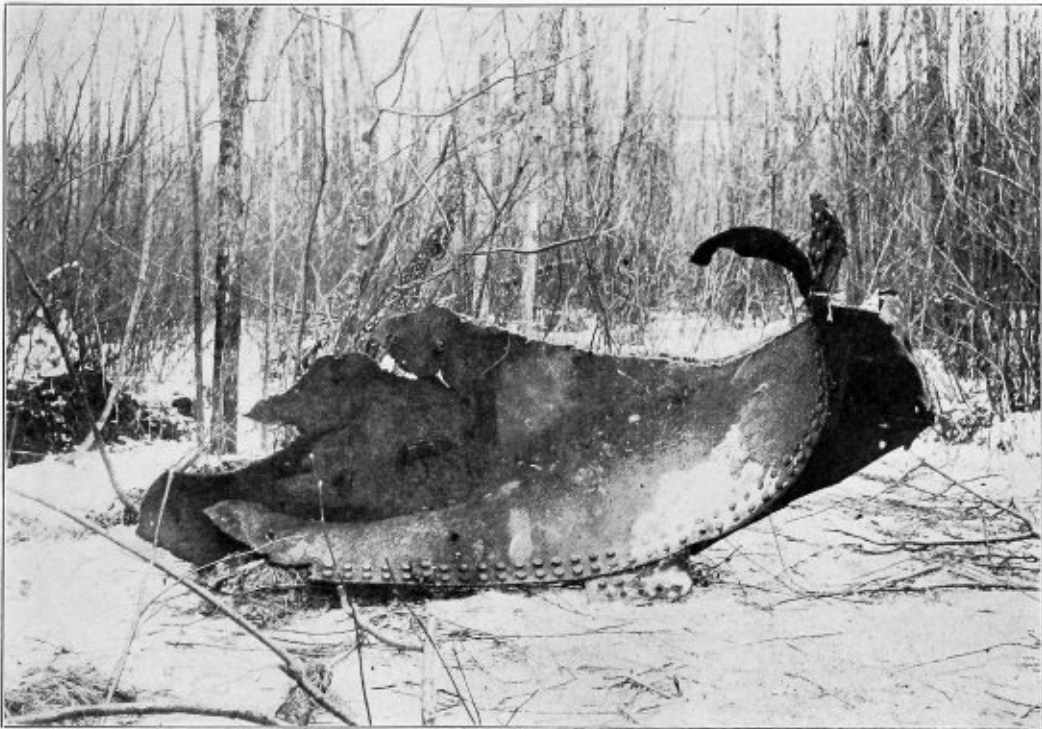
FIG. 1—PORTION OF BOILER SHELL, WEIGHING ABOUT 500 POUNDS, BLOWN 500 FEET, CUTTING OFF THREE TREES IN ITS PASSAGE, ONE OF WHICH WAS 8 INCHES IN DIAMETER.
