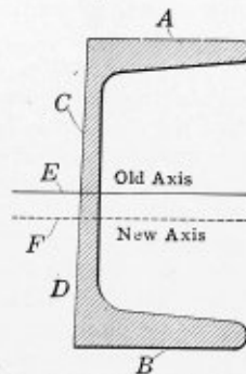
FIG. 2.—SHIFTING OF NEUTRAL AXIS
