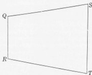
FIG. 6.—TAPER SHEET INCORRECTLY LAID OUT
