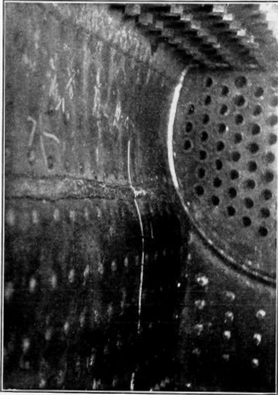
FIG. 2.—ELECTRICALLY WELDED FIRE-BOX SEAM
