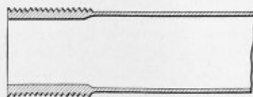
Fig. 13 Internal and External Upset Methods of Upsetting Tubes
