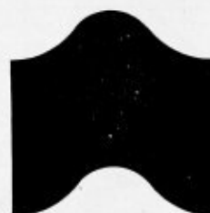
DEVELOPMENT OF OBLIQUE CYLINDER SHEET
