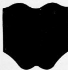
DEVELOPMENT OF SHEET FOR SLANTING TEE
