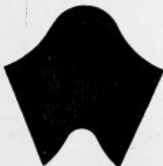
DEVELOPMENT OF OBLIQUE CONE SHEET
