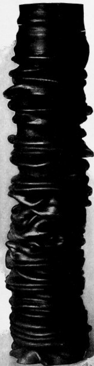
Fig. 4.—Shelby Hot-Finished Seamless Steel Boiler Tube, After Being Crushed Together From the Ends
