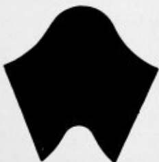
DEVELOPMENT OF OBLIQUE CONE SHEET
