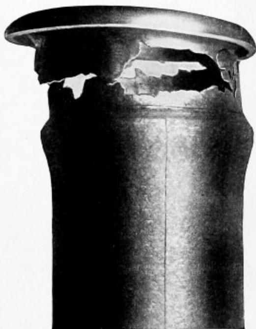
Fig. 2.—The Rolling and Beading Test (Note that the material wears away evenly when rolled to destruction before the bead cracks)
