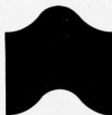
DEVELOPMENT OF OBLIQUE CYLINDER SHEET
