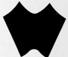
DEVELOPMENT OF TAPERING ARM OF Y-CONNECTION
