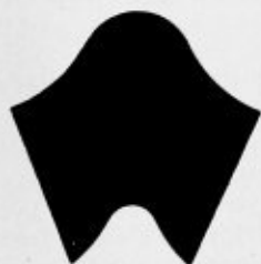
DEVELOPMENT OF OBLIQUE CONE SHEET
