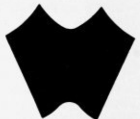
DEVELOPMENT OF TAPERING ARM OF Y-CONNECTION
