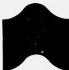
DEVELOPMENT OF OBLIQUE CYLINDER SHEET
