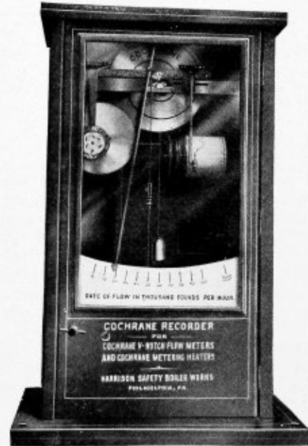
Recording Meter for Measuring Flow of Boiler Feed Water
