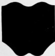
DEVELOPMENT OF SHEET FOR SLANTING TEE
