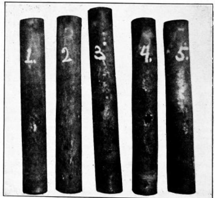
Fig. 18.—Tubes Heated and Split with Acetylene Gas
