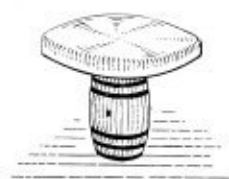
Fig. 2 - Head to be Drilled
