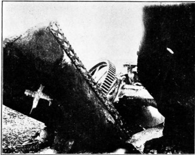
Fig. 13.—Munoz Boiler After Explosion
