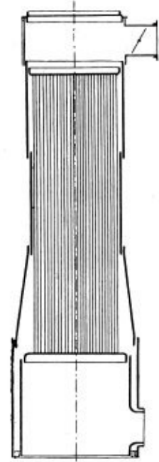
Fig. 6.—Vertical Boiler with Conical Course
