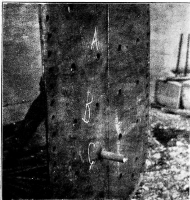
Fig. 10.—A Stripped Stay in the Plate
