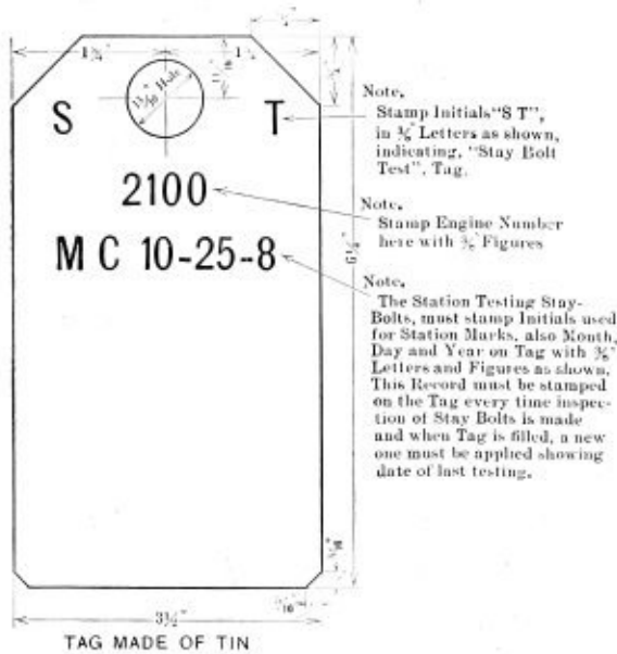
Fig. 7.—Metal Tag Showing Date of Staybolt Test
