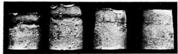
Sample of Tubes Taken from No. 16 Locomotive Boiler after Three Years' Service. This Boiler Was Equipped with Both Steel and Copper Ferrules, the Tubes Shown on the Left with Saw Marks Were Equipped with Copper Ferrules, and the Two without Saw Marks with Double Annealed Steel Ferrules. The Tubes Equipped with Steel Ferrules Showed Practically No Deterioration, While the Tubes Equipped with Copper Ferrules Showed Considerable Deterioration
