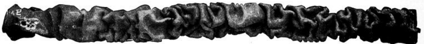
Fig. 2.—Eighteen-Foot Length of 5 3/16-Inch Steel Casing Crumpled to Length of 6 Feet Without Fracturing
