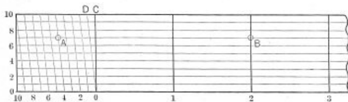
Fig. 1.—John Finds 2.47 Inches on a Steel Square
