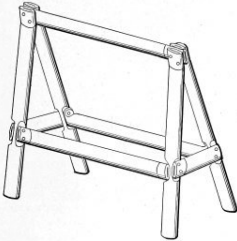
Fig. 1.—Work Horse Made from Old Boiler Tubes
