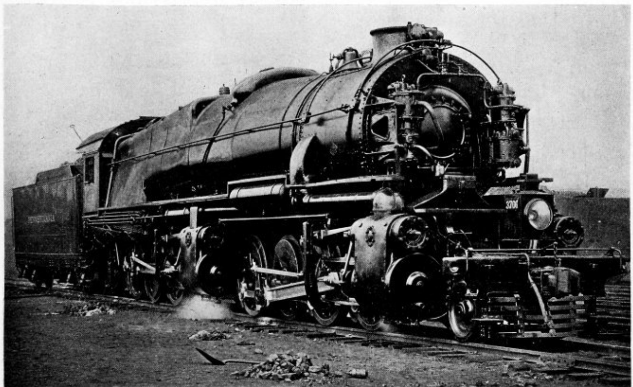
Fig. 1.—Heavy Freight Locomotive of the Mallet Type, Built by the Pennsylvania Railroad
