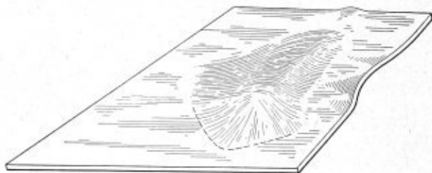
Fig. 1.—Sheet Buckled in the Middle
