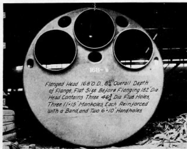
Fig. 2.—Large One-Piece Marine Boiler Head
