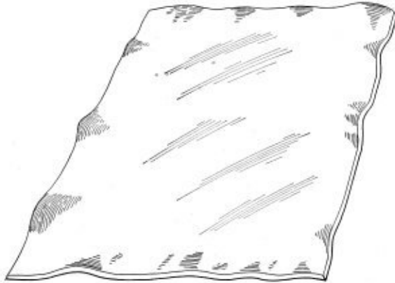
Fig. 2.—Edges of Plate Warped
