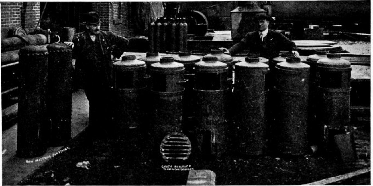
Fig. 2.—Completed Coal Stoves. Raw Material, in Shape of Discarded Air Tanks, Shown at the Left
