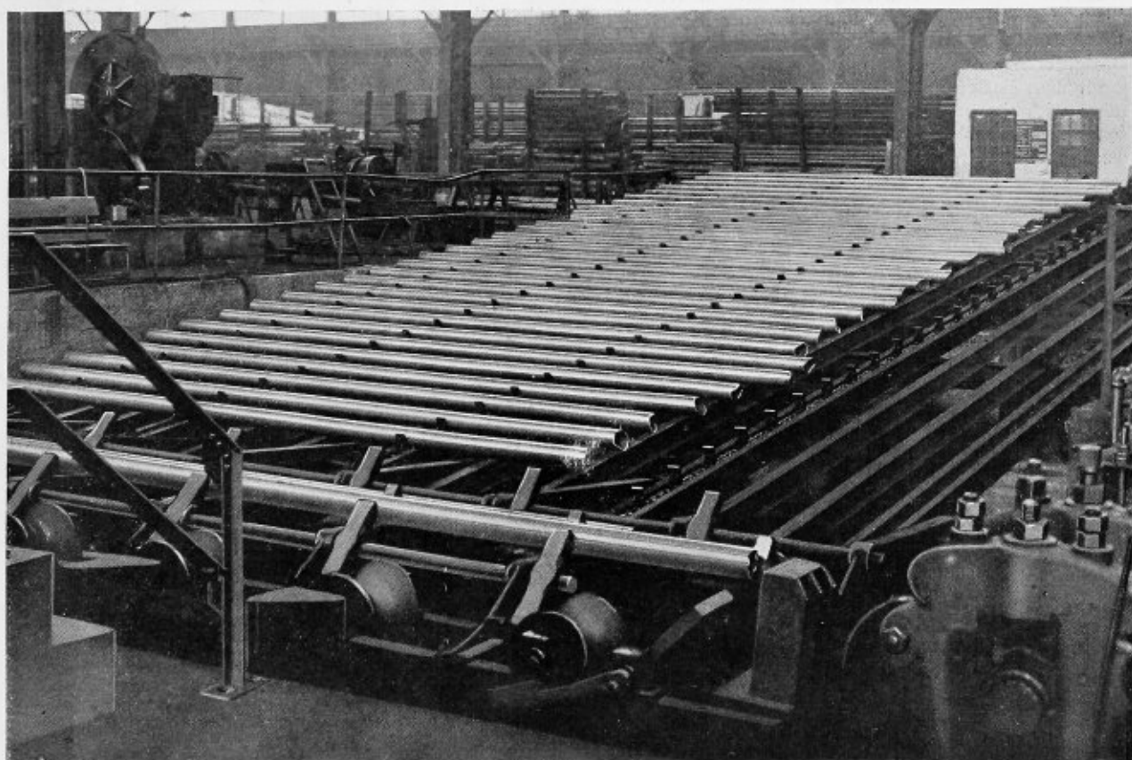
Cooling Table Receiving Tubes from Sizing Rolls
