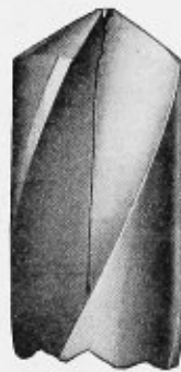
Fig. 9.—Split at Axis from Incorrect Grinding
