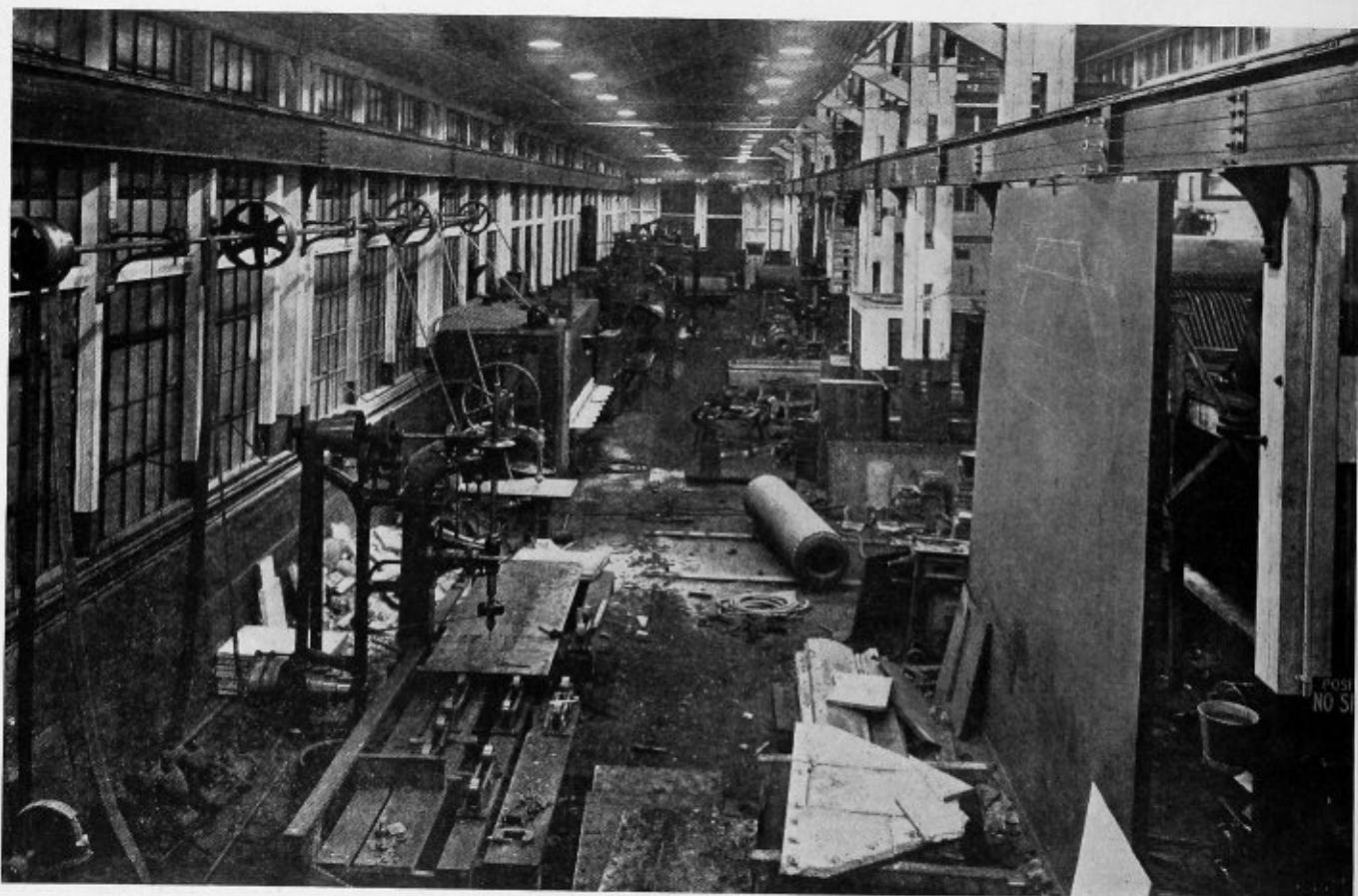
Fig. 10.—General View of West Bay Showing Drum Fabrication Facilities and Test Pit
