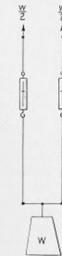
Fig. 5.—Angularity becomes zero when spring balances are parallel and in a vertical position
