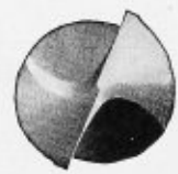
Figs. 11 and 12.—Correct and Incorrect Grinding of Drill Webs
