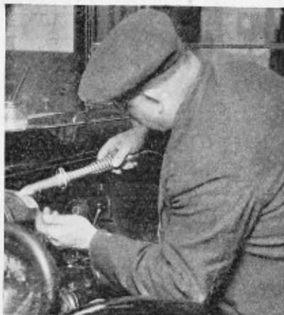
A Special Feature of the Electric Soldering Iron Is Its Flexible Handle
