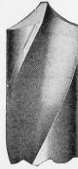
Fig. 10.—Thin and Weak Cutting Edges
