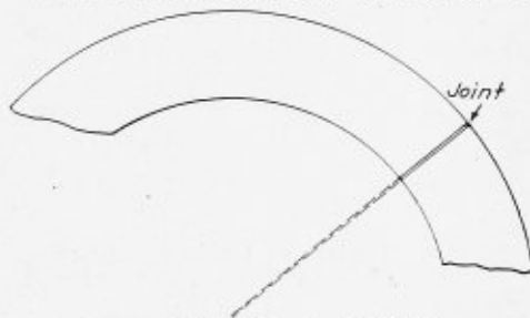
Fig. 1.—Perfect Joint in Thick Plates
