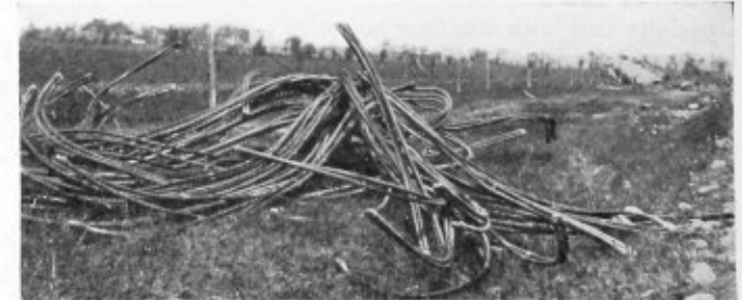
Fig. 5.—Superheater Header and Units 600 Feet from Point of Explosion
