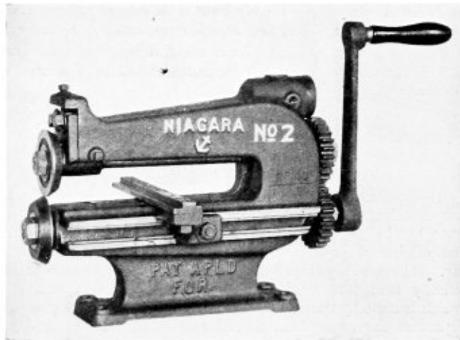
The Gage Is Set by Turning a Nut on the Gage Block.
