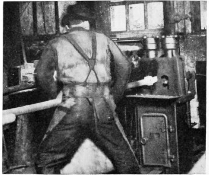
Fig. 6.—Tubes Are Heated to the Welding Point and Then Welded and Swedged on the Double Pneumatic Hammer Shown
