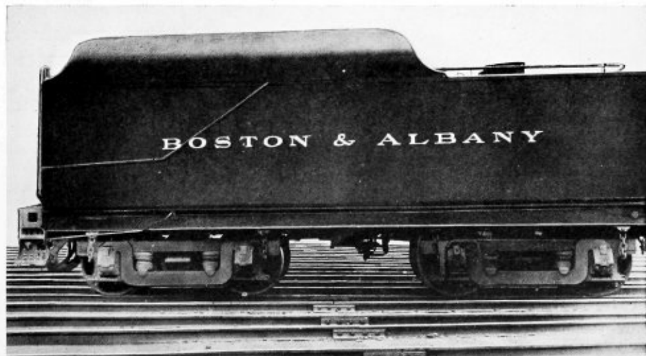
Fig. 5.—Eight Thousand Gallon All Welded Locomotive Tender Tank.
