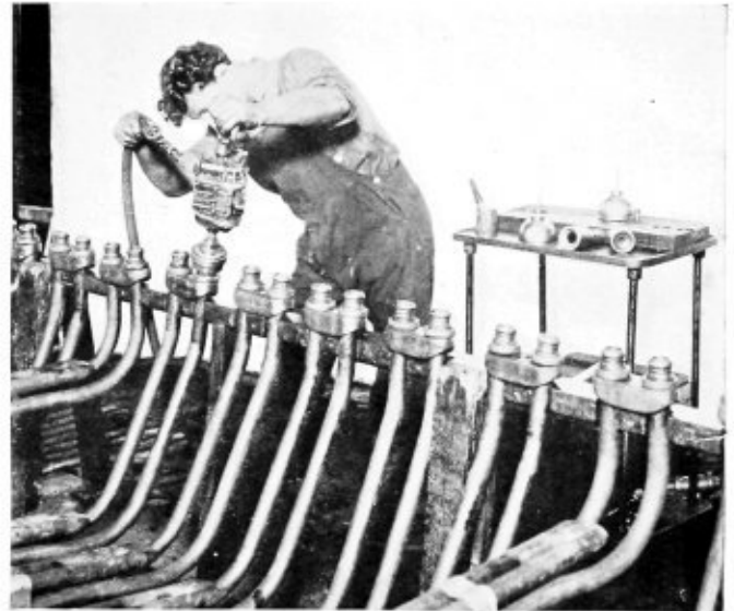
Fig. 6.—Grinding the Ball Ends on Superheater Units
