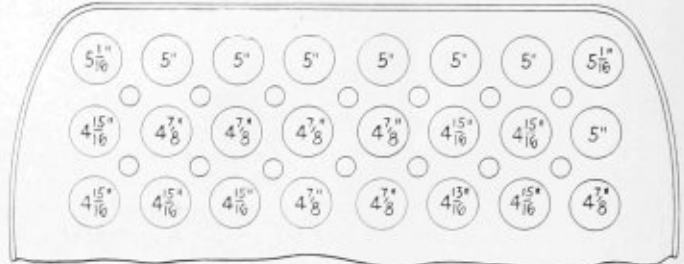
Fig. 10.—Tube Plate in Service Four Years and Seven Months
