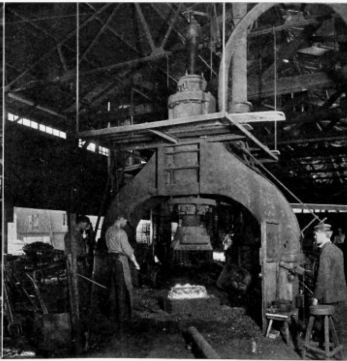
Fig. 2.—"Shingling" a Bloom Under a 3-ton Hammer
