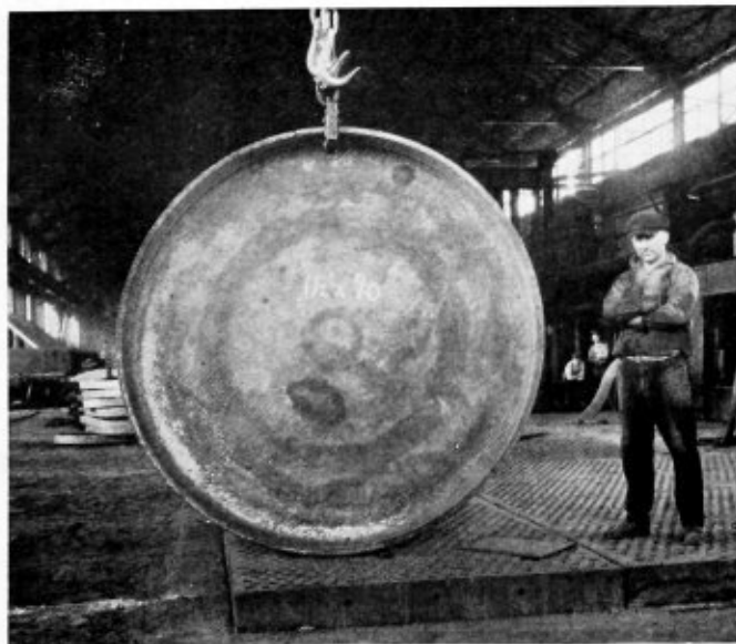
Fig. 3.—Ninety-Inch Ladle Bottom, Weighing 3,471 Pounds, Having 5-Inch Straight Flange
