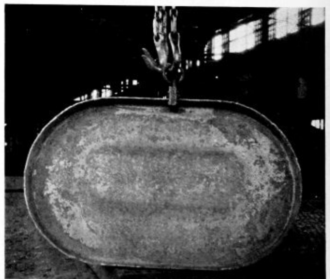
Fig. 6.—Tank Bottom Made on Sectional Flanger; Flange Is 76 Inches by 49 Inches by 6 Inches and Countersink Is 53 Inches by 22 Inches by 1\frac{1}{4} Inches
