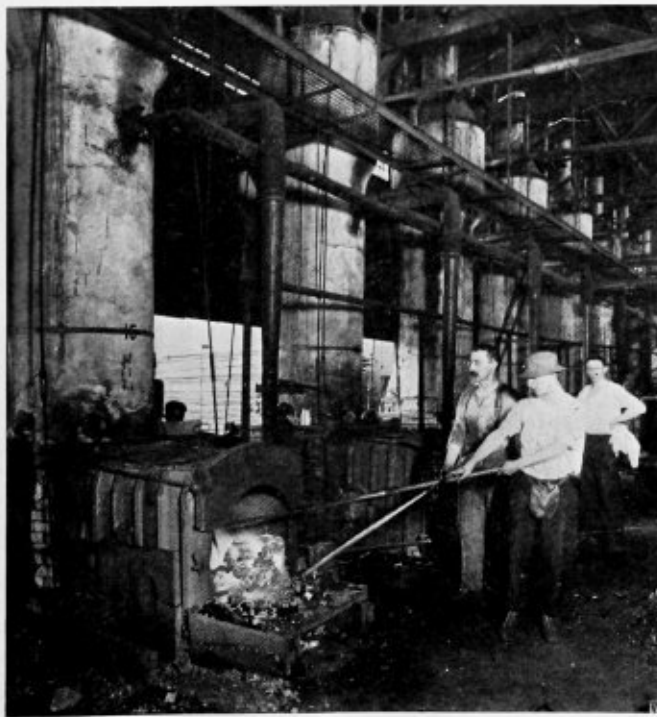
Fig. 1.—"Knobbling" a 300 Pound Charge in the Forge
