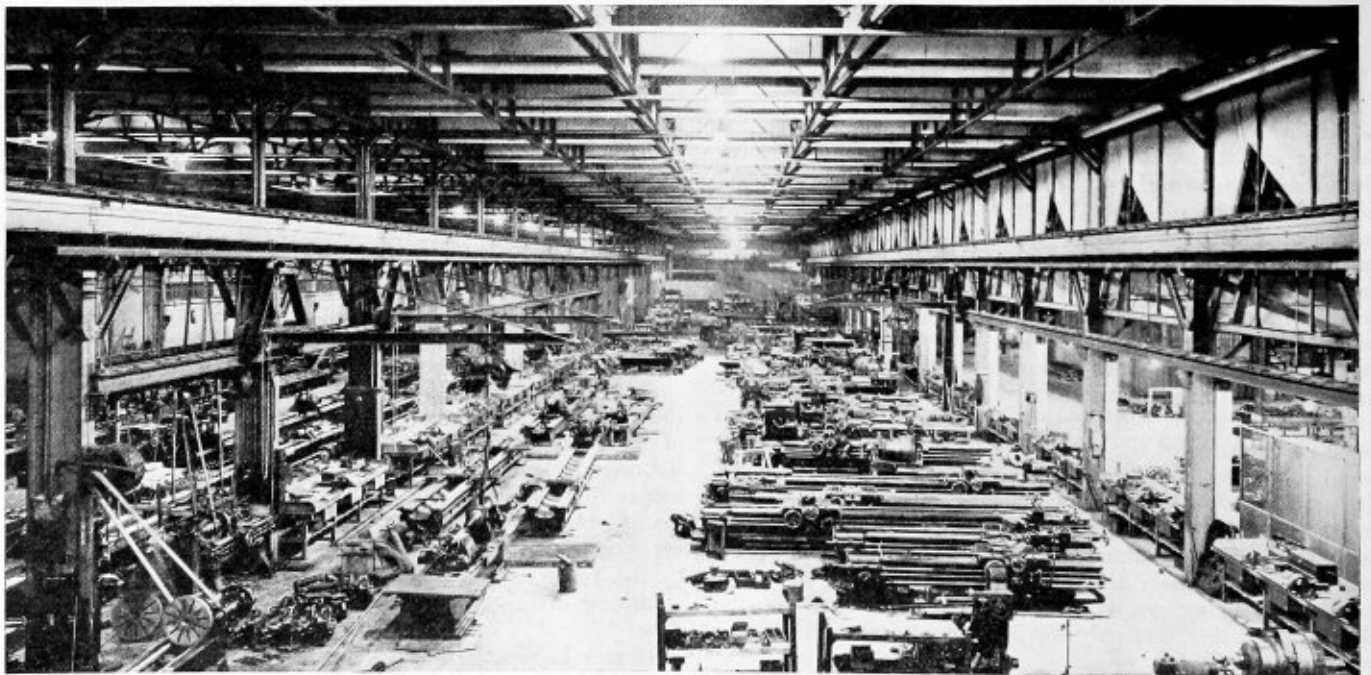
Fig. 4.—Mercury Vapor Lamps, Spaced 20 Feet Apart Are Used to Illuminate This Plant
