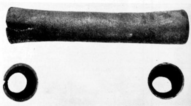
Fig. 8.—Effect of Expanding Tube When Passing Through the "Red Short" Temperature Range. Right End of Tube Expanded Correctly at Proper Temperature
