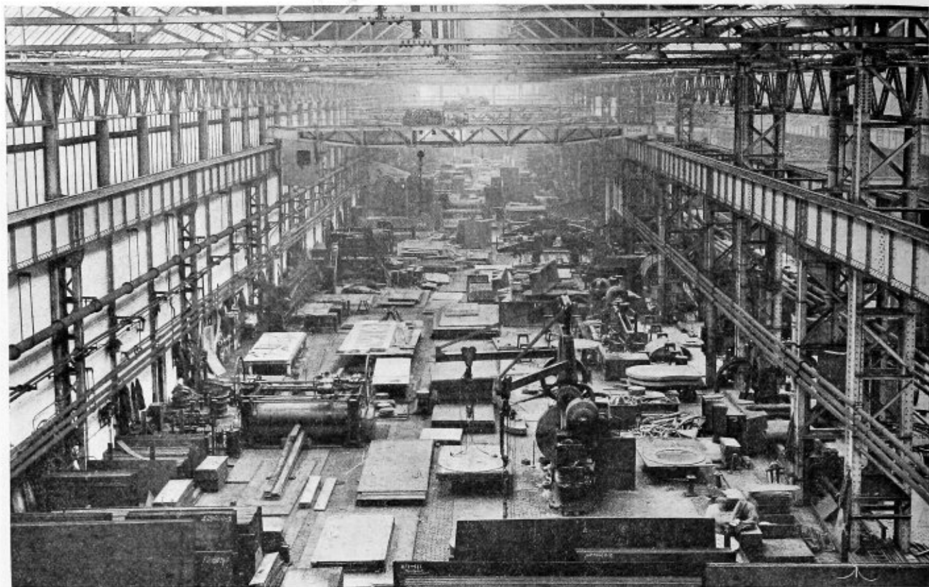
Fig 2—Eastern Section of North Bay Where Plates Are Laid Out, Drilled, Flanged and the Like
