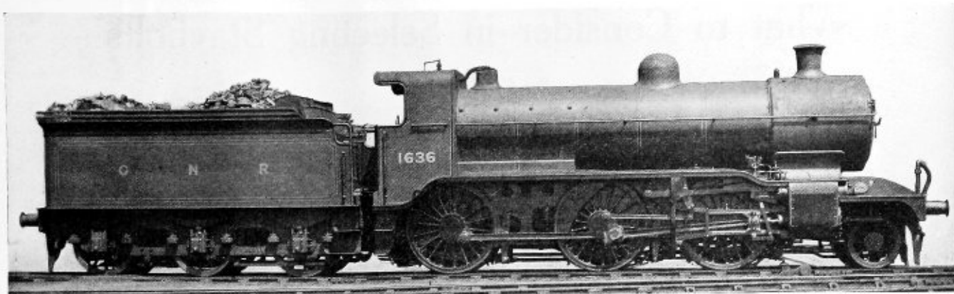
Fig. 1.—Type of Great Northern Railway 2-6-0 Express Locomotive Equipped with Exhaust Steam Injector
