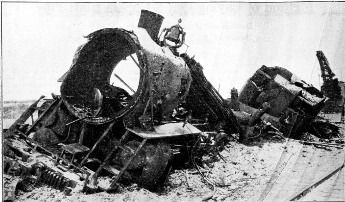
Fig. 1.—Results of a Low Water Explosion in Which the Water was Ten Inches Below the Top of the Crown Sheet at the Time of the Accident
