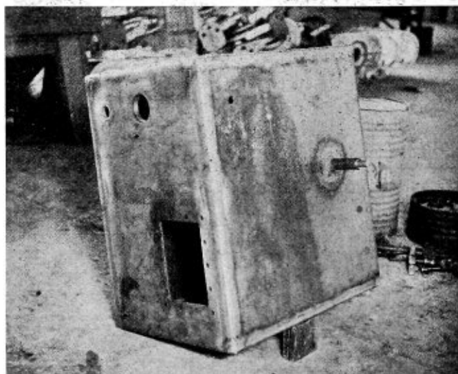
Fig. 7.—All Seams on This Tank Are Butt Welded
