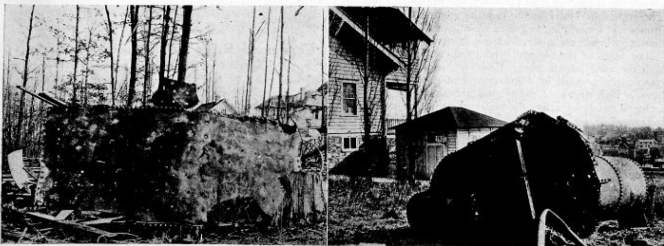
Fig. 2.—Crown Sheet of Boiler and Firebox and Barrel Near Scene of Disaster
