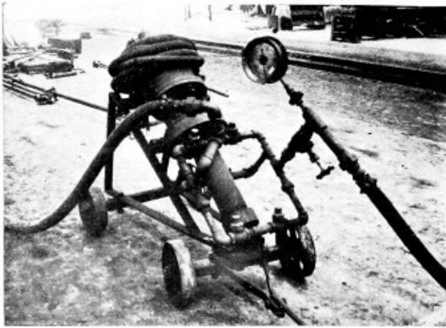
Portable Hydrostatic Pump for Boiler Testing
