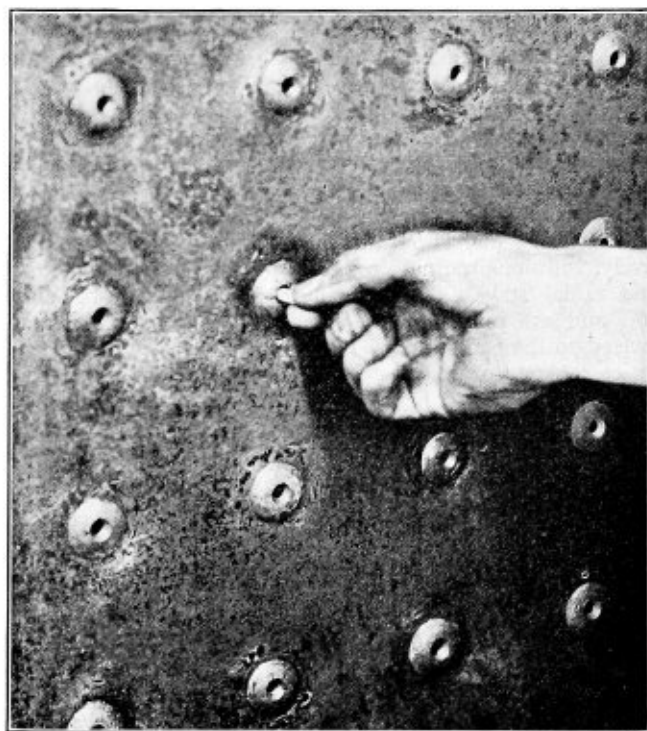
Fig. 4—Applying the porous closure to telltale hole after inspection
