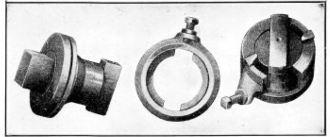
Construction and assembly of threadless washout plug
