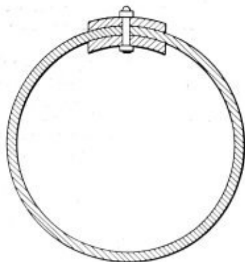
Fig. 3.—Clamp for maintaining alinement in welding longitudinal seams
