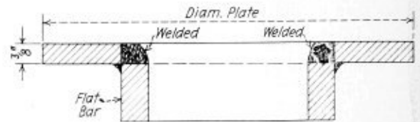
Fig. 1.—Detail of welded pipe flange
