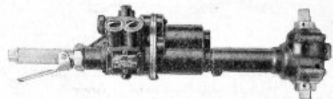
Thor type 71R pneumatic wrench
