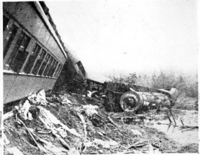
Figs. 1 and 2—This low water boiler explosion caused the death of four persons
