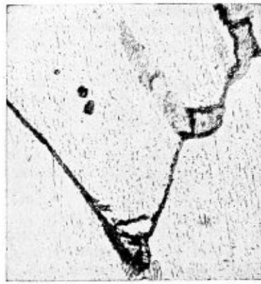
Fig. 11.—(a) and (b) Micrographs of flange steel embrittled in tests
