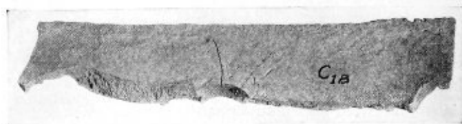
Fig. 5.—Section of cracked plate from boiler using treated water
