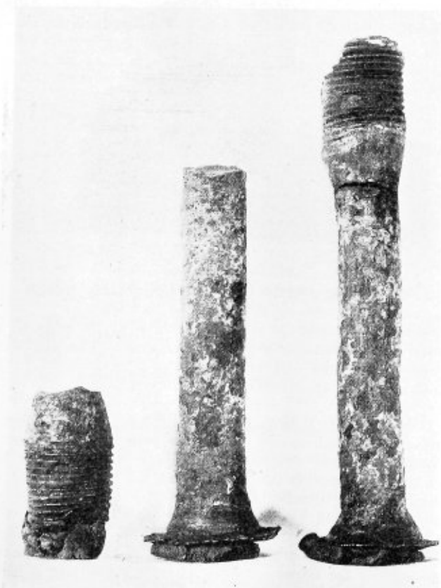
Fig. 12—Broken, reduced body staybolt
