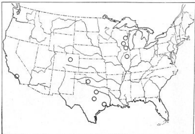
Fig. 4.—Areas in which boilers using well waters have been embrittled
