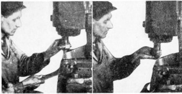
Fig. 18.—Correct way to adjust dies (left) and wrong method to use (right)
