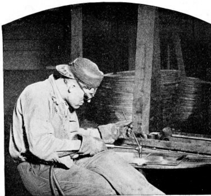
Fig. 3.—Making a practice weld
