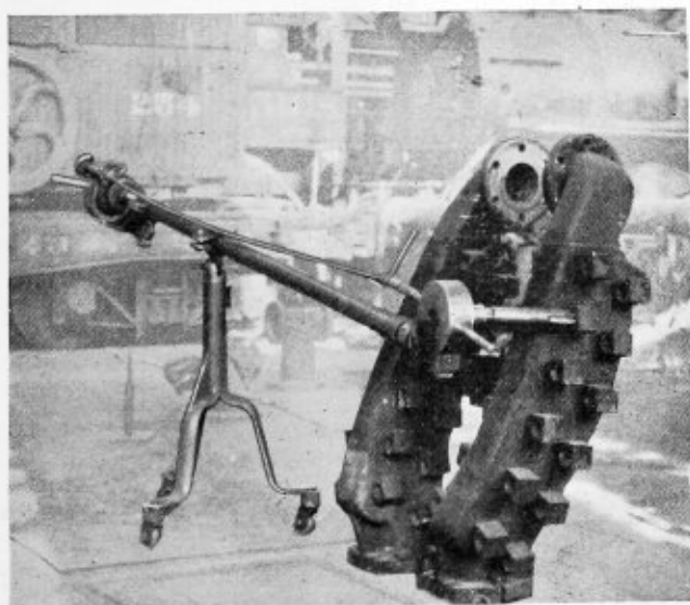
Machine in use for retapping superheater header block
