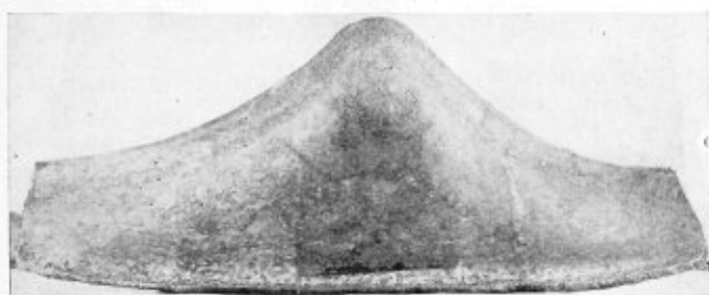
Fig. 1.—Section of flue ring, showing ruptured areas on the surface
