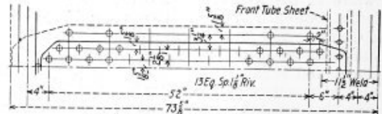
Fig. 6-Sextuple Riveted Longitudinal Seam Drawing
