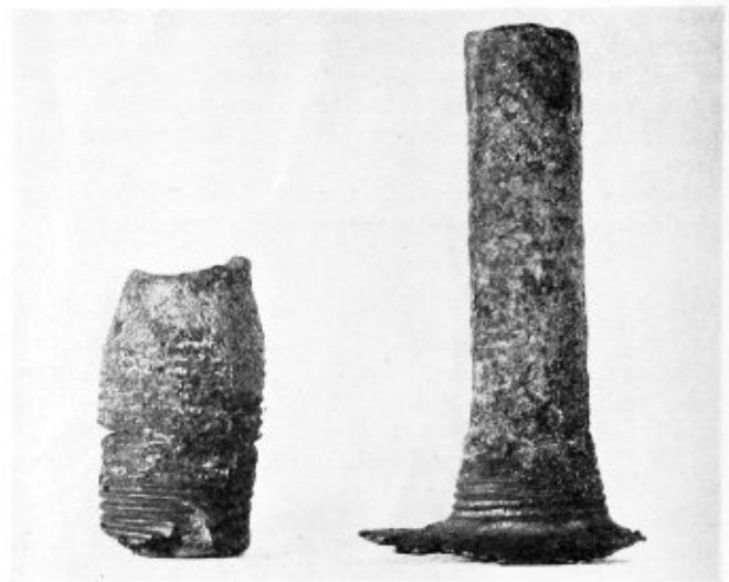
Fig. 6.—Broken, reduced body staybolt
