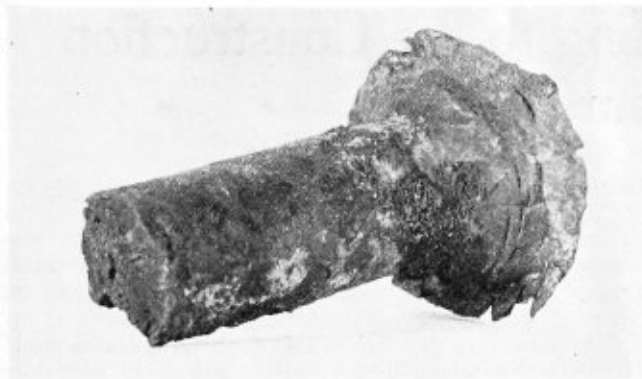
Fig. 8.—Part of broken staybolt which blew out of side sheet
