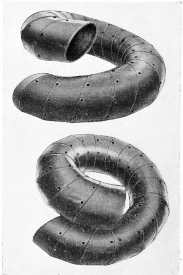
Two views of spiral pipe model developed by George House from a layout appearing in The Boiler Maker
