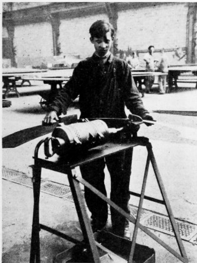
Cutting a template on a shop-made template-shearing machine
