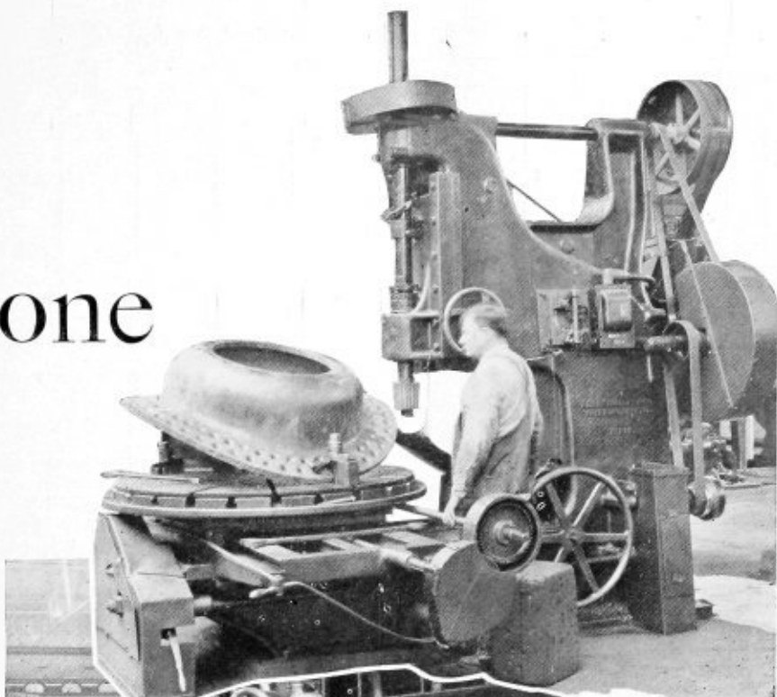
(Above)—Milling the flanges of a dome
