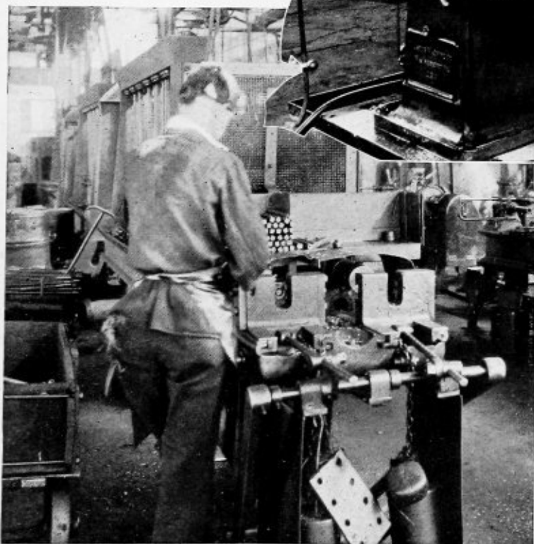
(Below)—Rounding the ends of waterspace staybolts
