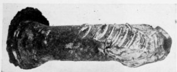
Fig. 4.—Another reduced-body staybolt removed from same firebox as the bolt shown in Fig. 3
