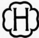
Fig. H-2A Official symbol for stamp to denote the American Society of Mechanical Engineers Standard
