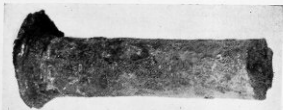
Fig. 3.—Part of a broken reduced-body staybolt that blew out of firebox sheet
