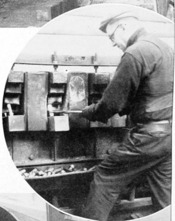
(Right) — Each bull riveter is equipped with a Berwick electric rivet heater
