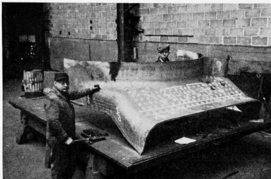
Laying out an outside throat sheet on the large surface block after flanging
