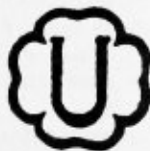
Fig. U-2A Official symbol for stamp to denote the American Society of Mechanical Engineers Standard
