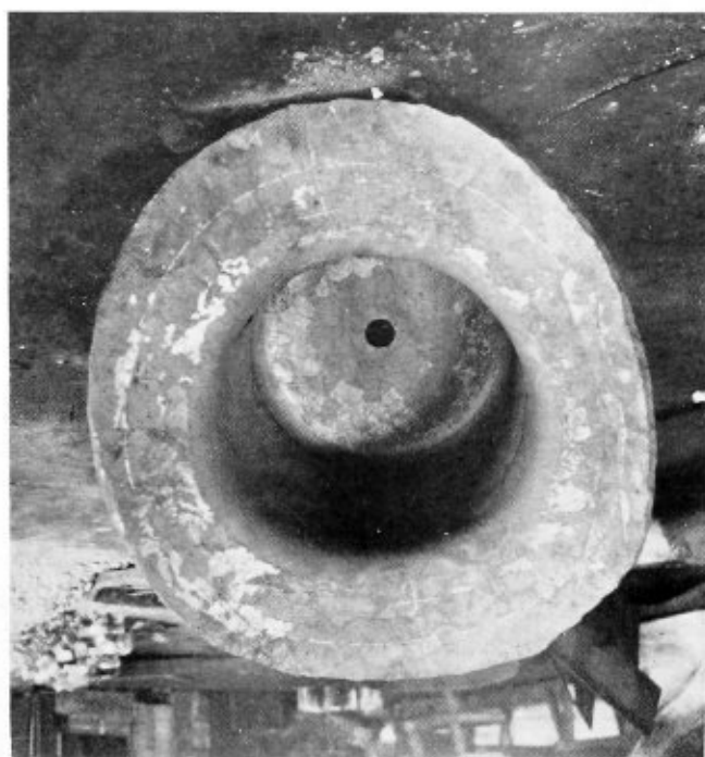
Fig. 55.—Looking into a dome flanged in one piece
