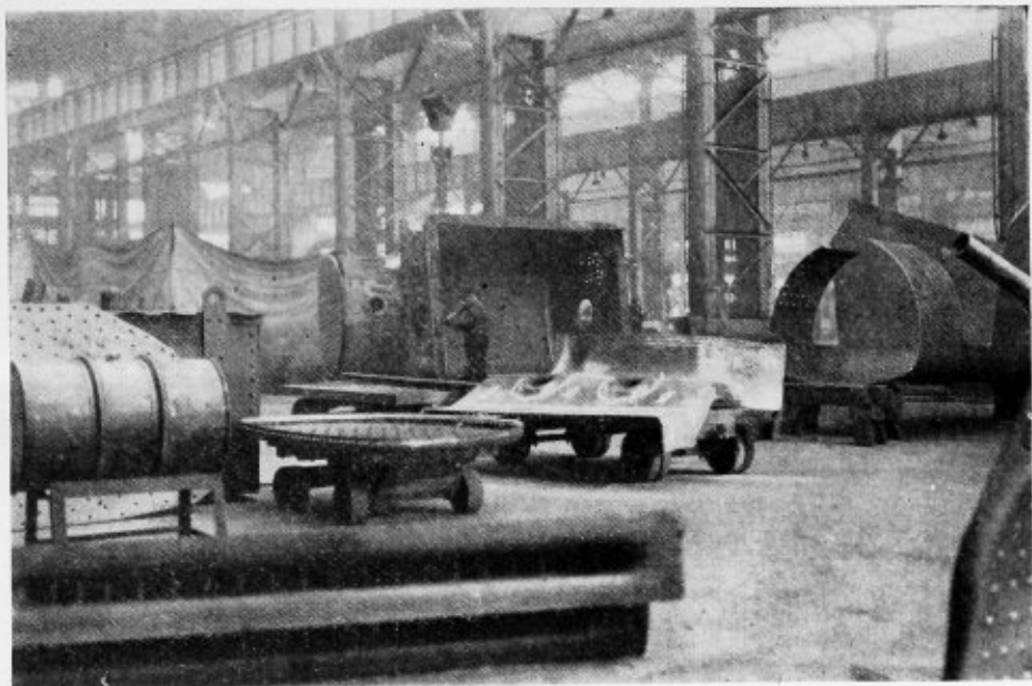
At work in the firebox assembly section
