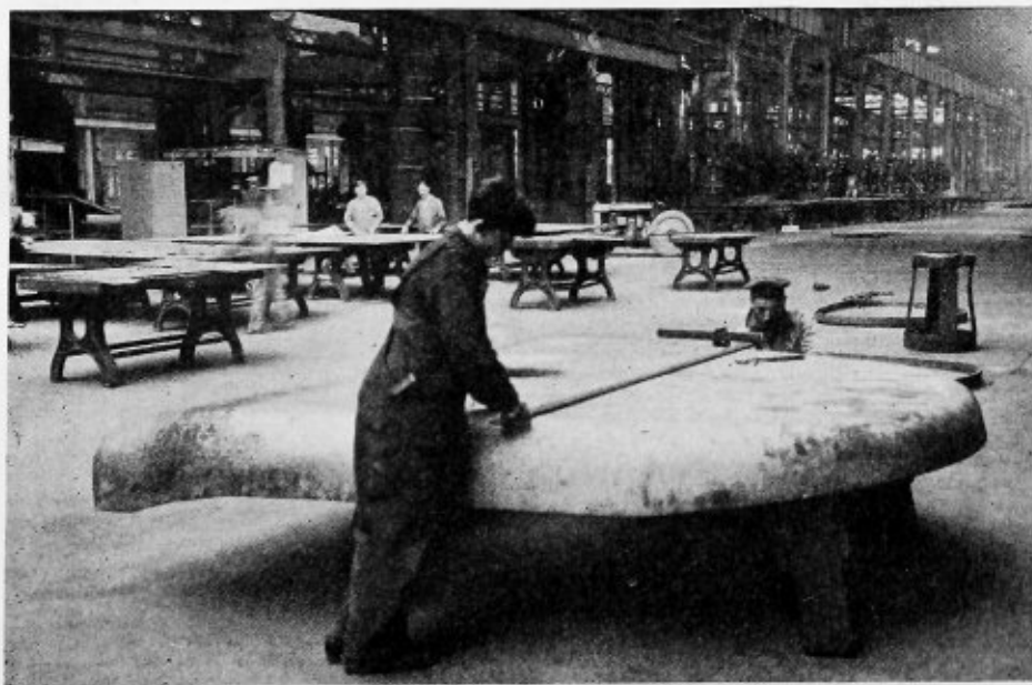
Leveling up a backhead after flanging
