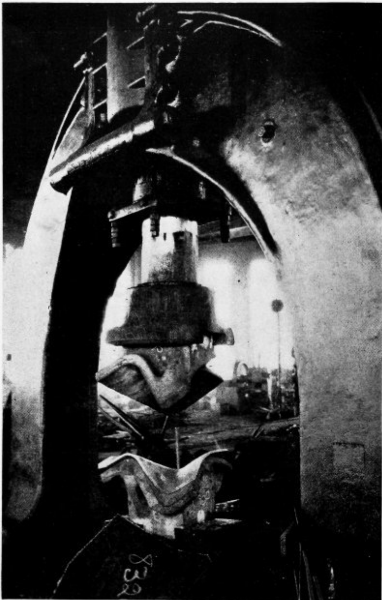
Forming a single patch under the steam hammer
