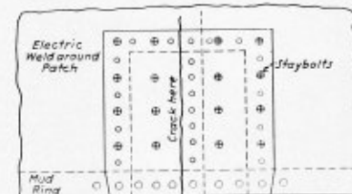
Fire crack repair
