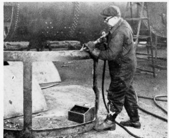
Clipping excess material from smokebox liners
