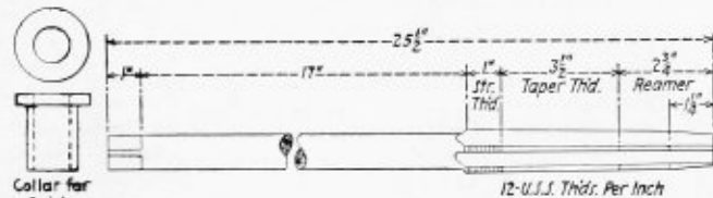
Fig. 4.—Flexible staybolt tap in common use
