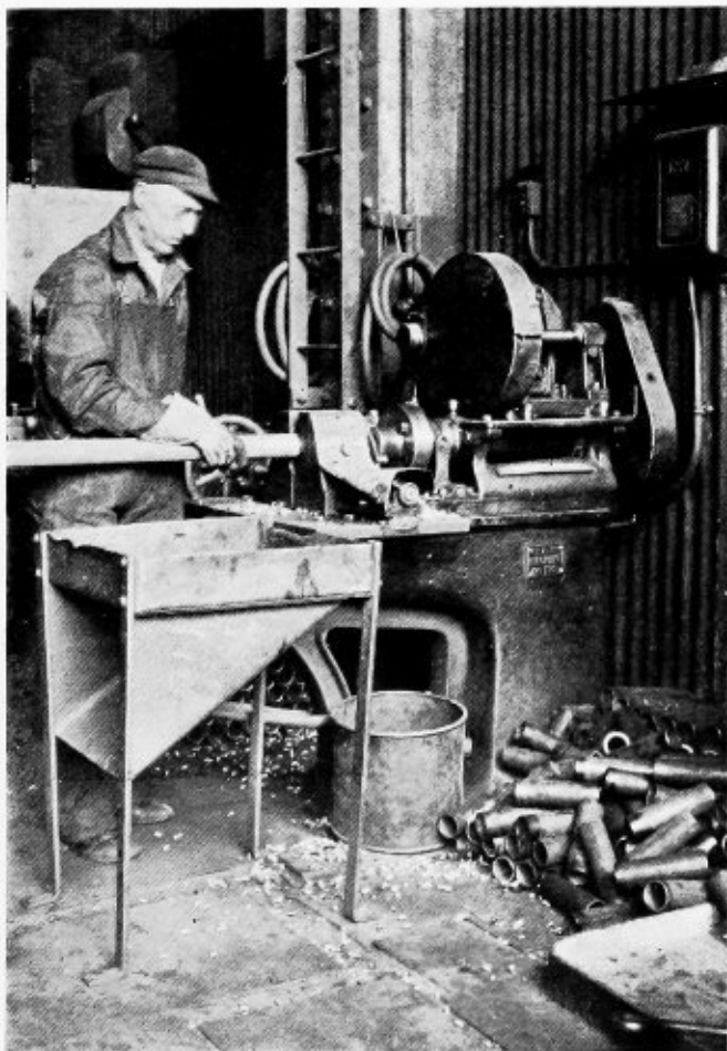
(Right)—Grinding the flue end prior to the safe-end welding operation. (Below)—Redesigned bolt cutter used for scarfing the flues for welding
