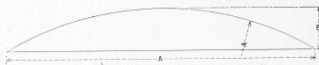
Formula: \frac{A^3}{102} \times C Cubic Capacity of Dished Ends in Cu. ft.
