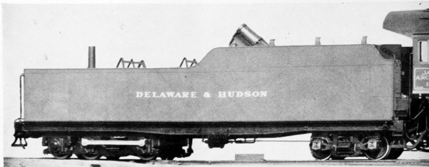
The locomotive James Archbald of the Delaware & Hudson Railroad, third of a design by John E. Muhlfeld, consulting engineer, with combined watertube and firetube boiler.
