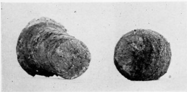
Fig. 9.—Ends of a broken reduced-body staybolt
