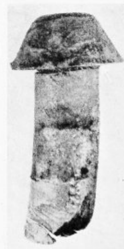
Rivet failed because of internal stress in shank
