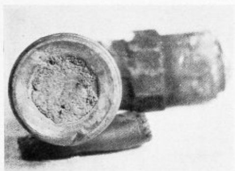
Fig. 5.—(At top). Transverse seam in door sheet which failed. Fig. 6.—(At right). Crown sheet failure resulting from low water. Fig. 7.—(Above). Water column connection which was plugged with scale
