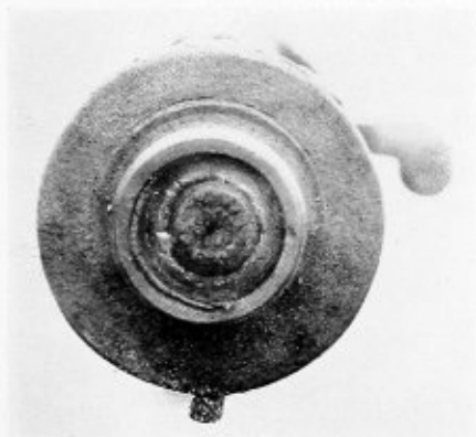
Fig. 2.—Water glass opening plugged by rubber gasket
