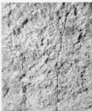
Fig. 1.—(Top) Pieces of shell plate from ruptured seam. Fig. 2.—(Bottom) Microphotograph showing rivet hole crack magnified eight times
