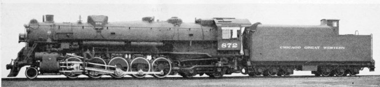
"Old Ironsides" weighed something less than 6 tons in working order—this locomotive weighs 232 tons in working order
