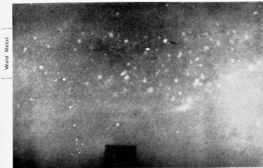
Radiograph Type 2.—Porous but acceptable
