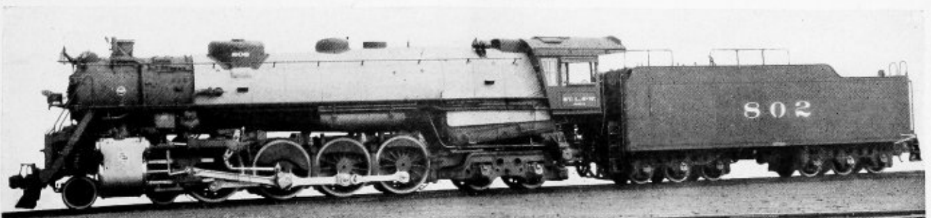
New Cotton Belt 4-8-4 locomotive built at The Baldwin Works
