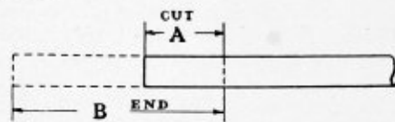
Fig. 6.—Method of piecing flues
