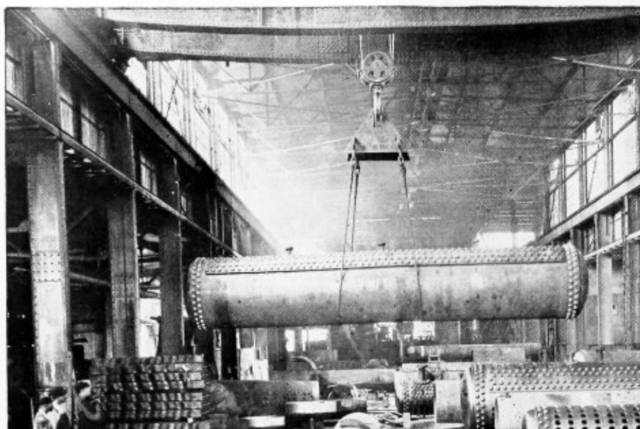
Boiler drum moved through shop by a large traveling crane. Note perfect balance of drum, also men standing clear of load
