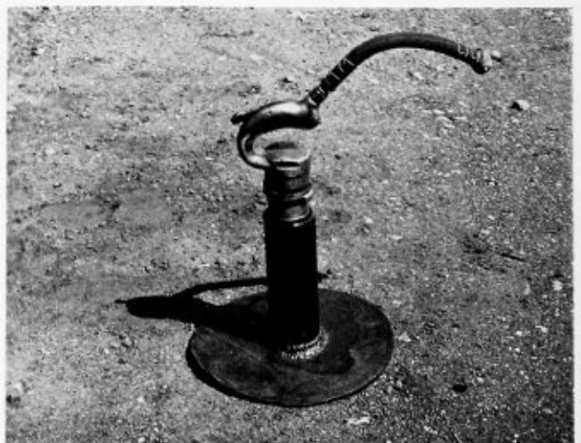
Rivet-hammer receptacle which contributes to convenience and safety
