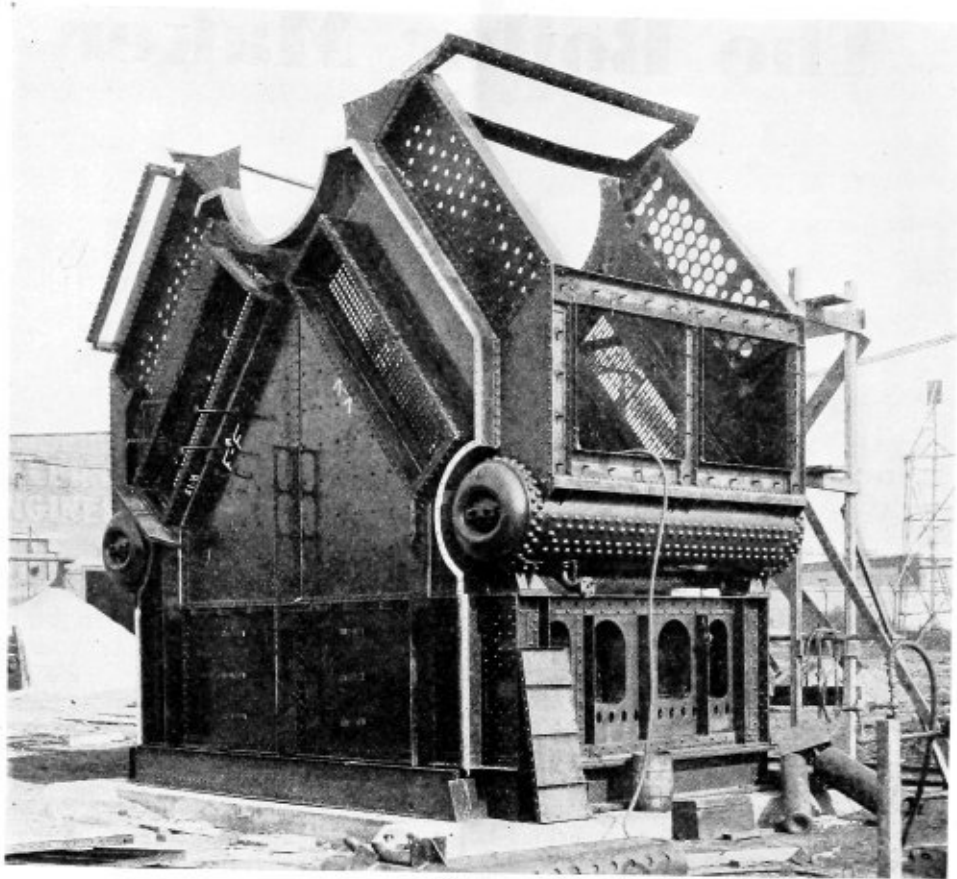
Fig. 1.—Casing assembly of new marine boiler
