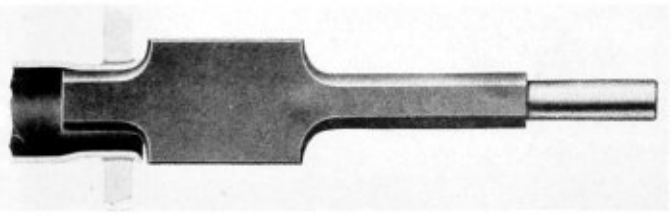
Fig. 6.—Standard flaring tool
