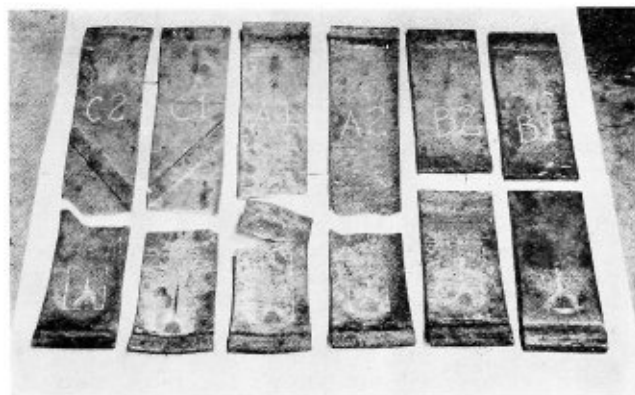
Fig. 5.—Welded lap joints after failure
