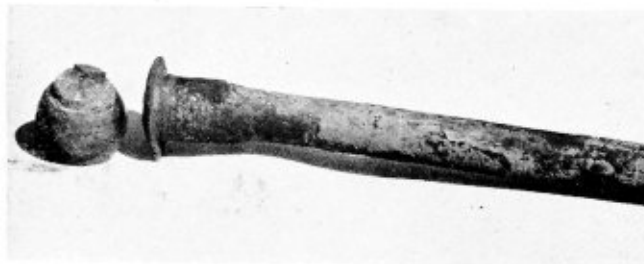
Fig. 6.—Broken flexible radial stay
