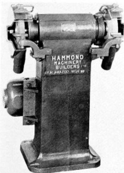
General purpose grinder using V-belt power transmission
