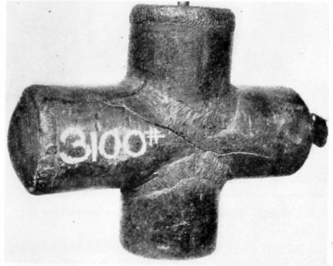
Fig. 3.—Crossed pipe sample failed at 3100 pounds
