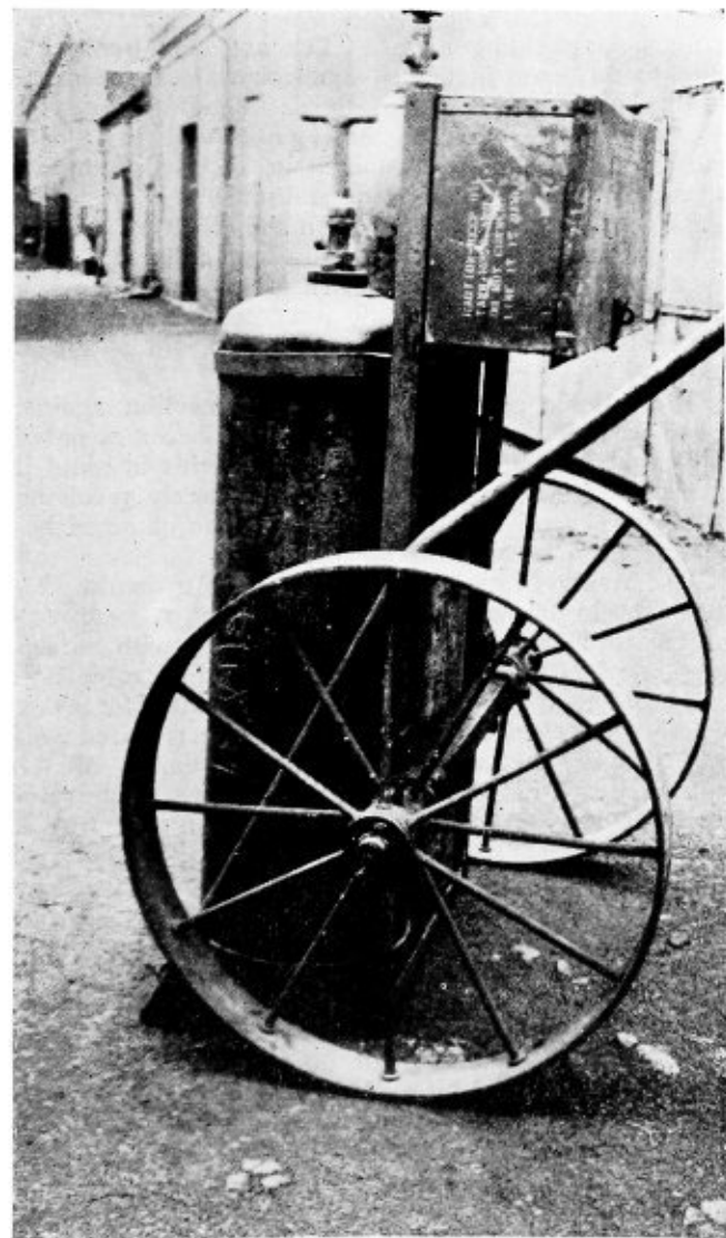
A portable truck for welding equipment that can be handled by one man
