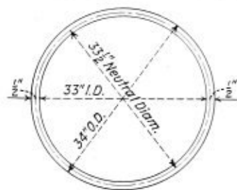
Section of tank showing dimensions
