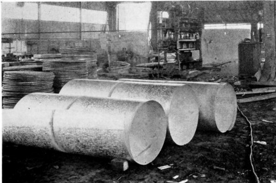
Fig. 1.—Lap-welded sheets after welding and rolling
