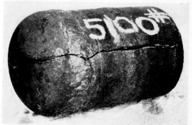
Fig. 4.—Pipe with welded heads failed at 5100 pounds
