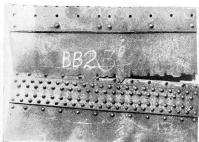
Fig. 5.—Specimen BB2 after failure
