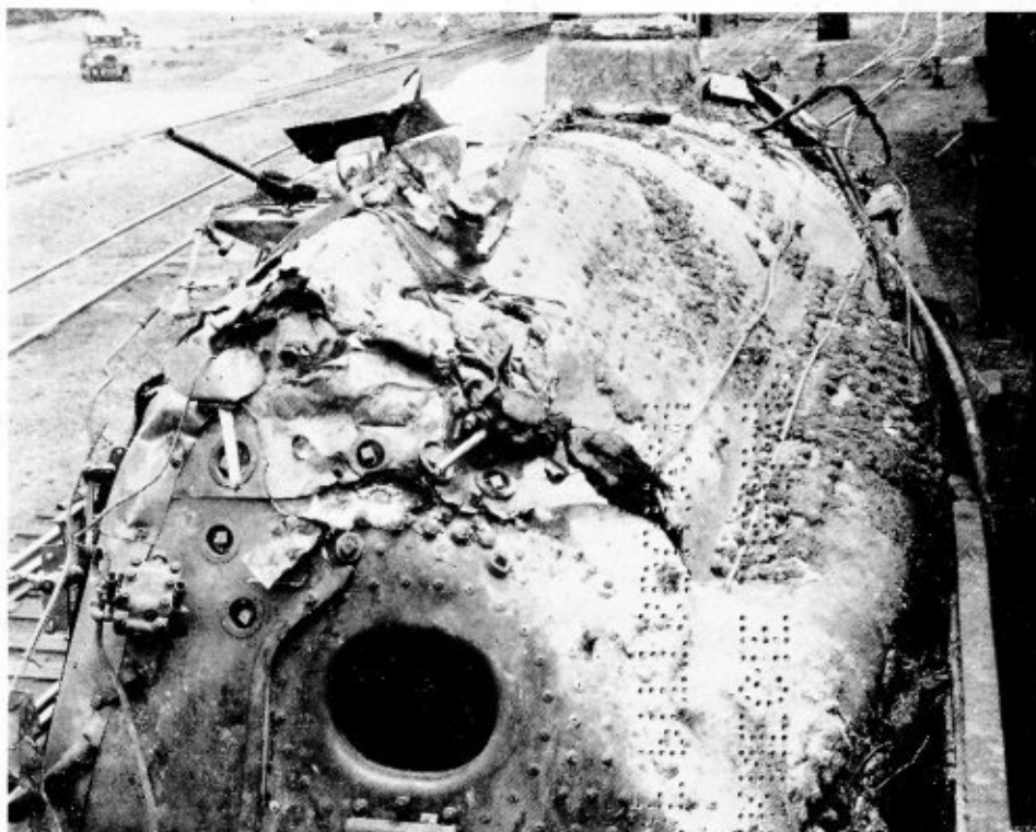
Fig. 1.—Result of crown sheet failure caused by low-water
