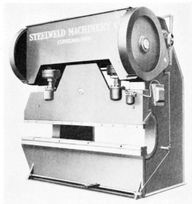
New bending brake with box-type welded housings
