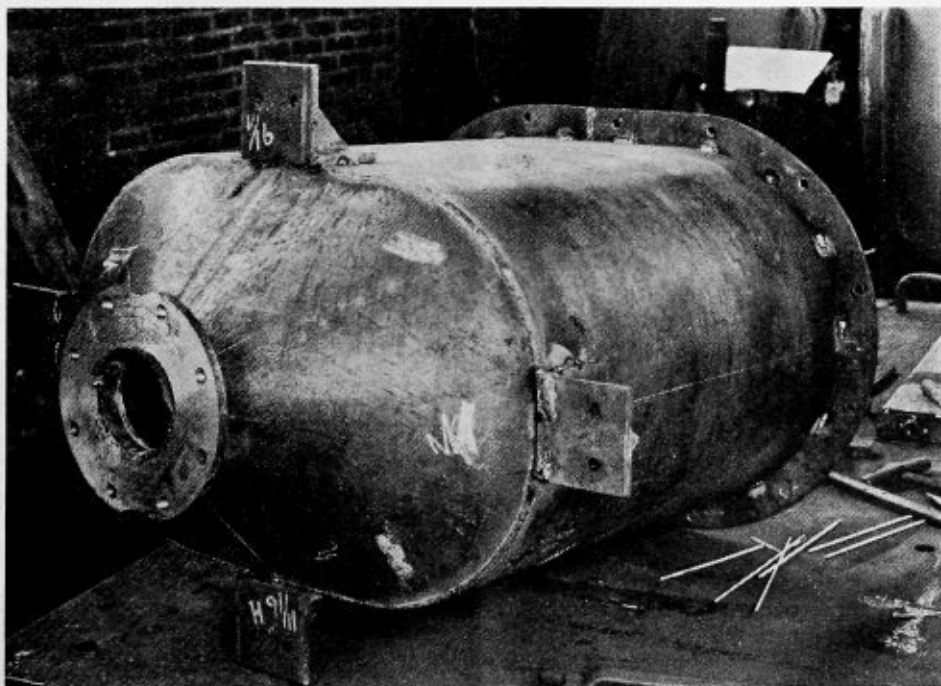
Fig. 3.—Elliptical nickel-clad steel pressure vessel
