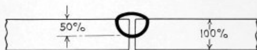
Fig. 1.—Plain butt weld where only 50 percent penetration is required. Most of the weld metal was supplied by the parent material
