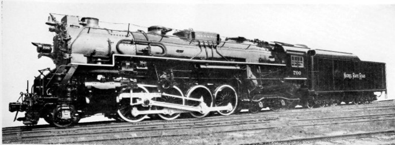
Nickel Plate 2-8-4 locomotive for freight service
