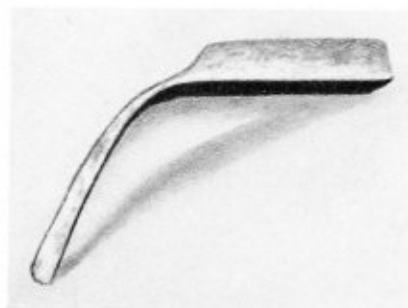
Fig. 1.—Effect of corrosion on mud drum head
