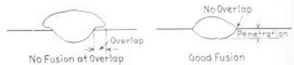
Fig. 2.—Correct bead should not overlap
