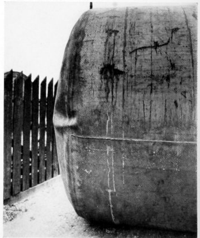
Tank that grew one foot in length under high pressure
