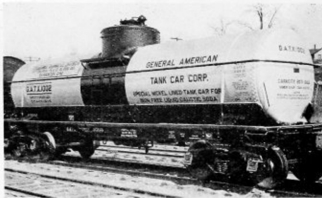
Fig. 5.—Tank car of 8000 gallons capacity
