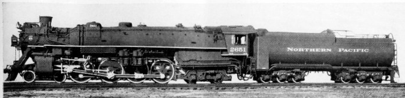
Northern Pacific 4-8-4 type, Class A-2, heavy passenger locomotive
