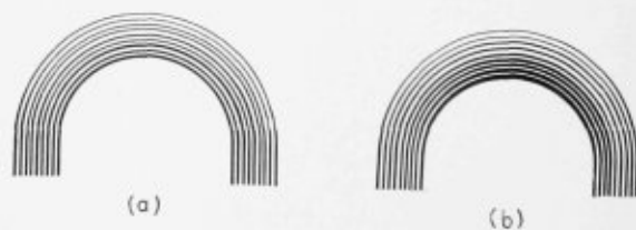
Fig. 3.—(a) Illustrating action of elastic parts each free to stretch individually—(b) If deck were gripped tightly at ends and then bent, outer cards would thin out and inner ones, instead of buckling, would compress and thicken
