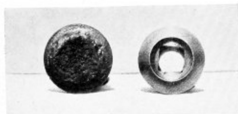
Fig. 6—Water column fitting plugged solid, compared with fitting in proper condition
