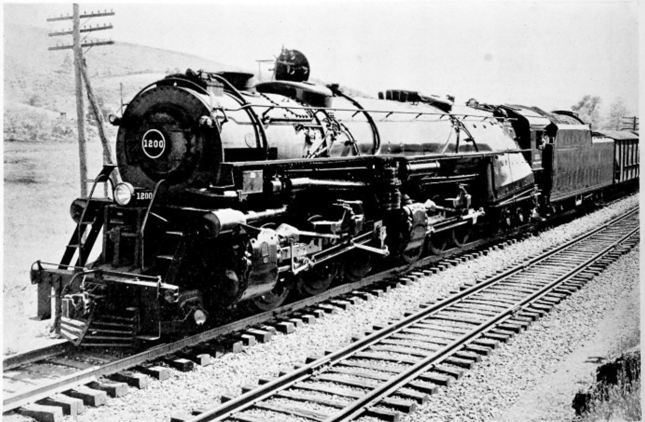
One of two new simple articulated Mallet locomotives built at the Roanoke shops of the Norfolk & Western
