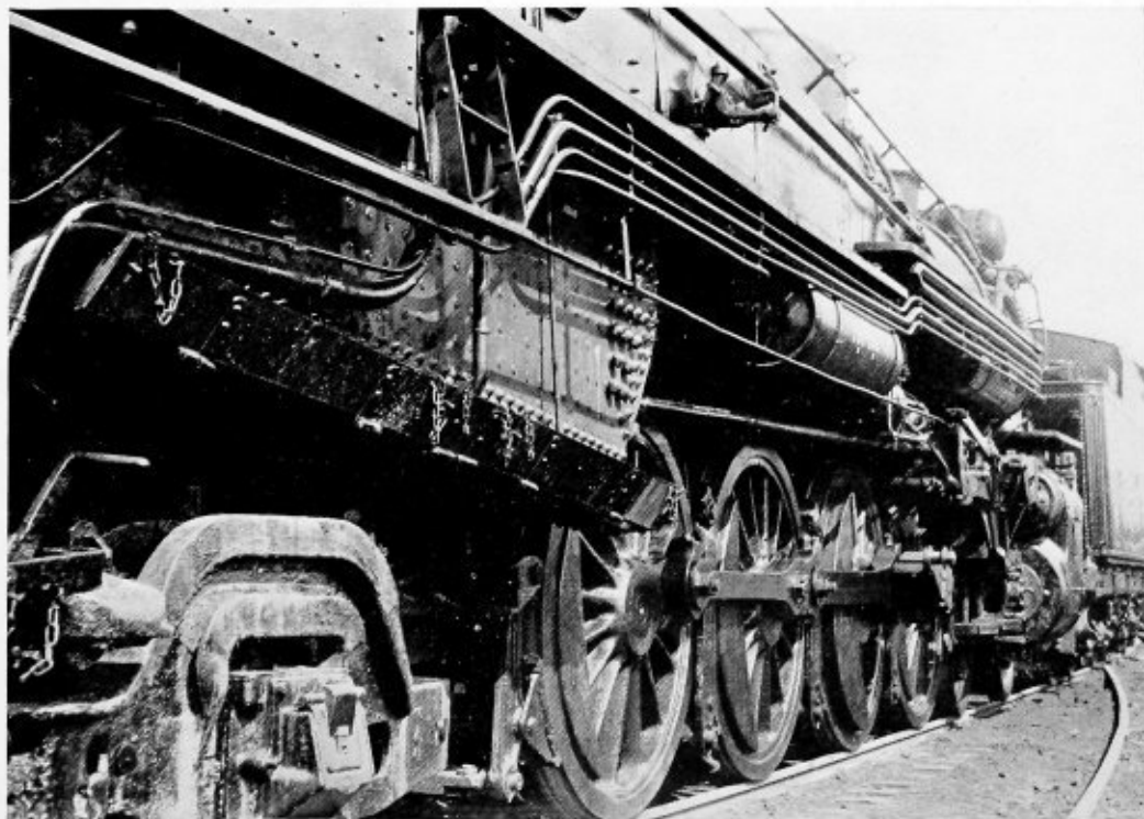
Oxy-acetylene welded piping on a locomotive
