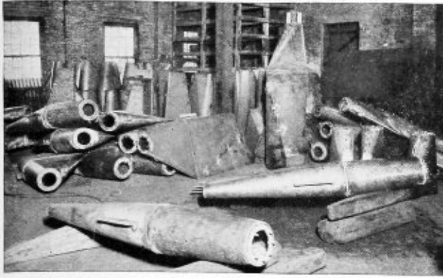
Buoys in process of fabrication
