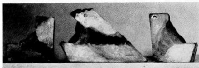
Good fusion in pipe joints
