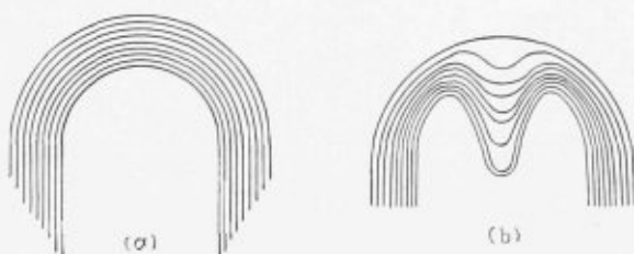
Fig. 2.—(a) This illustrates what would happen if all sections of a plate were free to move using a deck of cards to simulate the plate—(b) When the ends are gripped tightly the inside fibers must buckle when bent unless the outside fibers stretch
