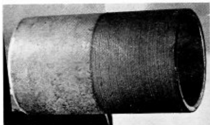
Fig. 1.—Section of standard locomotive flue—half bare and half surfaced with Apexior number 1
