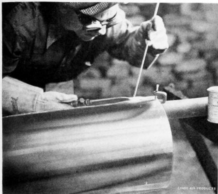
Welding a stainless steel container
