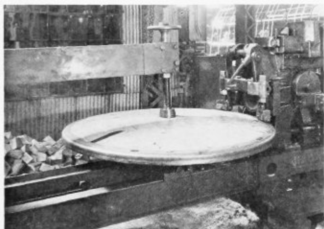
Fig. 16.—A spinning machine for cold flanging heads 28 inches in diameter and larger
