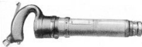
Fig. 1—Pneumatic hammer for driving staybolts
