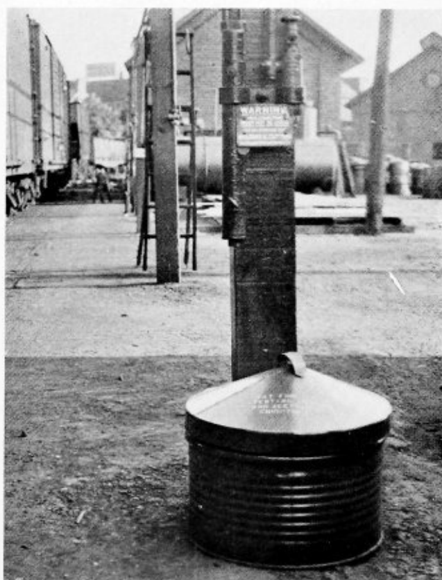
The practice of testing cutting torches and hose before use reduces accidents and saves gas
