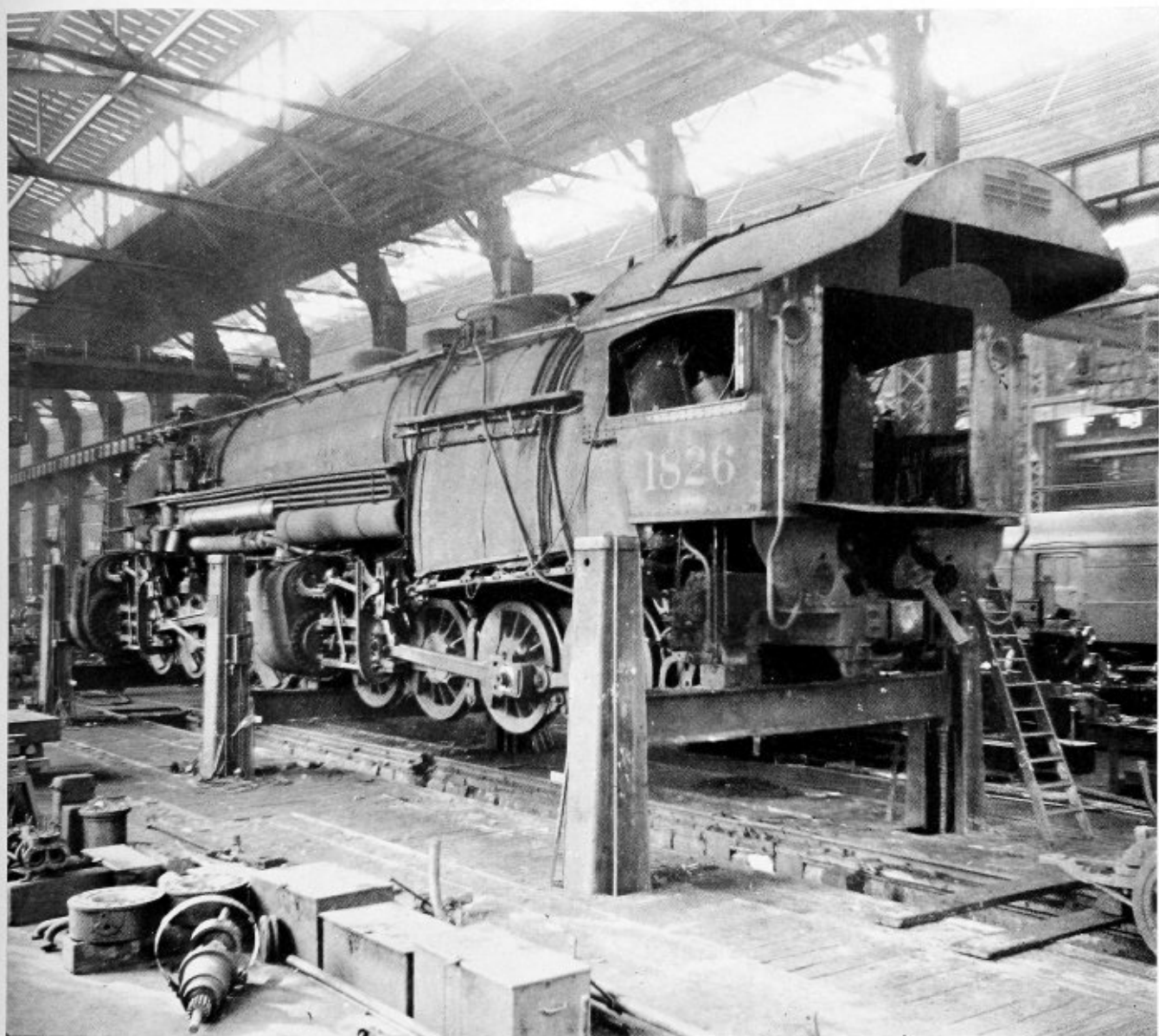
Mallet type locomotives are repaired at a special location equipped with a Whiting hoist
