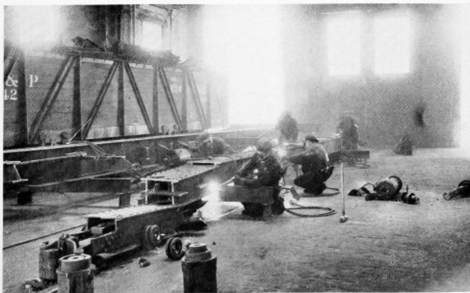
Cutting up underframes and center sills is an important part of the work in the North Shop
