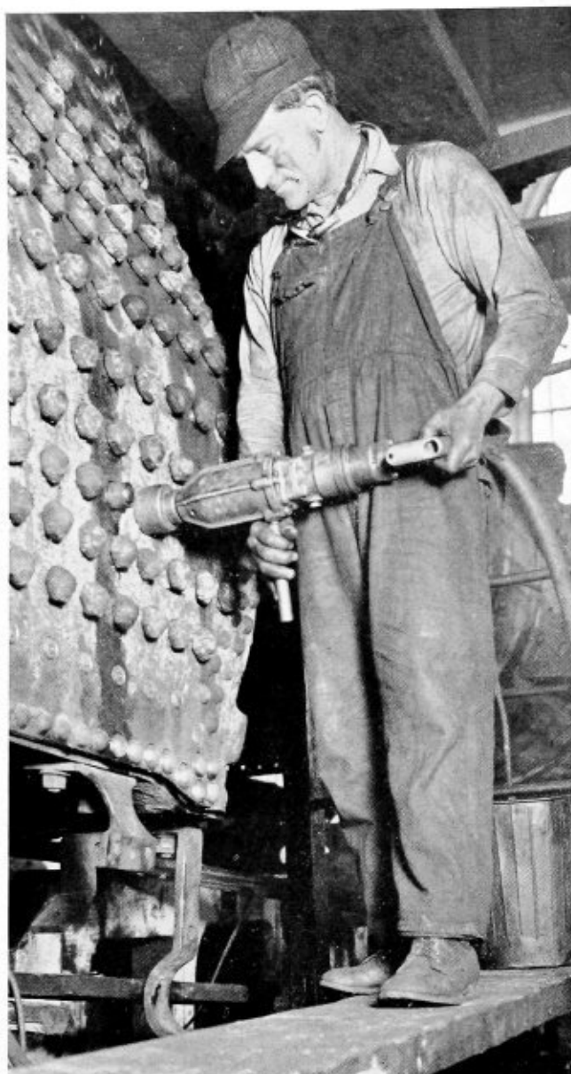
Using the impact wrench on staybolt caps
