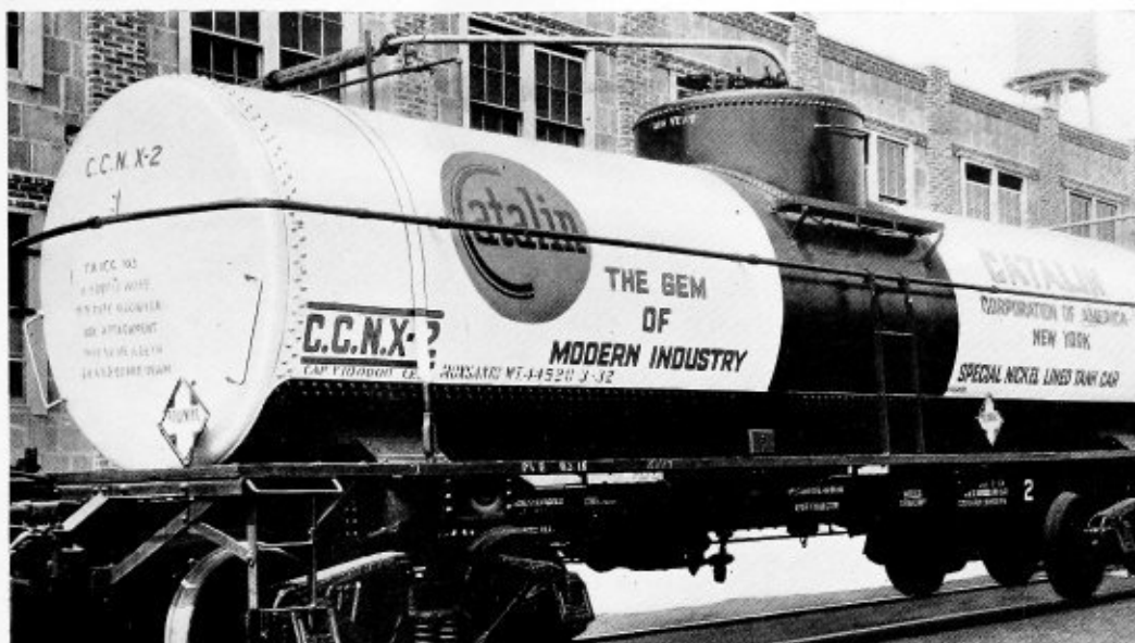
Fig. 5.—Nickel-clad steel tank car of 8000 gallons capacity used in transporting phenol for plastics
