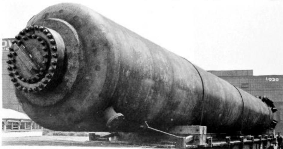
Water scrubber weighing 72 tons, 8 feet in diameter and over 72 feet long, fabricated by arc welding
