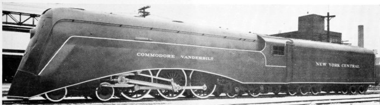
Fig. 1.—The steam locomotive offers opportunities for stream-lining
