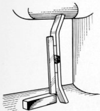
Fig. 1.—Start of the free bend test for ductility
