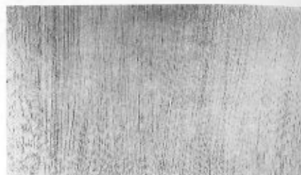
Fig. 2.—Apexior surfaced boiler plate, after two years service under 215 pounds steam pressure
