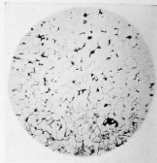
Fig. 4.—Normal grain structure of boiler plate before cutting
