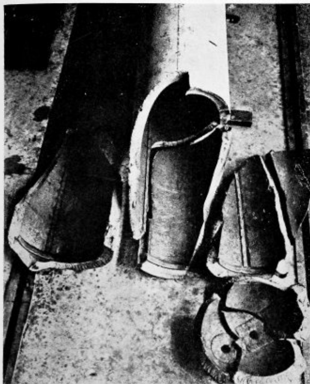
Fig. 1.—Failure of solid wall pressure vessel
