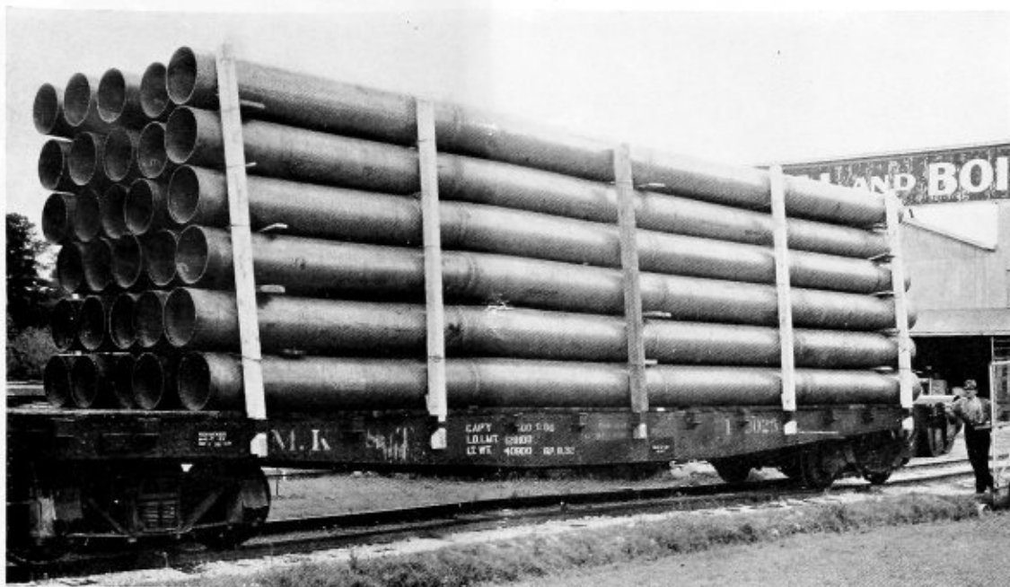
Fig. 1.—A carload of steel pipe manually fabricated by the shielded arc process of welding
