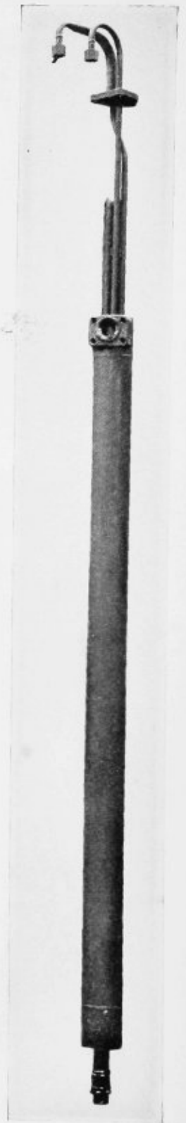
Fig. 4.—Superheater element partially withdrawn from evaporator tube
