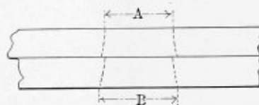
FIG. 9.—EFFECT OF PUNCHING HOLES IN LIGHT PLATE.
