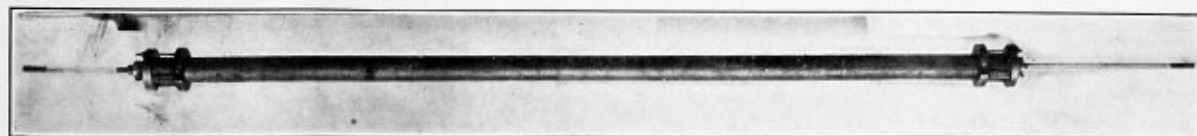
FIG. 5.—PHOTOGRAPH OF TUBE ABOUT TO BE TESTED, SHOWING MANNER OF CLOSING THE ENDS.
