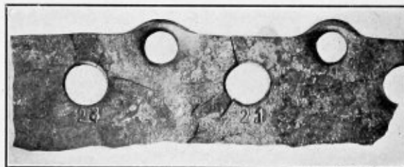
FIG. 6.—HOLES PUNCHED AT THE EDGE OF THE PLATE SHOWED THAT THE METAL HAD NOT BECOME BRITTLE.
