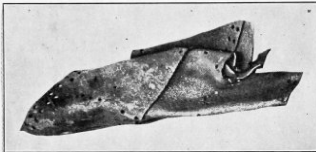
DAMAGED SHIP PLATE FROM S. S. "ROTTERDAM."
