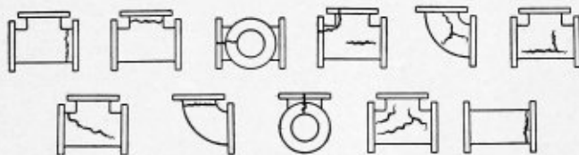
MANNER IN WHICH THE FITTINGS FAILED.
