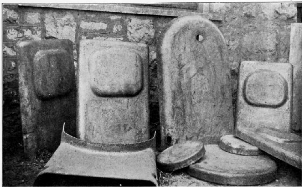
ILLUSTRATING THE VARIOUS SHEETS WHICH REQUIRE FLANGING IN A LOCOMOTIVE-TYPE BOILER.
