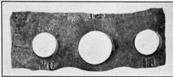
FIG. 5.—THE TAPERED PIN-TEST PRODUCED NO CRACKS, ALTHOUGH THE HOLE WAS ENLARGED 36 PERCENT.
