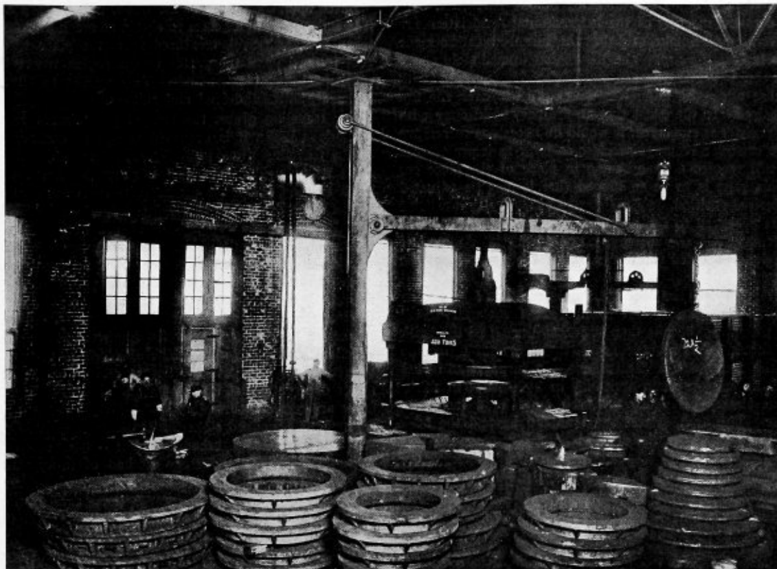
FIG. 52.—FOUR-COLUMN PRESS INSTALLED IN A BOILER SHOP FOR FLANGING ROUND PLATES.
