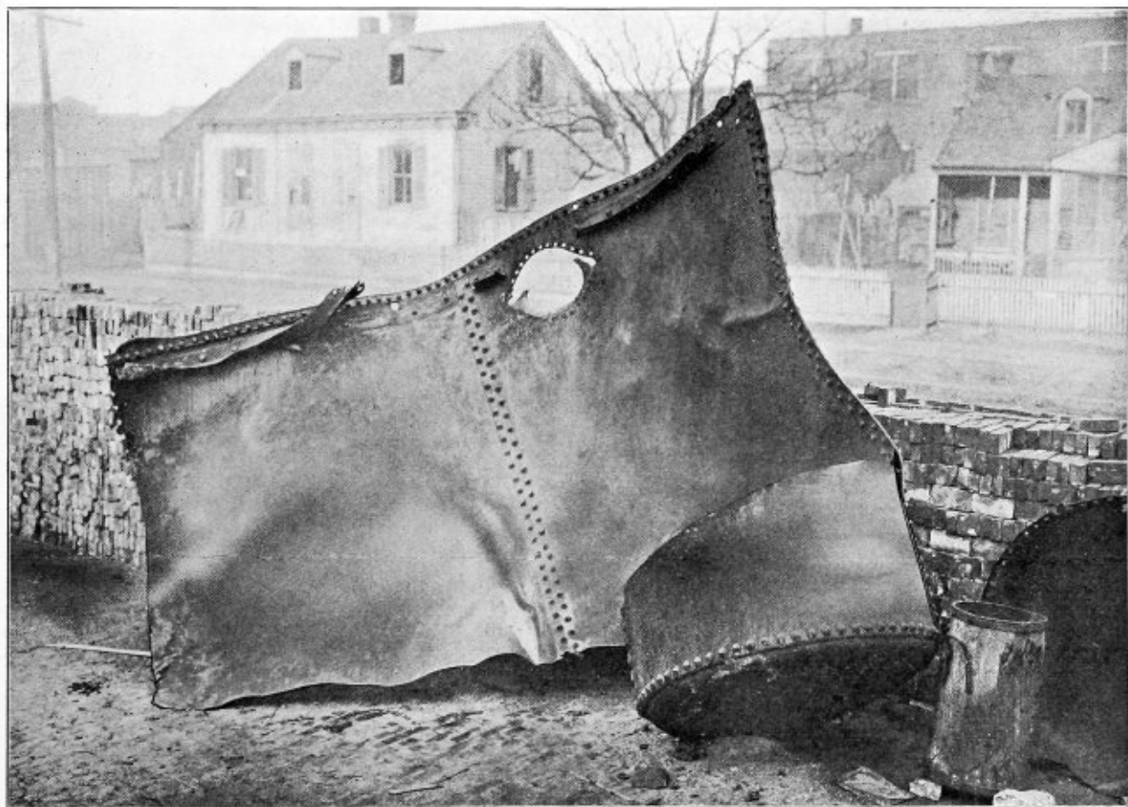
FIG. 1.—PORTION OF EXPLODED TANK, SHOWING NATURE OF THE RUPTURE.
