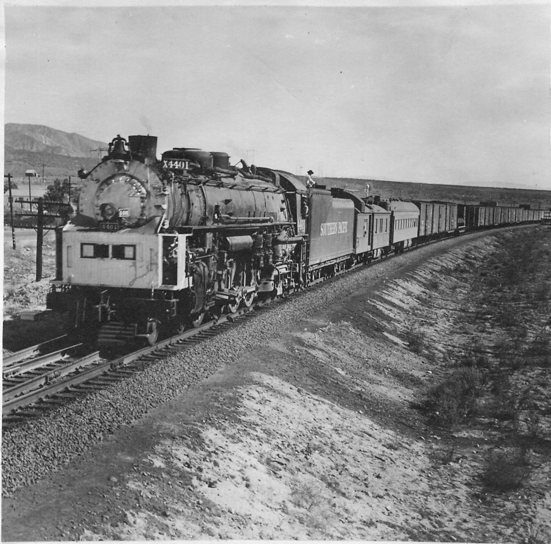
Test locomotive SP-4401 followed by Dynamometer Car SP-137 and Auxiliary Test Car SP-2300 handling maximum tonnage test train at full throttle upgrade near Cabazon, California.
