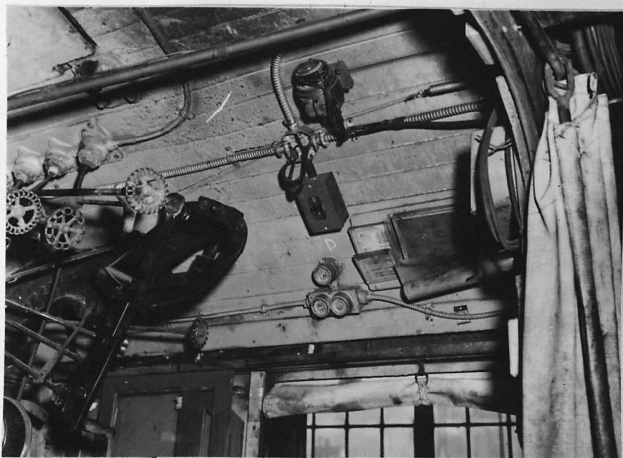
Throttle position selsyn transmitter application to roof of cab and throttle lever.
