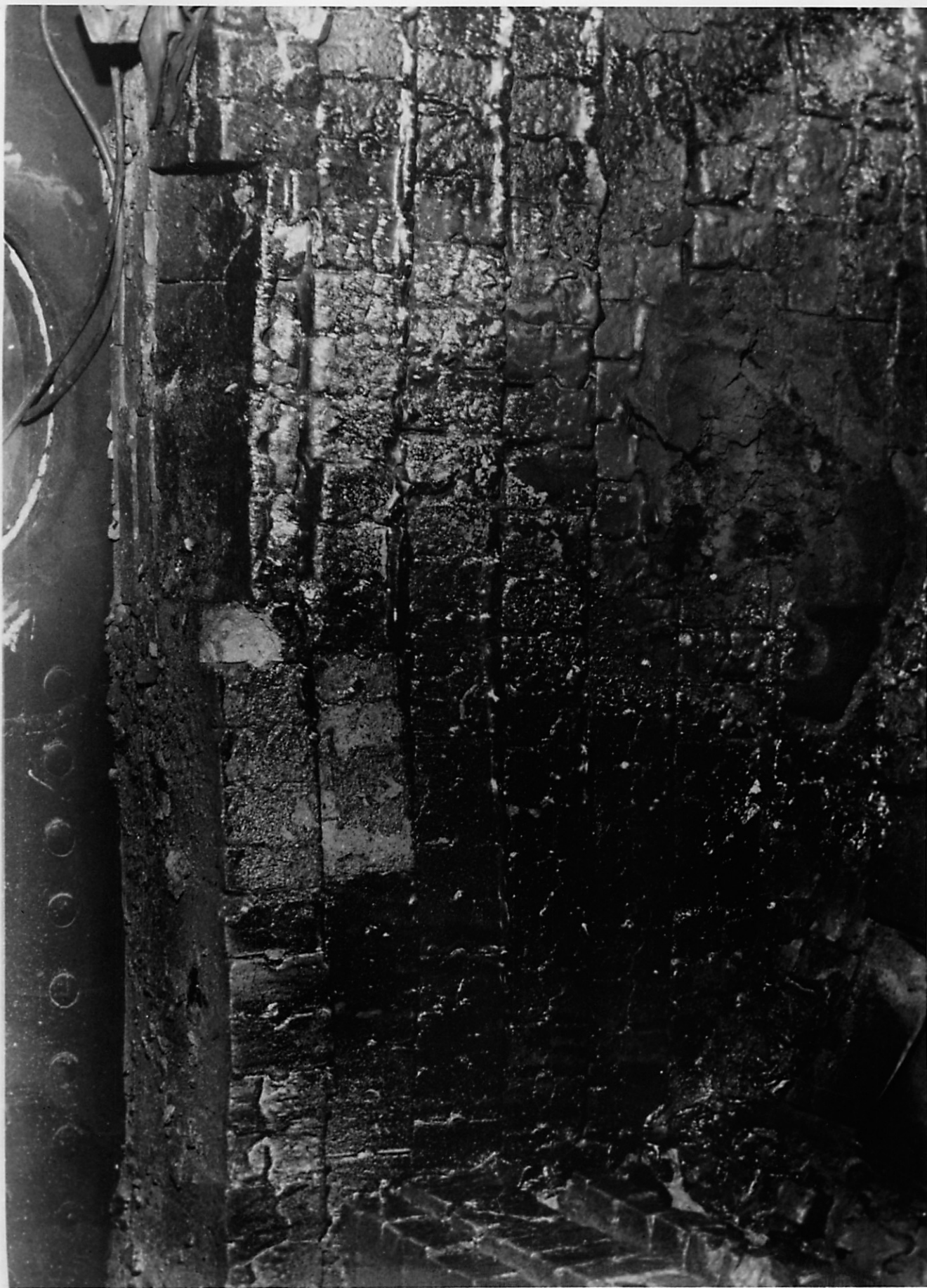
Appearance of buckled brickwork in flash wall - Test Locomotive SP 4401.
