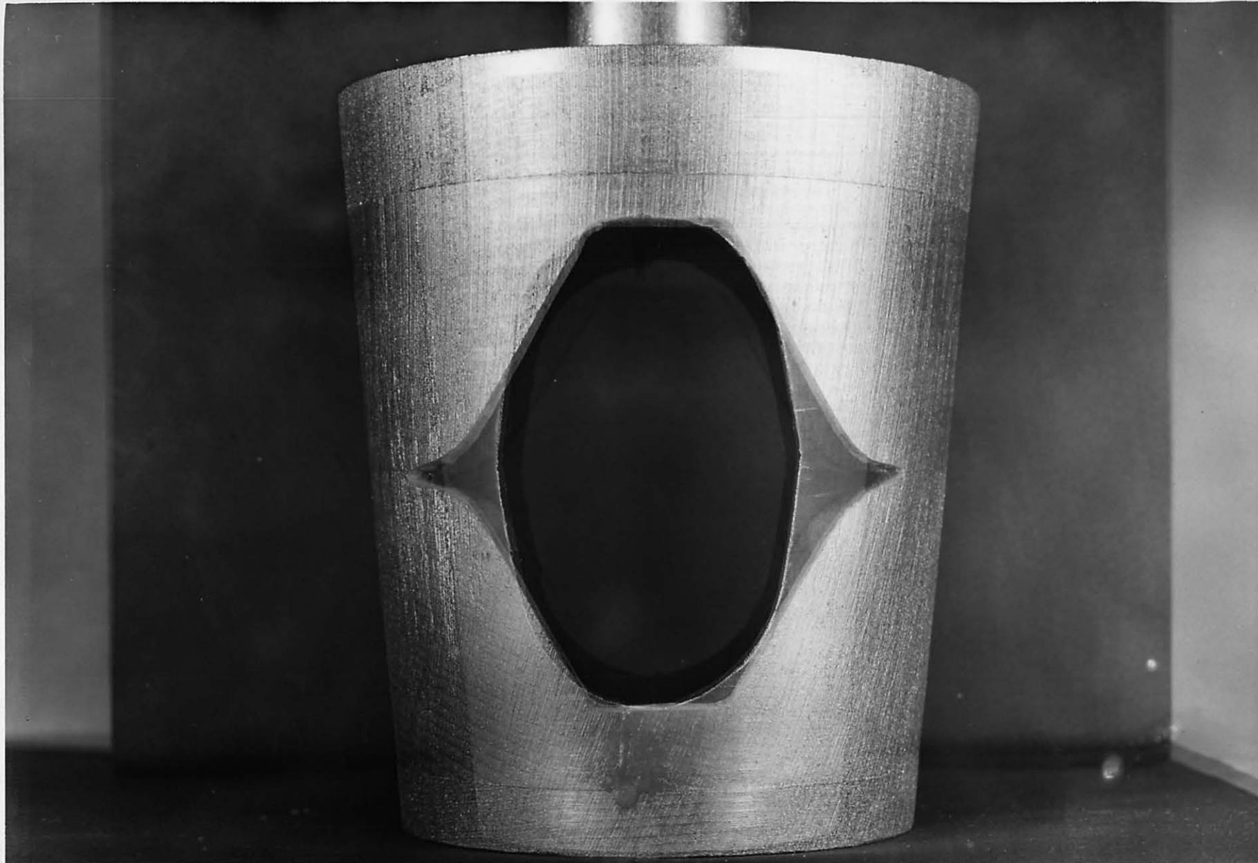
Double taper and common standard plug valves - Study of comparative contours superimposed by double exposure.
